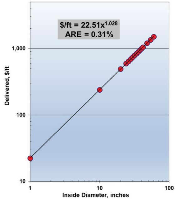
Fig. 3. Seamless API 5L x60 PSL2, ½” wall thickness.
