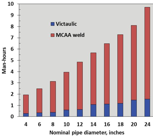
Fig. 5. Victaulic vs. weld installation time, man-hours/joint.
