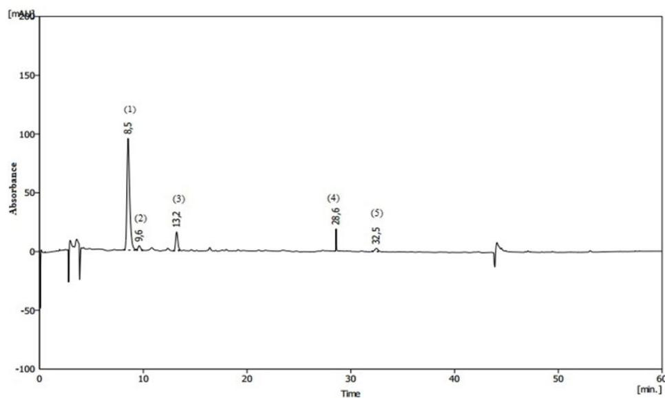
Fig. 5. HPLC chromatogram of the phenolic extract: (1) hydroxytyrosol, (2) tyrosol, (3) caffeic acid, (4) *p*-coumaric acid, and (5) oleuropein.
