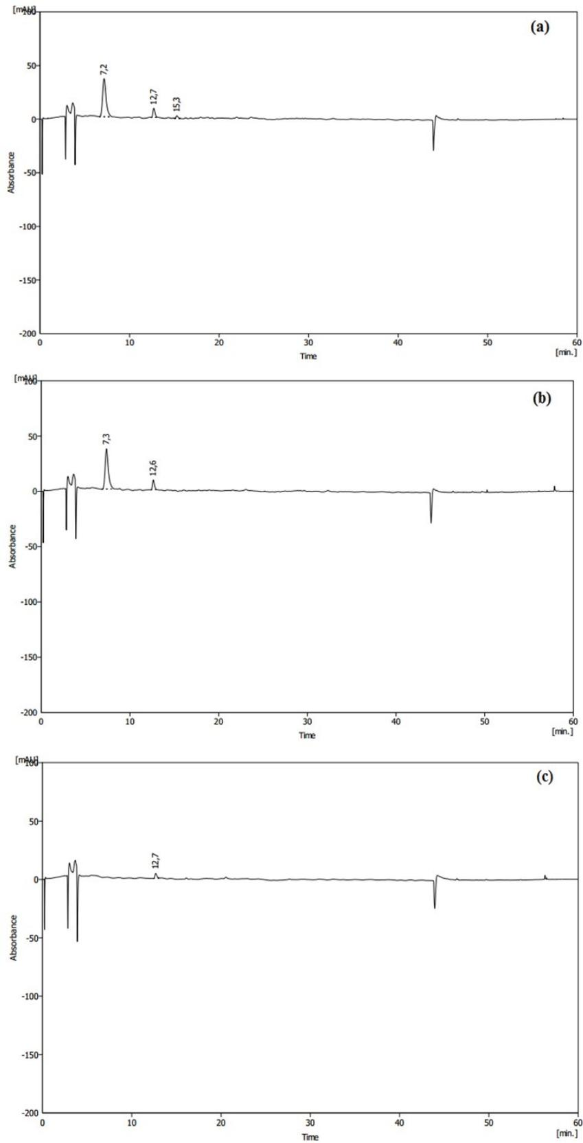
Fig. 6. HPLC chromatogram of phenolic compounds extracted from olive mill wastewater after treatment, (a) shaking (150 rpm), (b) incubation temperatures (37°C), and (c) nitrogen sources (urea).
