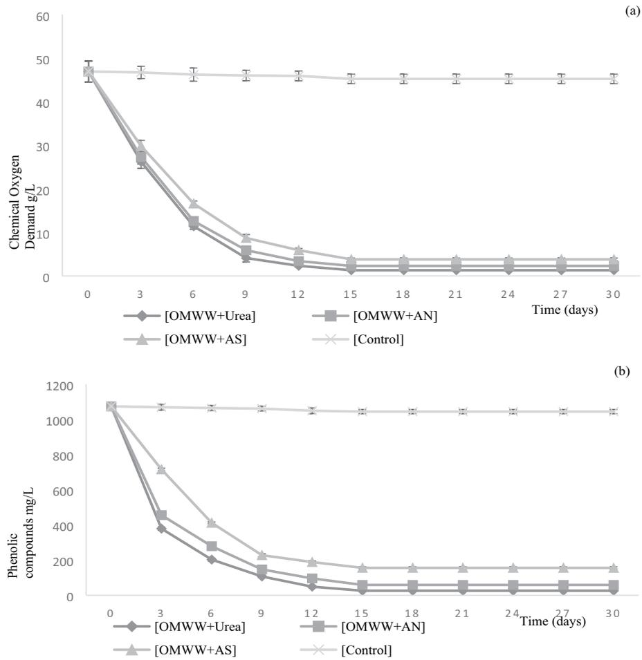
Fig. 4. Effect of different nitrogen sources on the olive mill wastewater chemical oxygen demand removal (a) and phenolic compounds biodegradation (b) by *Bacillus subtilis*. (Urea; AS: ammonium sulfate; AN: ammonium nitrate)
