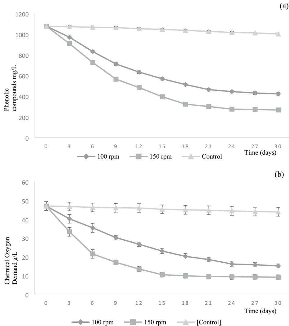
Fig. 2. Effect of different shaking rates on the olive mill wastewater phenolic compounds biodegradation (a) and chemical oxygen demand removal (b) by *B. subtilis*.
