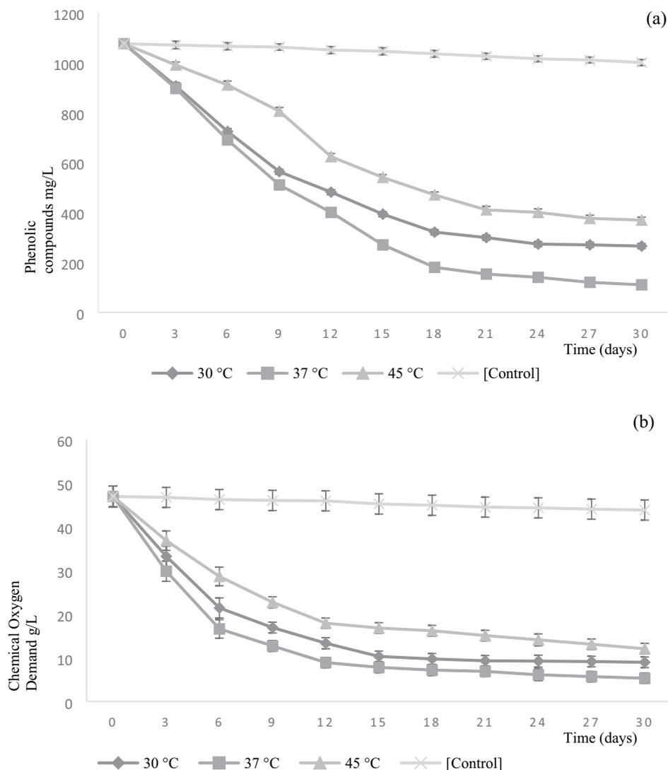
Fig. 3. Effect of different incubation temperatures on the olive mill wastewater phenolic compounds biodegradation (a) and chemical oxygen demand removal (b) by *Bacillus subtilis*.
