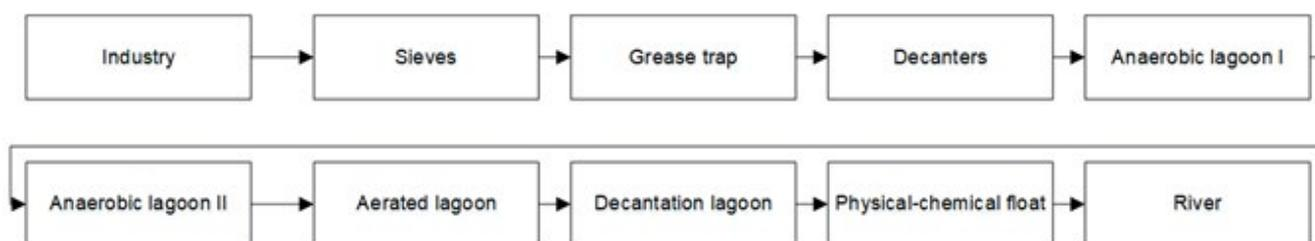
Fig. 1. Effluent treatment adopted by the industry.
