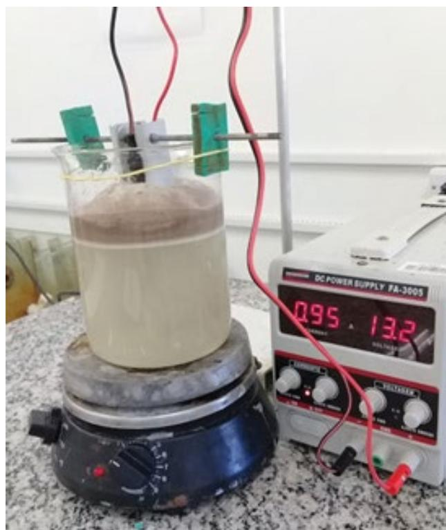
Fig. 2. Batch electrocoagulation system.
