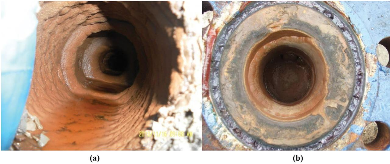
Fig. 1. Scaling phenomena of station A (a) pipeline and (b) valve in the gas field.
