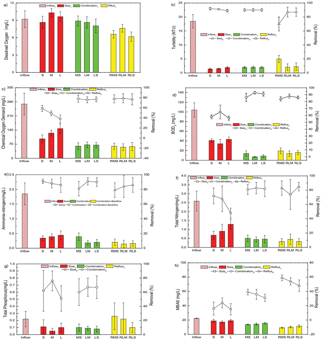
Fig. 2. Comparison between inflow and outflow synthetic graywater treated in a variety of experimental setup designs of quartz sand filters in terms of the following parameters: (a) DO, (b) turbidity, (c) COD, (d) BOD<sub>5</sub>, (e) NH<sub>4</sub><sup>+</sup>-N, (f) TN, (g) TP, and (h) MBAS. X-axis: the number of tested samples was, respectively, 9, 10, and 7 for the three stages. Y-axis: the subscripts V and R refer to the value and removal rate of the water quality index.
