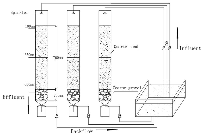
Fig. 1. Setup of quartz sand filter.
