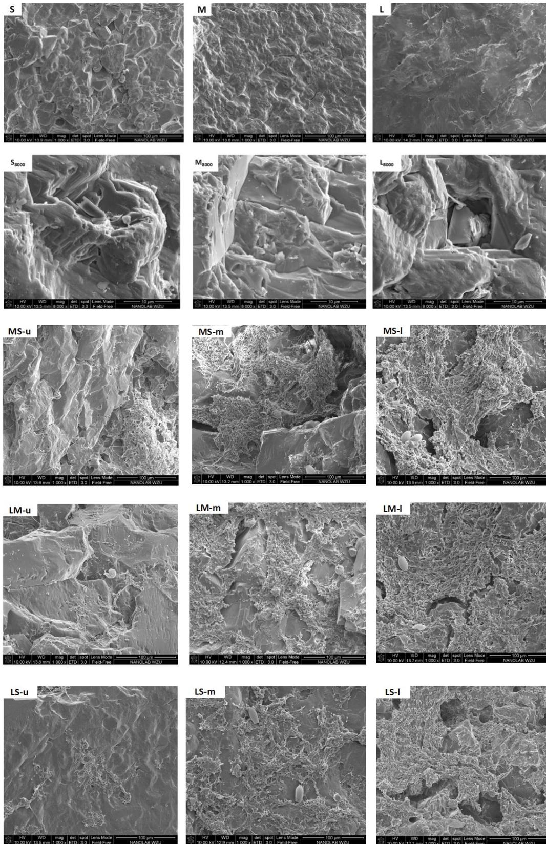
Fig. 3. SEM images of quartz sand. The subscript *u*, *m*, and *l* refer to the upper, middle, and lower quartz sand of the column filter for the second stage, respectively.
