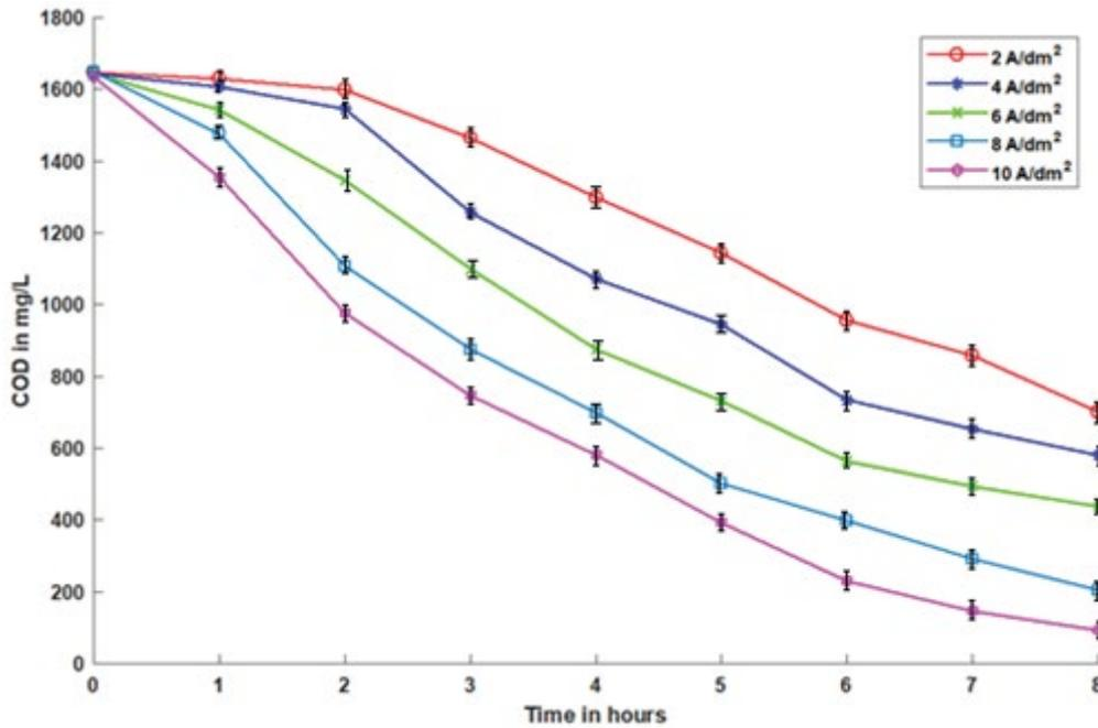
Fig. 4. COD reductions with respect to time for different current densities at 20 L/h.
