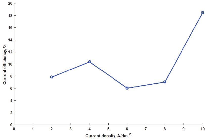
Fig. 6. Current efficiency vs. current densities at 20 L/h.
