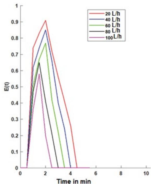
Fig. 2. Exit age distribution  $E(t)$  curve for different flow rates
