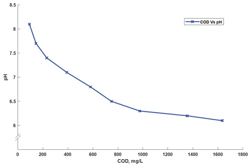
Fig. 7. Variation of pH vs. COD for the flow rate 20 L/h at 10 A/dm<sup>2</sup>
