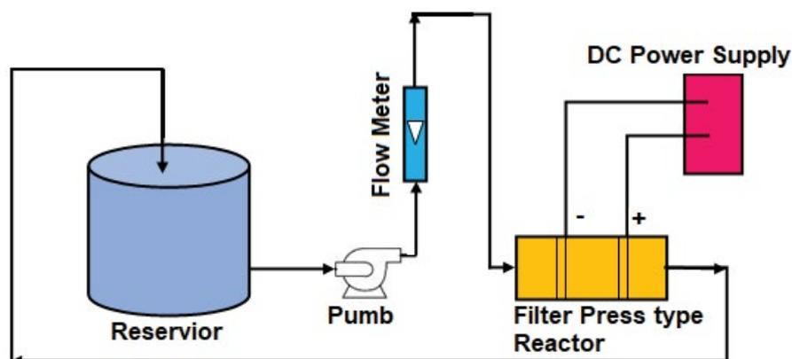
Fig. 1. Schematic representation of filter press type electrochemical reactor (FPECR) set up.
