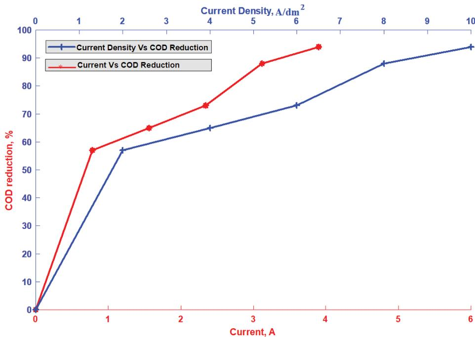
Fig. 5. Percentage reduction of COD vs. current density and current for the flow rate of 20 L/h.
