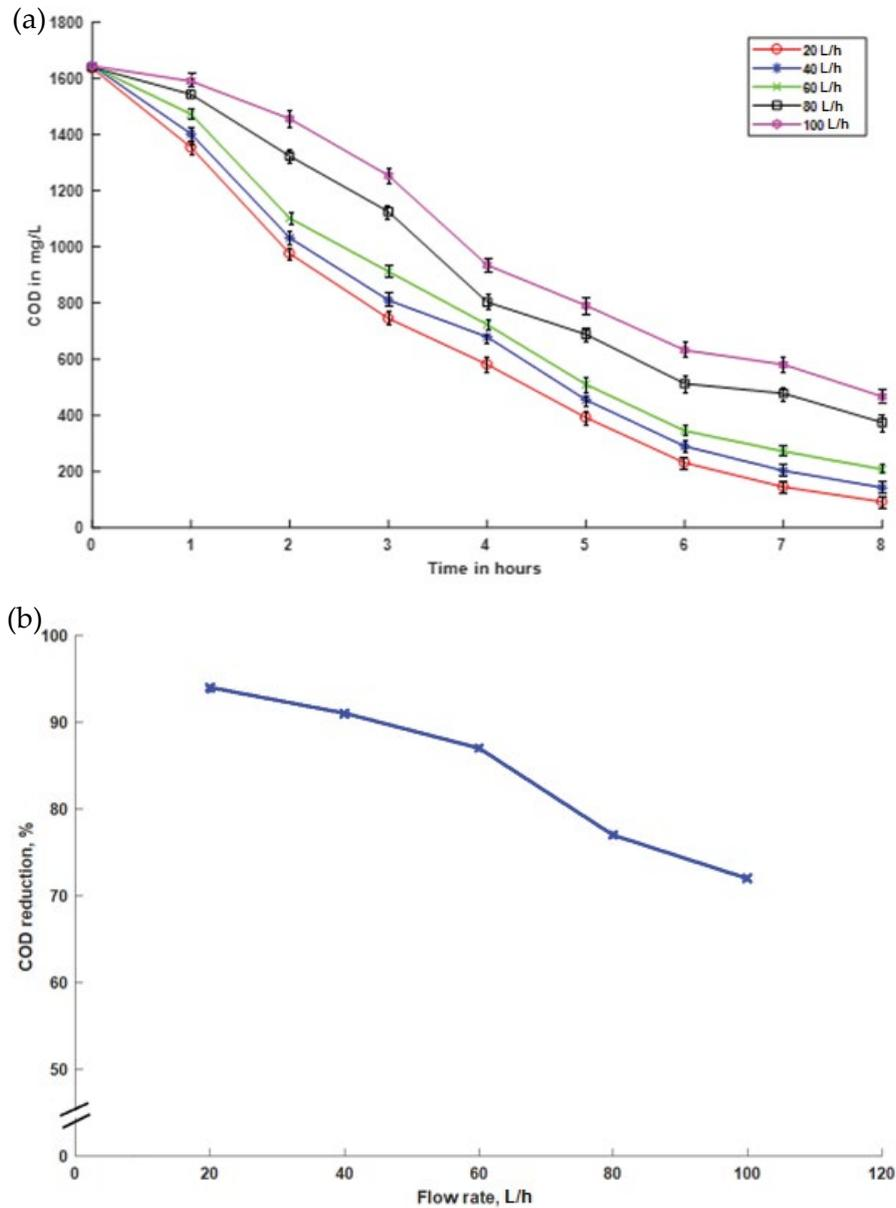
Fig. 3. (a) Reduction of COD vs. time for various flow rates at current density 10 A/dm<sup>2</sup>. (b) COD reduction (%) for various flow rates (L/h).
