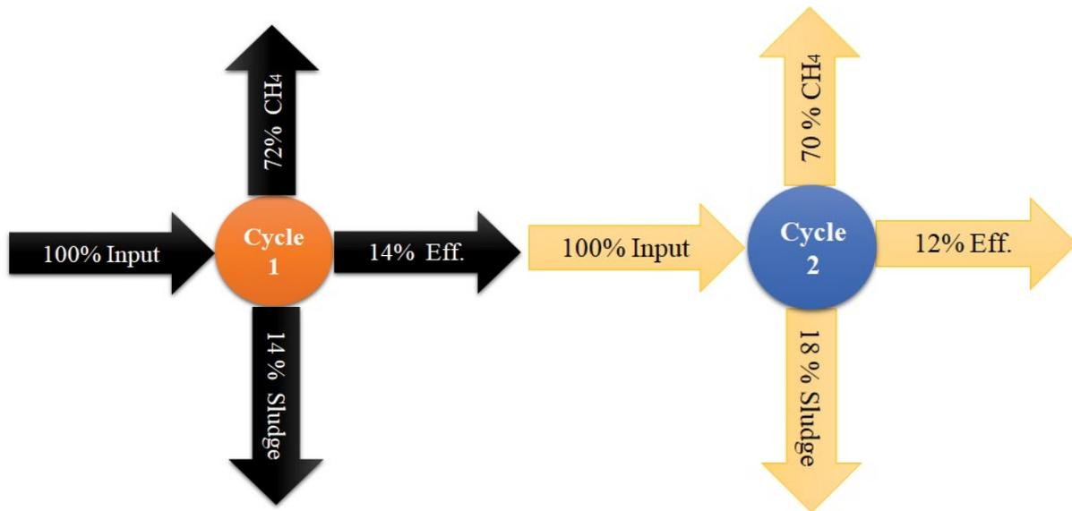
Fig. 11. Behavior of fractions of carbonaceous material mass balance.
