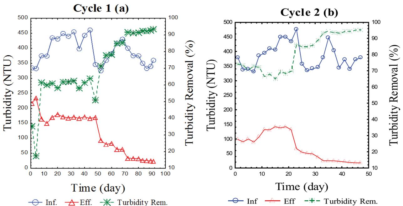
Fig. 5. Turbidity variation in Cycle 1 and 2 during system operation time.
