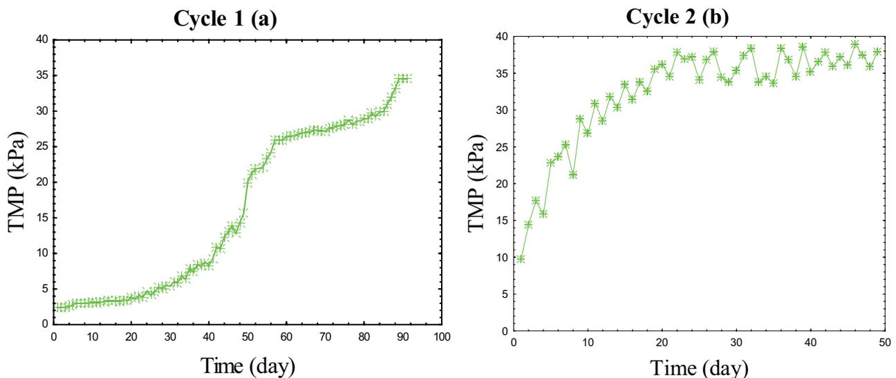
Fig. 3. TMP behavior in Cycle 1 and 2 throughout time of operation.
