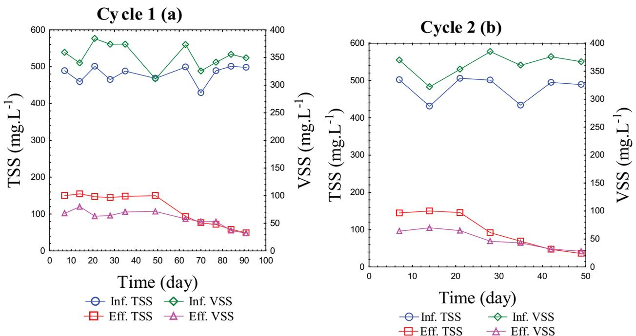
Fig. 6. Average values for fractions of solids for Cycle 1 and 2 during operation.
