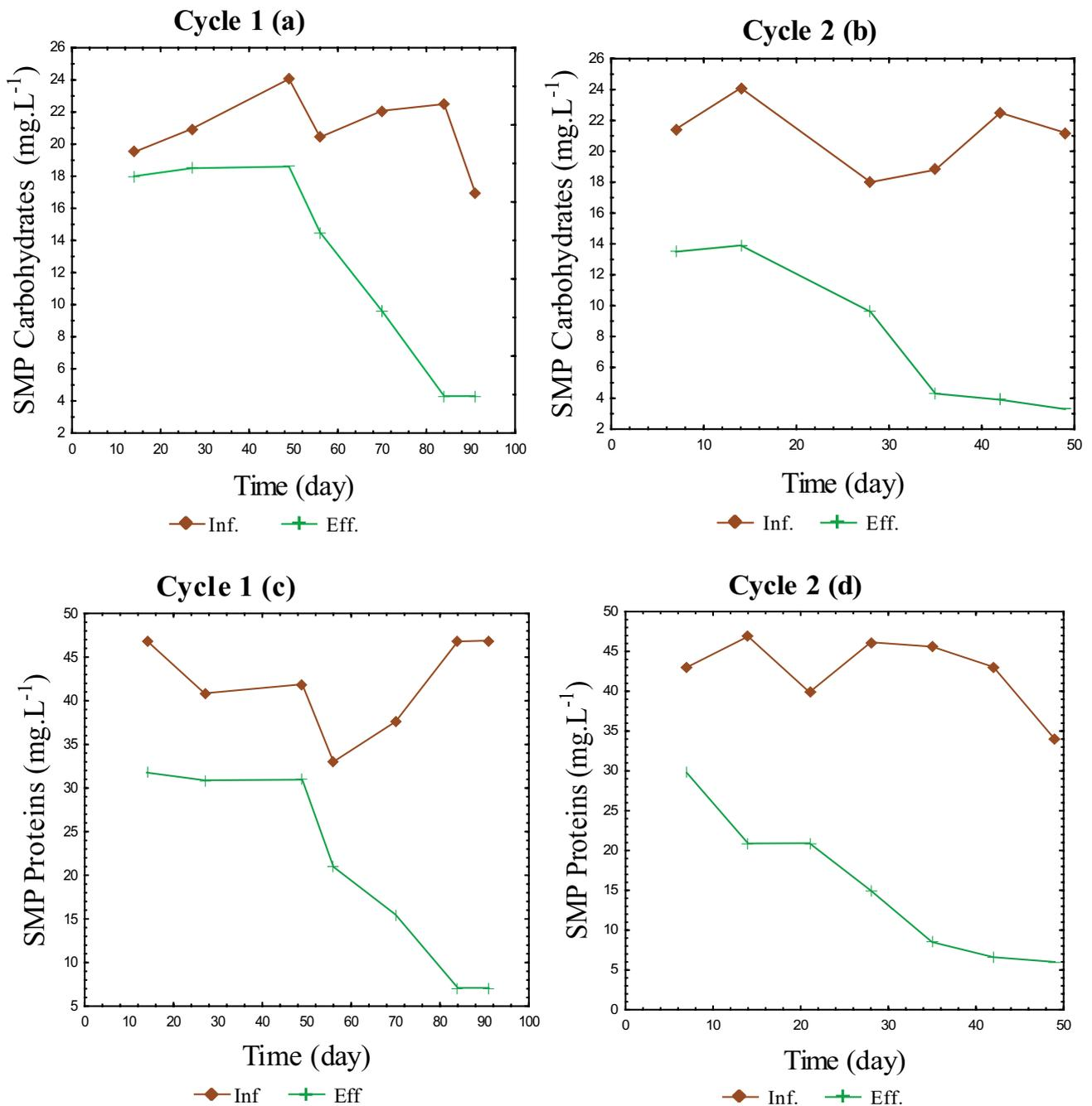
Fig. 8. Carbohydrate and protein concentrations of the influent and effluent, over the period of operation (Cycle 1 and 2).
