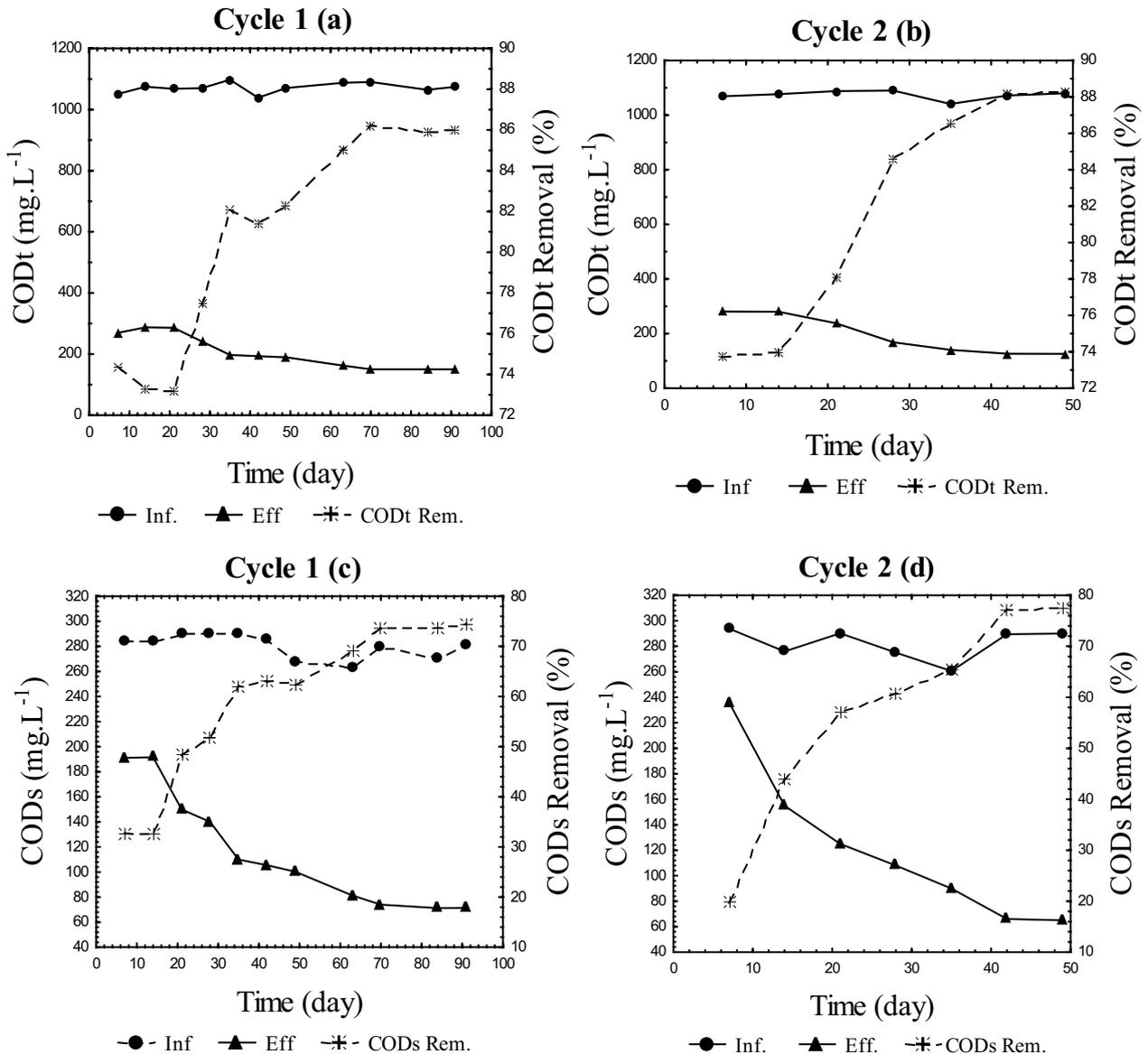
Fig. 7. Variation of total and soluble COD concentrations during system operation time (Cycle 1 and 2).
