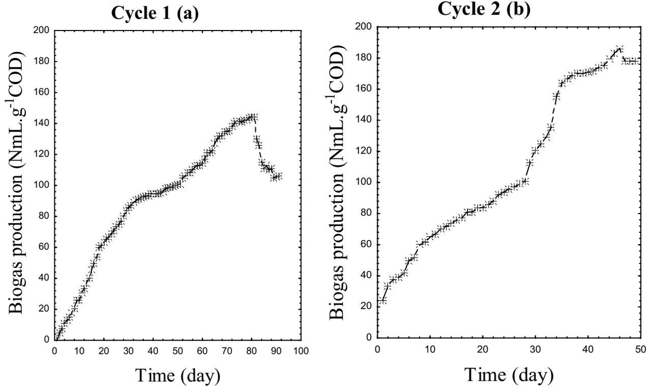
Fig. 10. Behavior of biogas production during Cycle 1 and 2 operation.
