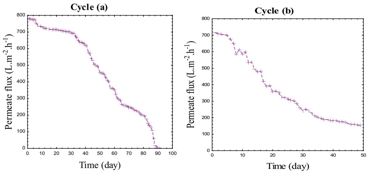
Fig. 4. Permeate flow profile of Cycle 1 and 2 during operating time.
