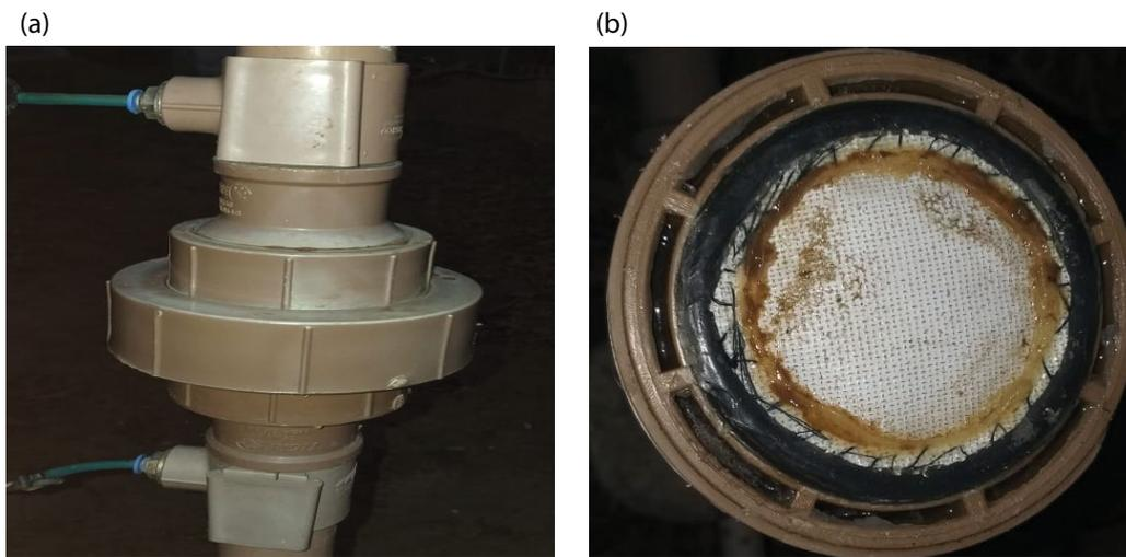
Fig. 2. Dynamic membrane module and support mesh images.
