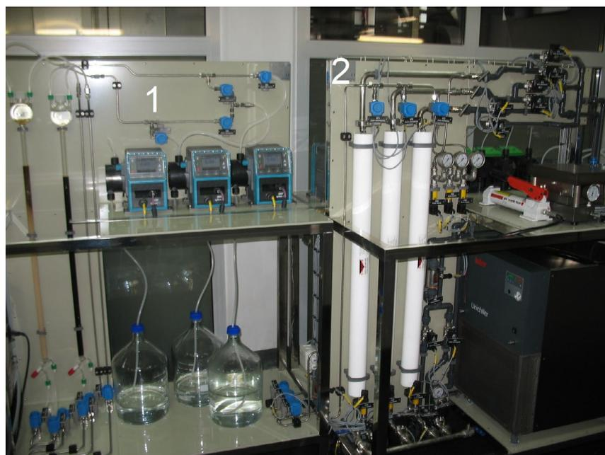
Fig. 2. IE system (1) and NF modules (2) with spiral membranes on the experimental stand at Janówek WWTP Test Station.
