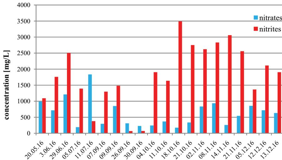
Fig. 3. Changes of nitrates and nitrites concentration in the IE feed tank in the first experiment.
