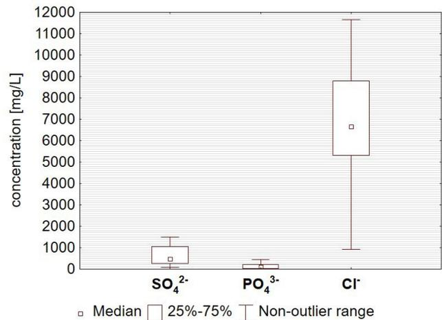
Fig. 11. Anions concentration in eluate 2 from 10% NaCl regeneration.
