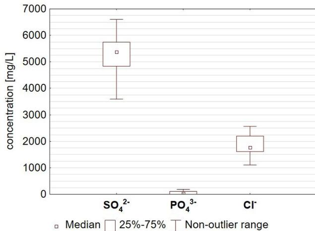
Fig. 14. Anions concentration in eluate 2 from 10% NaHCO<sub>3</sub> regeneration.
