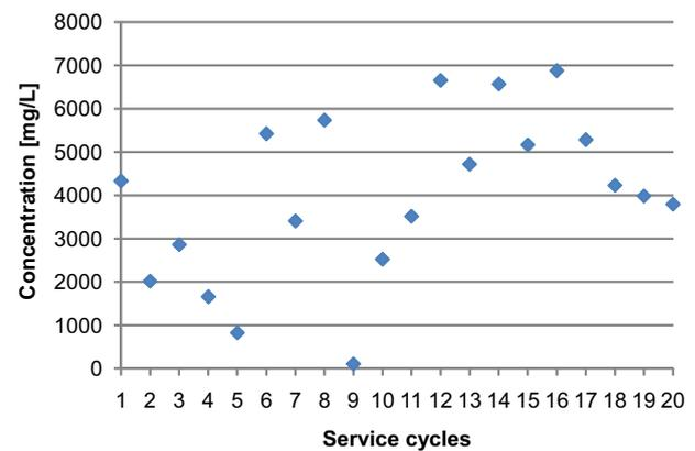
Fig. 16. Nitrite concentration in eluate 1 from 10% NaCl regeneration.
