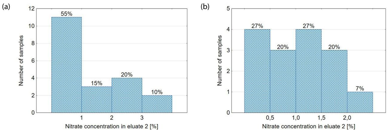
Fig. 9. Frequency distribution of nitrate concentration in eluate 2 from (a) 10% NaCl and (b) 10% NaHCO<sub>3</sub> regeneration.
