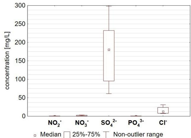
Fig. 15. Anions concentration in eluate 3 taken at the end of fast rinse of Lewatit S 5428 (Lanxess Deutschland GmbH, BU LPT, D-51369 Leverkusen) with distilled water (second experiment).
