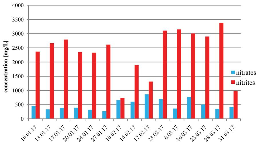
Fig. 4. Changes of nitrates and nitrites concentration in the IE feed tank in the second experiment.
