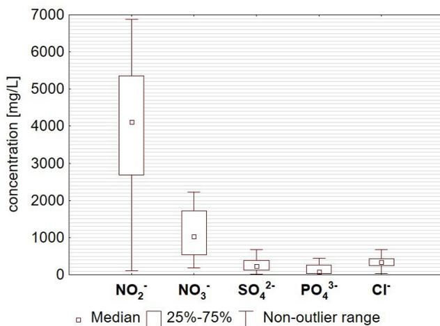
Fig. 10. Anions concentration in eluate 1 from 10% NaCl regeneration.
