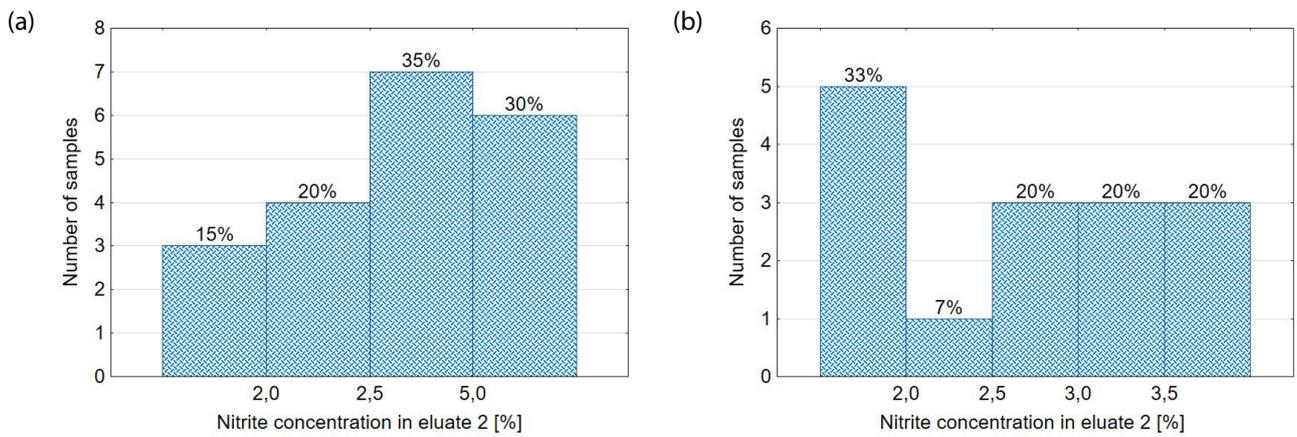
Fig. 8. Frequency distribution of nitrite concentration in eluate 2 from (a) 10% NaCl and (b) 10% NaHCO<sub>3</sub> regeneration.
