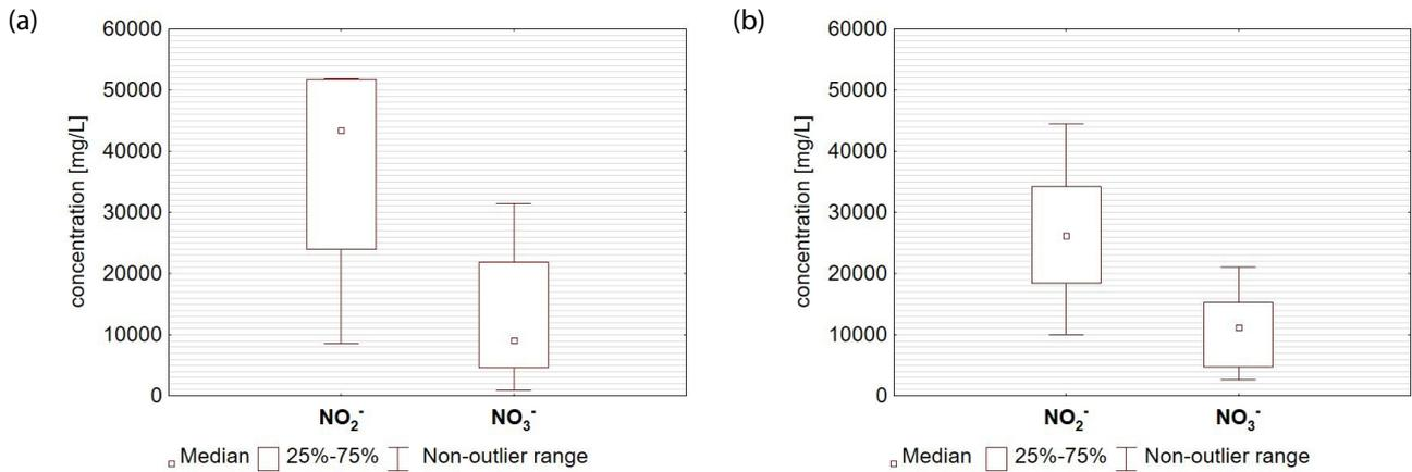
Fig. 7. Nitrite and nitrate concentration in eluate 2 from (a) 10% NaCl and (b) 10% NaHCO<sub>3</sub> regeneration.
