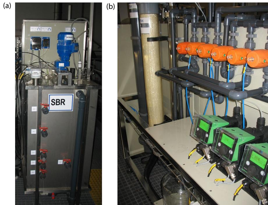
Fig. 1. SBR (a) and microfiltration system and (b) on the experimental stand at Janówek WWTP Test Station.
