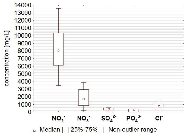
Fig. 12. Anions concentration in eluate 3 taken at the end of fast rinse of Lewatit S 5428 (Lanxess Deutschland GmbH, BU LPT, D-51369 Leverkusen) with distilled water (first experiment).
