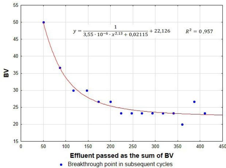
Fig. 6. Decrease of total capacity in the second experiment.
