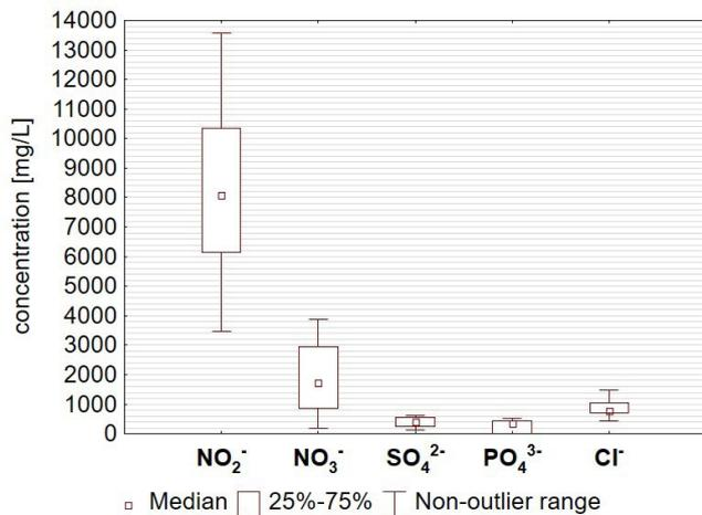
Fig. 13. Anions concentration in eluate 1 from 10% NaHCO<sub>3</sub> regeneration.
