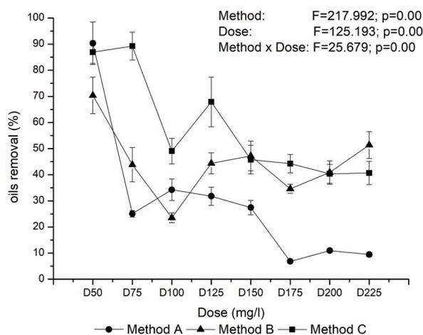
Fig. 4. Oil (C12–C35) removal percentage efficiency using the coagulation; A – aluminum sulfate(VI), B – iron(III) chloride, C – ultrasounds, and iron(III) chloride.
