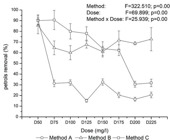
Fig. 3. Petrol (C6–C12) removal percentage efficiency using the coagulation; A – aluminum sulfate(VI), B – iron(III) chloride, C – ultrasounds, and iron(III) chloride.
