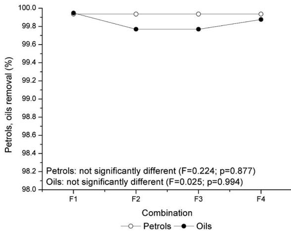
Fig. 5. Petrol (C6–C12) and oil (C12–C35) removal percentage efficiency using the Fenton's method; ratio of  $\text{Fe}^{2+}:\text{H}_2\text{O}_2$ ; F1-1:6, F2-1:10, F3-1:3, F4-1:5.
