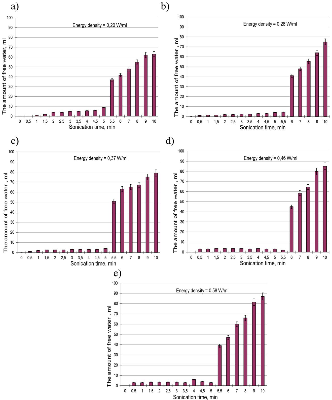
Fig. 2. Amount of free water released from the sewage sludge disintegrated with the ultrasound field (a) energy density 0.20 W/ml, (b) energy density 0.28 W/ml, (c) energy density 0.37 W/ml, (d) energy density 0.46 W/ml, and (e) energy density 0.58 W/ml; sludge time 30 min.
