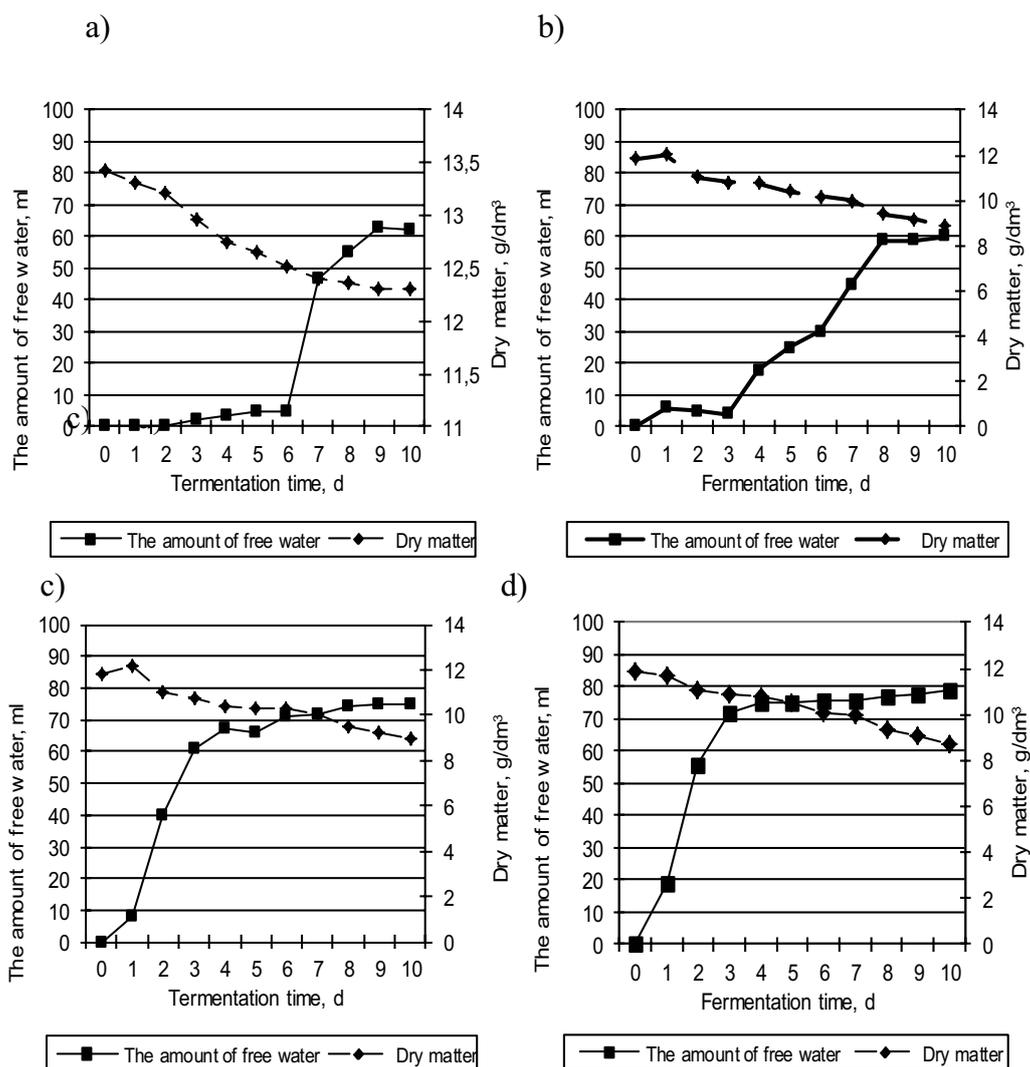
Fig. 3. Volume of free water and dry matter of sewage sludge formed during the stabilization process: (a) non-conditioned sludge, (b) sludge + ultrasound field 0.37 W/ml, (c) sludge + ultrasound field 0.46 W/ml, and (d) sludge + ultrasound field 0.58 W/ml; sedimentation time 30 min; sonication time 5 min.
