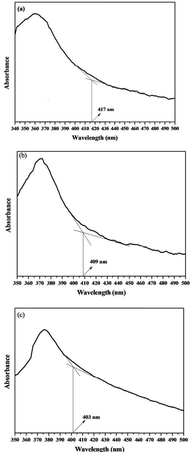
Fig. 4. UV-vis spectra of (a) ZB4, (b) ZB5, and (c) ZB6 photocatalyst.
