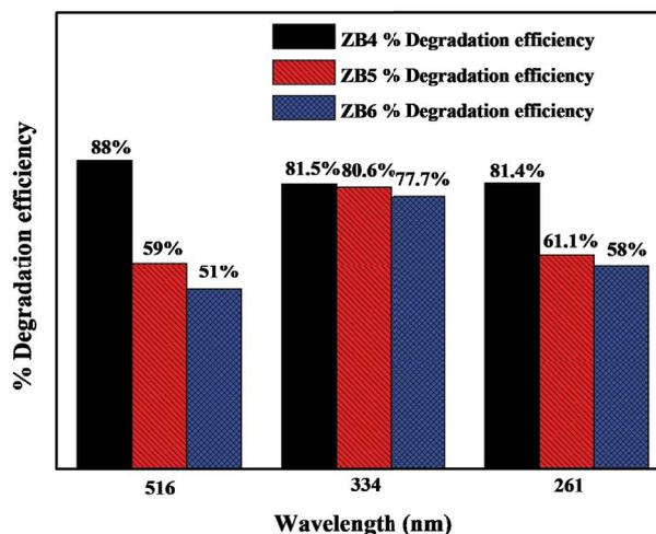
Fig. 6. Comparison of percentage degradation of ARS dye solution (dye concentration – 20 mg/L, pH – 6.7 (neutral), time – 13 h) using ZB4, ZB5, and ZB6 photocatalyst (0.1 g/100 mL) at different peaks 516, 334, and 261 nm.
