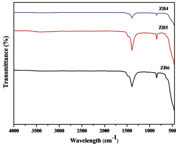
Fig. 3. FT-IR spectra of ZB4, ZB5, and ZB6 photocatalyst.
