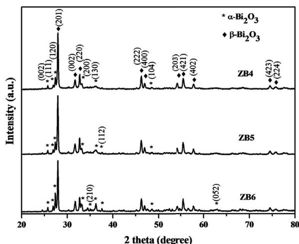
Fig. 1. XRD patterns of ZB4, ZB5, and ZB6 photocatalyst.
