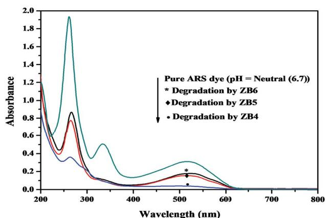
Fig. 5. UV-vis absorption spectral changes of ARS dye solution in the presence of ZB4, ZB5, and ZB6 photocatalyst at neutral pH (6.7) (dye concentration – 20 mg/L, catalyst dose – 0.1 g/100 mL, time – 13 h).
