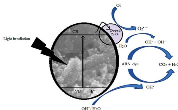
Fig. 7. Schematic diagram of the photocatalytic degradation mechanism of ZB4 photocatalyst.
