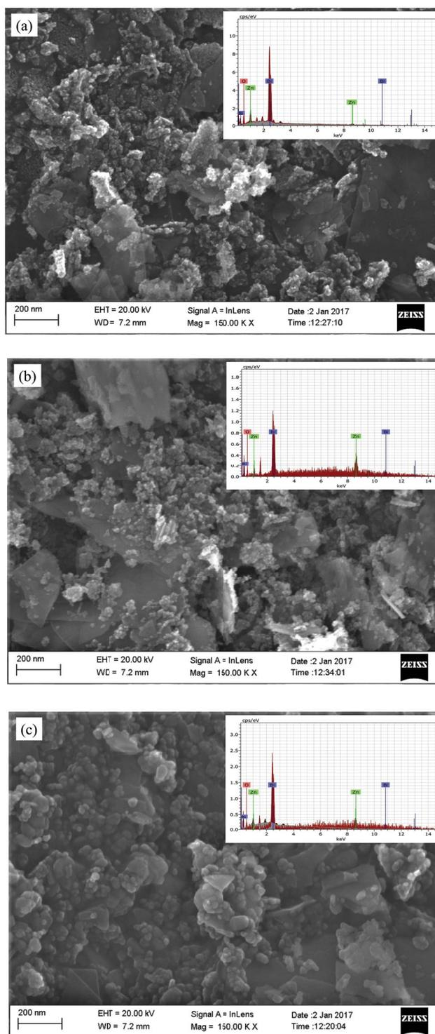
Fig. 2. FESEM images and EDS spectra of (a) ZB4, (b) ZB5, and (c) ZB6 photocatalyst.
