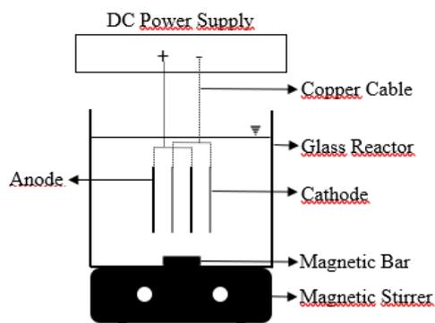
Fig. 1. Schematic diagram of the electrochemical set-up.
