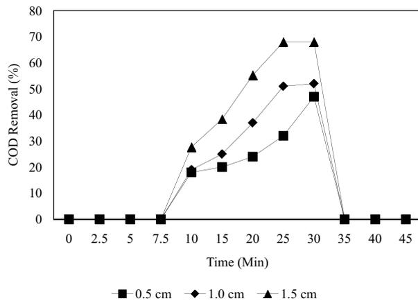
Fig. 6. The effect of distance between the electrodes on COD removal (conditions: anode: iron; cathode: steel; pH: 3;  $H_2O_2$ : 2,000 mg/L; stirring rate: 250 rpm).
