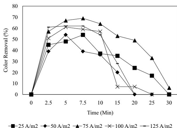
Fig. 5. The effect of current density on color removal (conditions: anode: iron; cathode: steel; pH: 3; H<sub>2</sub>O<sub>2</sub>: 2,000 mg/L; stirring rate: 250 rpm; the distance of electrodes: 1.5 cm).
