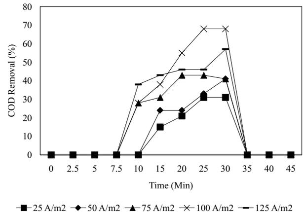
Fig. 4. The effect of current density on COD removal (conditions: anode: iron; cathode: steel; pH: 3; H<sub>2</sub>O<sub>2</sub>: 2,000 mg/L; stirring rate: 250 rpm; the distance of electrodes: 1.5 cm).
