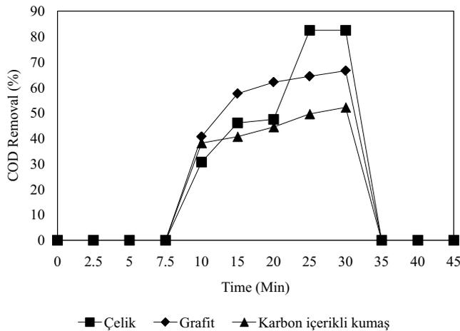
Fig. 2. The effect of cathode material on COD removal (conditions: anode: iron, pH: 3; current density: 100 A/m<sup>2</sup>; H<sub>2</sub>O<sub>2</sub>: 2,000 mg/L; stirring rate: 250 rpm; the distance of electrodes: 1.5 cm).
