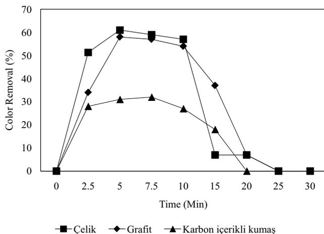
Fig. 3. The effect of cathode material on color removal (conditions: anode: iron; pH: 3; current density: 100 A/m<sup>2</sup>; H<sub>2</sub>O<sub>2</sub>: 2,000 mg/L; stirring rate: 250 rpm; the distance of electrodes: 1.5 cm).
