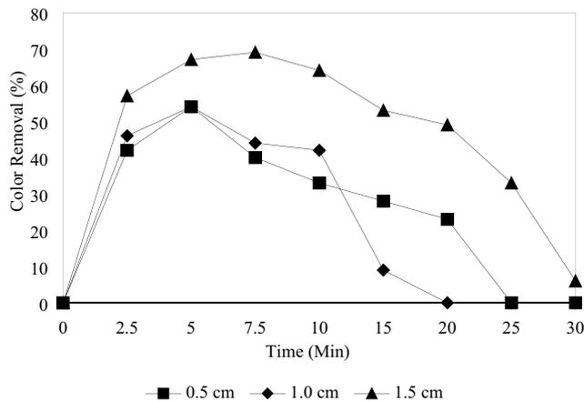
Fig. 7. The effect of distance between the electrodes on color removal (conditions: anode: iron; cathode: steel; pH: 3;  $H_2O_2$ : 2,000 mg/L; stirring rate: 250 rpm).
