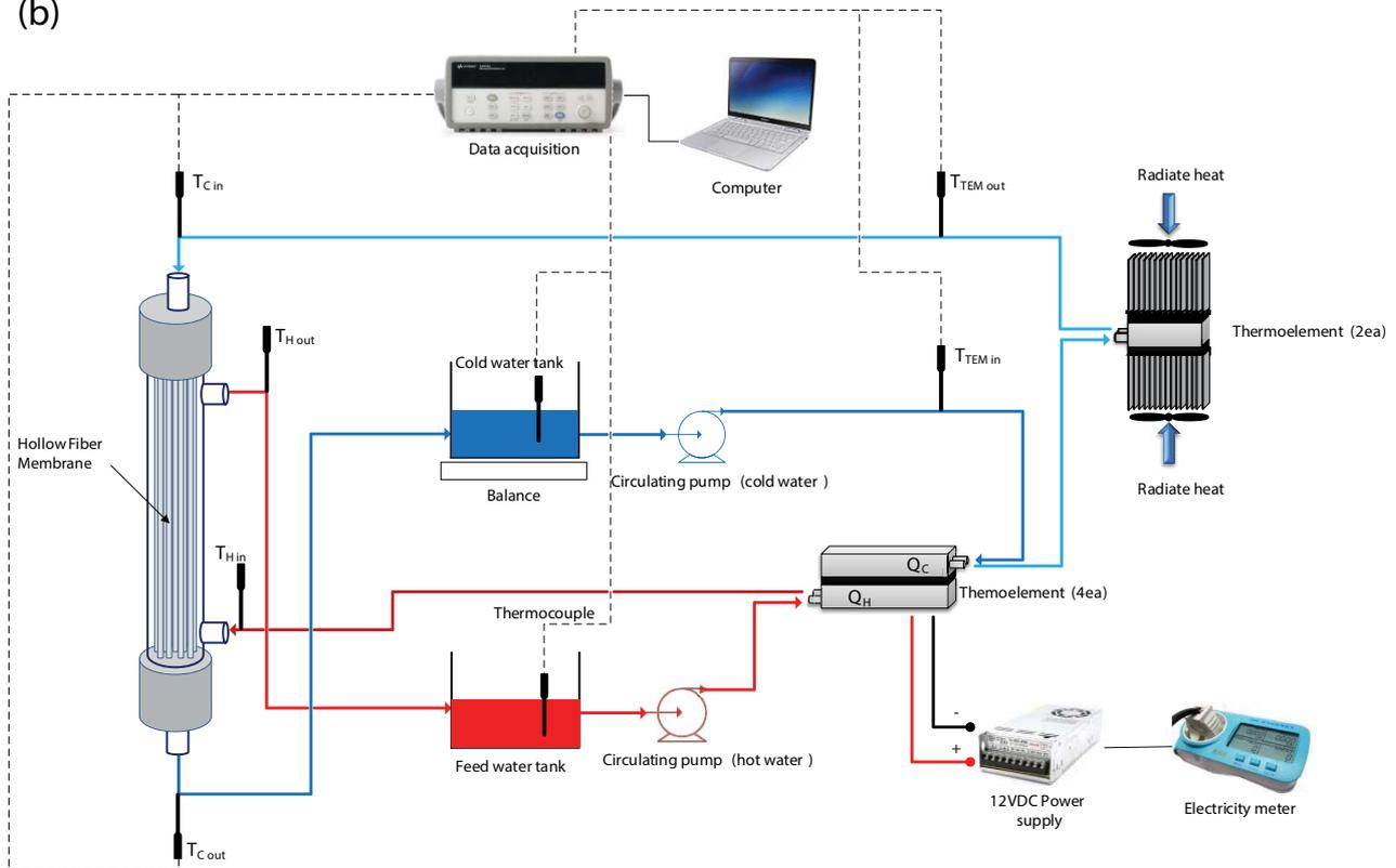
Fig. 3. (a) Schematic of the DCMD-TEM system and (b) schematic of the CEDCMD-TEM system
