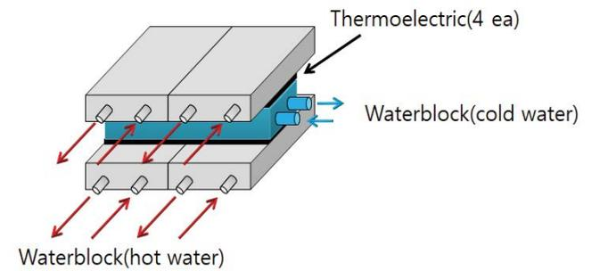
Fig. 1. Schematic of water block including TEMs used in this study.
