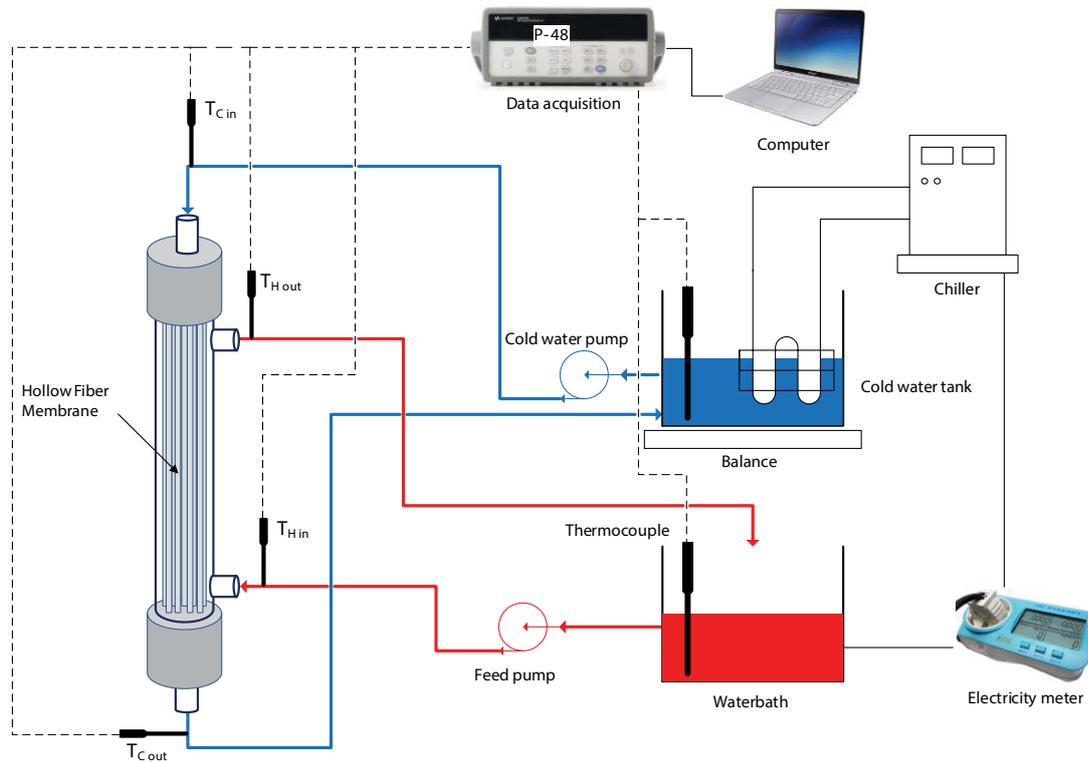
Fig. 2. Schematic of the conventional DCMD system.
