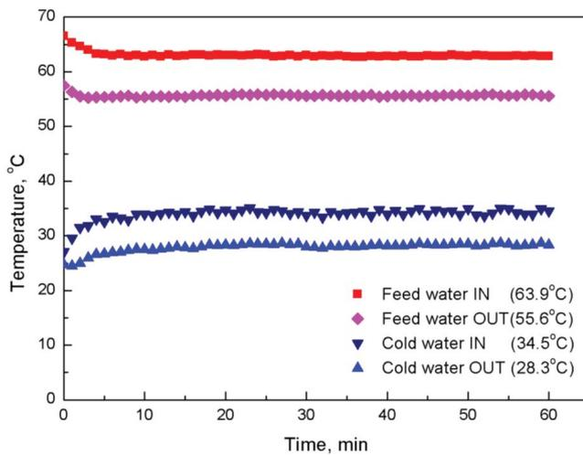
Fig. 4. Operational results of the conventional DCMD system.
