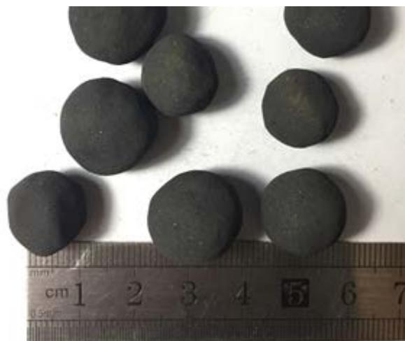
Fig. 2. Iron–carbon micro-electrolytic filler.
