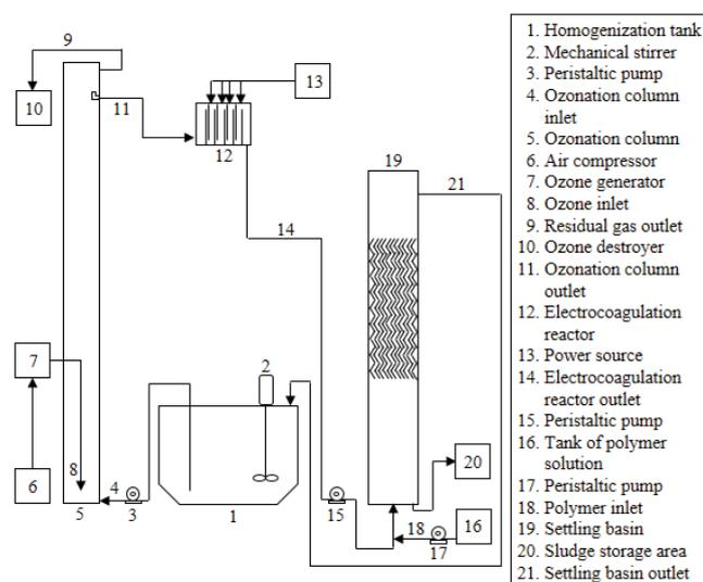
Fig. 1. Treatment system used in the study.
