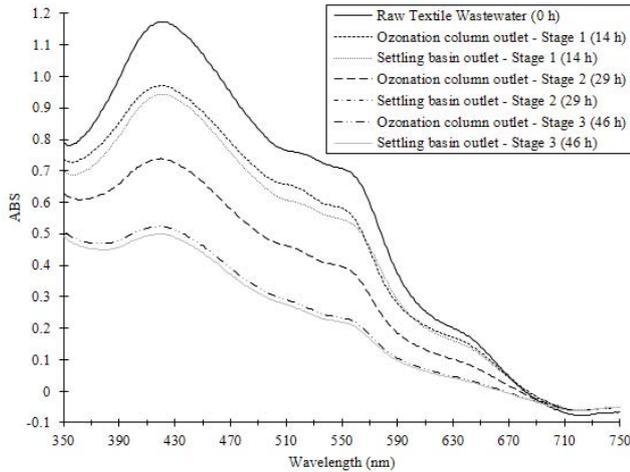
Fig. 3. Spectral scan of textile wastewater before and after the experimental stages 1 ( $O_3$ : 13.6 mg/L; EC: 15.8 A), 2 ( $O_3$ : 13.6 mg/L; EC: 22.1 A) and 3 ( $O_3$ : 13.6 mg/L; EC: 28.5 A).
