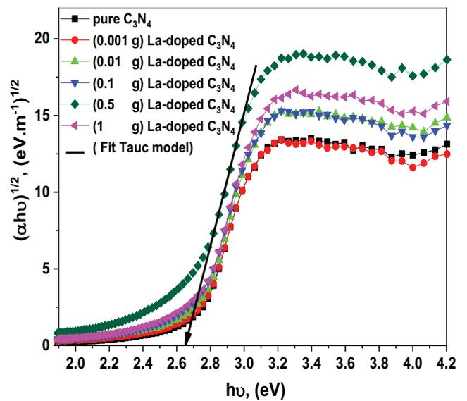
Fig. 4. Plots of  $(\alpha h\nu)^{1/2}$  vs. the incident photon energy hν for the investigated samples.
