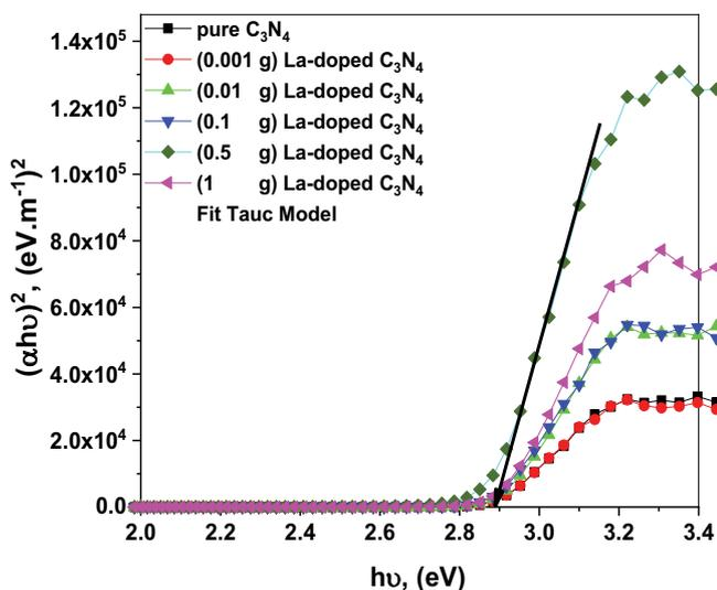
Fig. 5. Plots of  $(\alpha h\nu)^2$  vs. the incident photon energy  $h\nu$  for the as-prepared samples.
