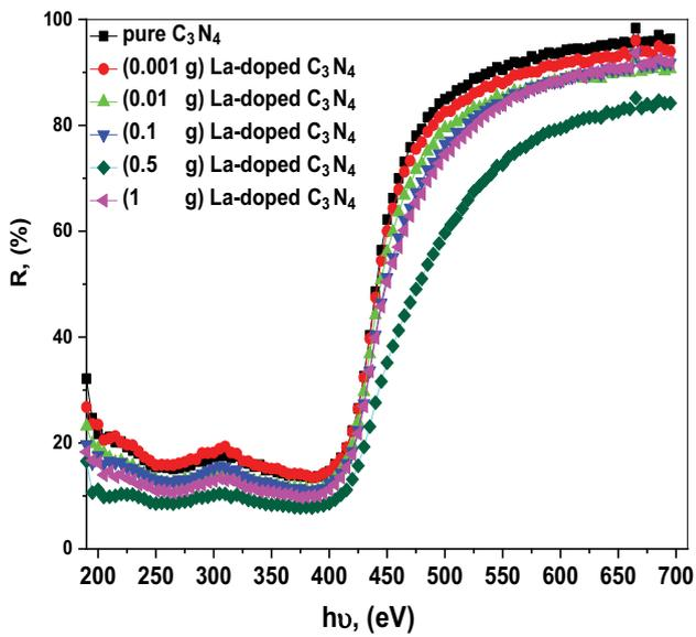
Fig. 3. UV-vis diffused reflectance of pure g-C<sub>3</sub>N<sub>4</sub> and La doped g-C<sub>3</sub>N<sub>4</sub> samples with various La ion concentrations.
