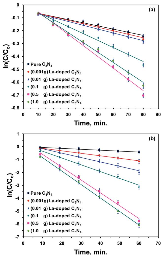
Fig. 6. (a and b) Effect of photodegrading MB dye on the first order kinetic adjustment curves of the photocatalytic samples.
