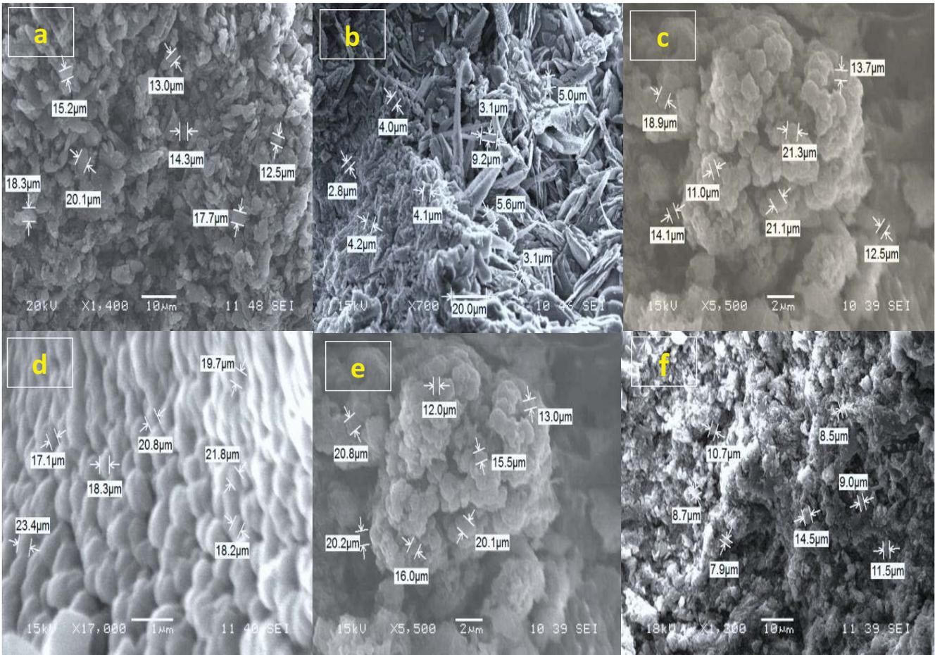
Fig. 2. SEM micrographes of (a) pure g-C<sub>3</sub>N<sub>4</sub>, (b) 0.001 La-C<sub>3</sub>N<sub>4</sub>, (c) 0.01 La-C<sub>3</sub>N<sub>4</sub>, (d) 0.1 La-C<sub>3</sub>N<sub>4</sub>, (e) 0.5 La-C<sub>3</sub>N<sub>4</sub>, and (f) 1 La-C<sub>3</sub>N<sub>4</sub>.
