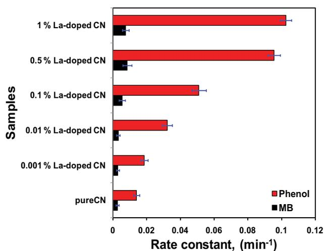
Fig. 7. MB evolution rate constants during photocatalytic degradation for the samples under visible light irradiation.
