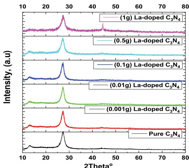
Fig. 1. XRD distributions of pure  $g\text{-C}_3\text{N}_4$  and La nitrate ions doped  $g\text{-C}_3\text{N}_4$  samples with various amounts of La (0.001, 0.01, 0.1, 0.5, and 1.0 g La).
