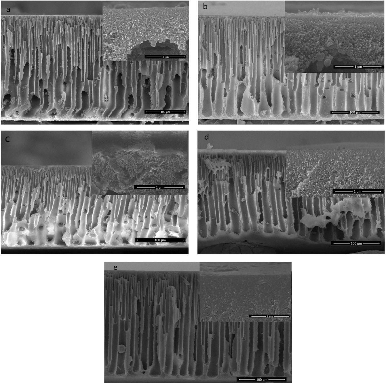
Fig. 2. Cross-section morphology of the polyimide membranes with different polymer contents (the insets are the morphologies of the skin layer with a magnification of 100,000, (a) 12 wt.%, (b) 13 wt.%, (c) 14 wt.%, (d) 15 wt.%, and (e) 16 wt.%.
