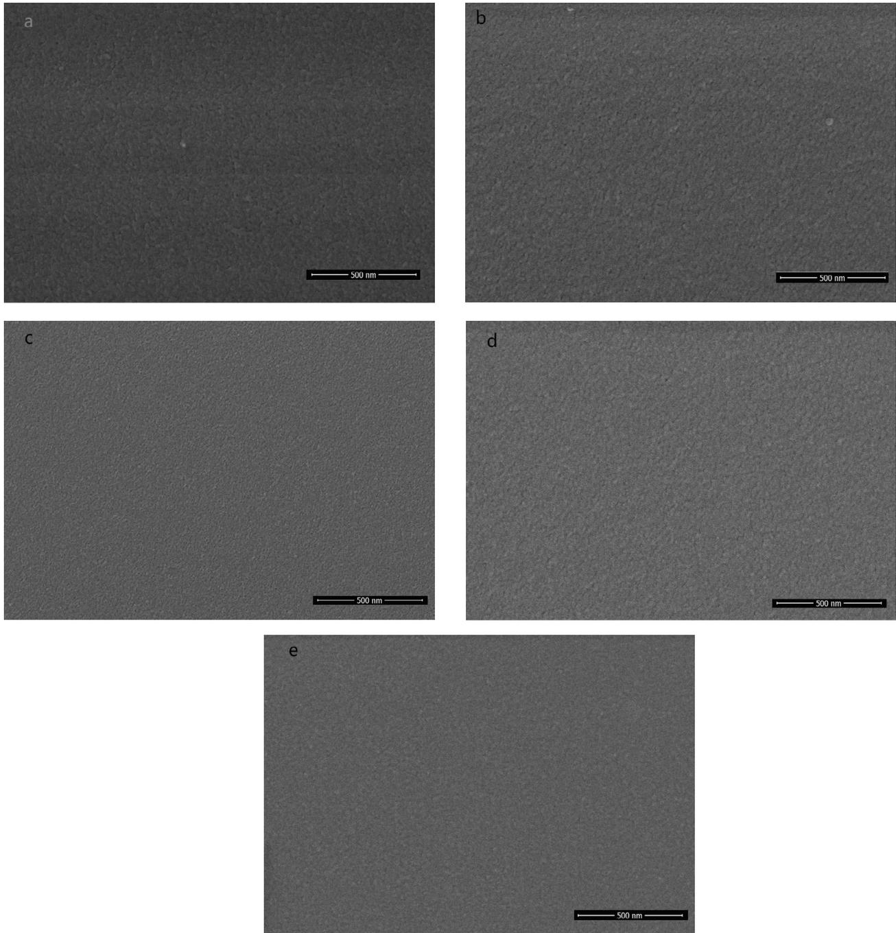
Fig. 5. Top surface morphology of the polyimide membranes with different PVP contents (a) 1 wt.%, (b) 2 wt.%, (c) 3 wt.%, (d) 4 wt.%, and (e) 5 wt.%.
