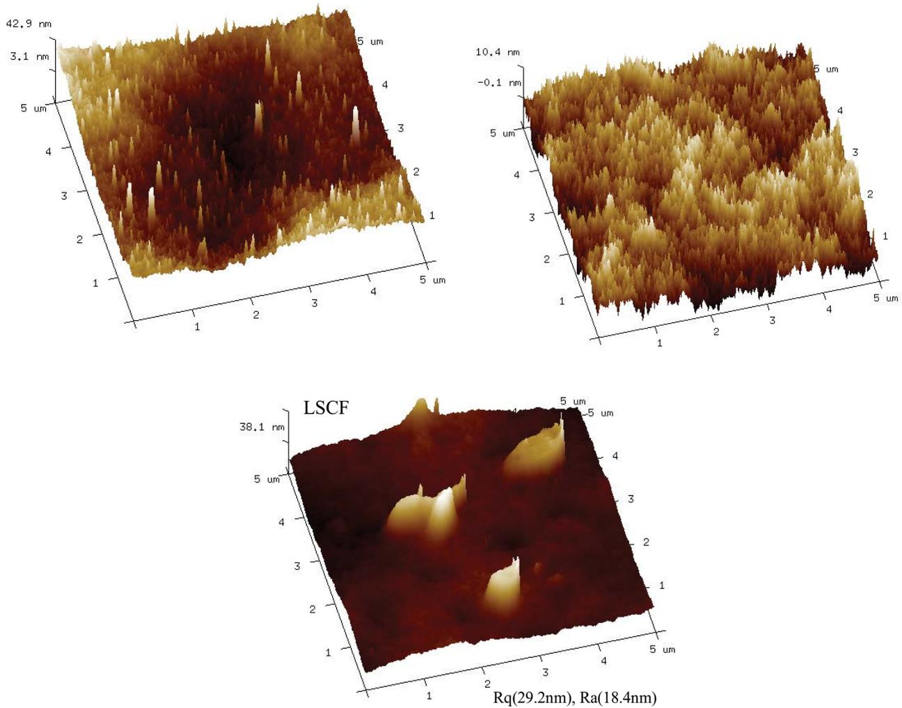
Fig. 11. AFM images of the polyimide membrane (no additive, bare polyimide membrane; PVP, membrane with 5 wt.% PVP; LSCF, membrane with 4 wt.% LSCF).
