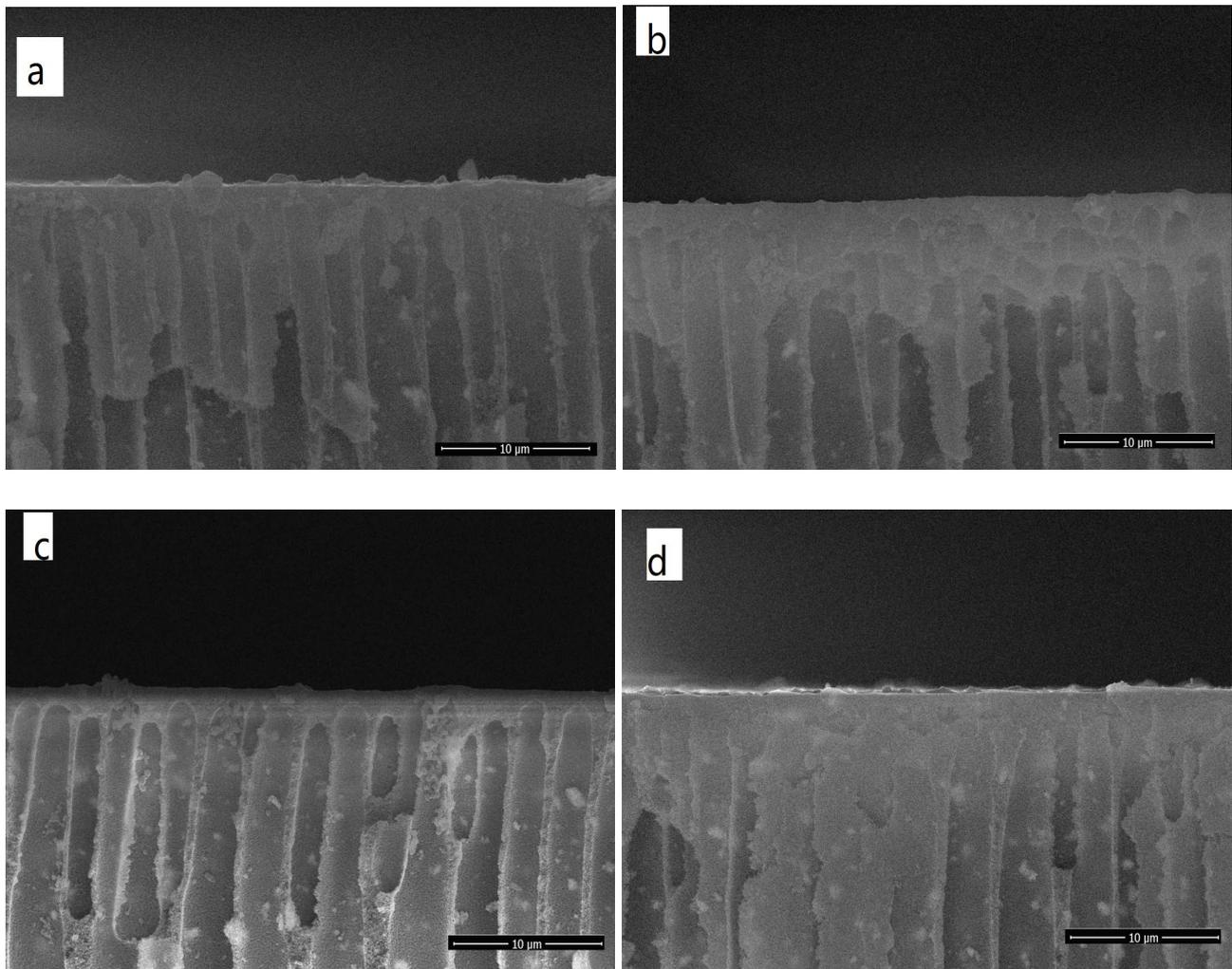
Fig. 9. Cross-section morphology of polyimide membranes with different LSCF content (a) 1 wt.%, (b) 2 wt.%, (c) 3 wt.%, and (d) 4 wt.%.
