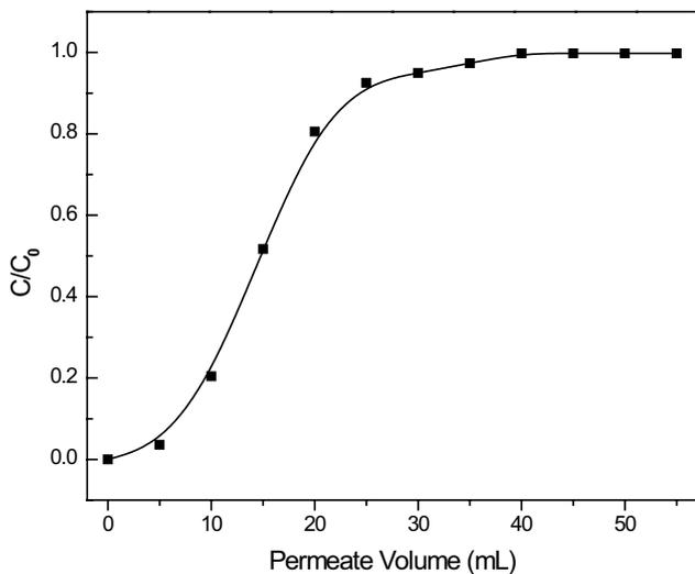
Fig. 12. Dynamic adsorption for bilirubin of P84® membrane.
