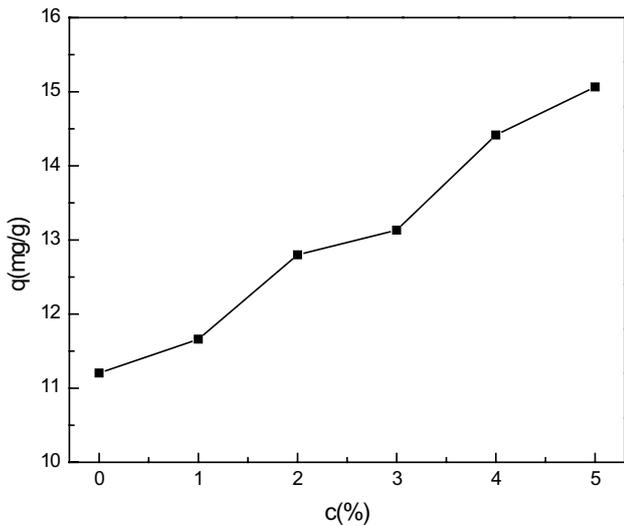
Fig. 7. Effect of PVP content on the adsorption capacity of the affinity membrane.
