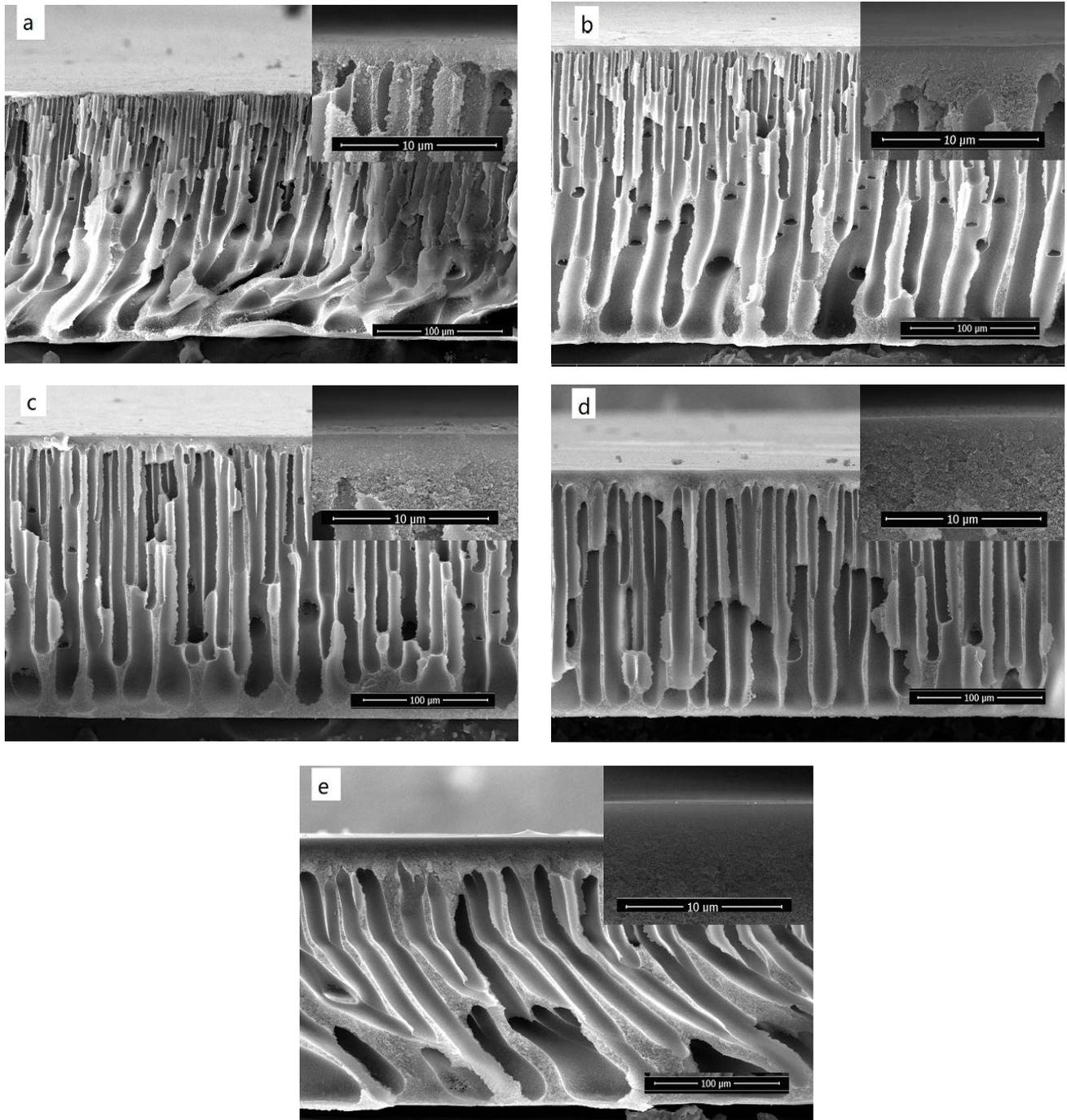
Fig. 6. Cross-section morphology of the polyimide membranes skin layer with different PVP contents (the insets are the morphologies of the skin layer with a magnification of 10,000 (a) 1 wt.%, (b) 2 wt.%, (c) 3 wt.%, (d) 4 wt.%, and (e) 5 wt.%).
