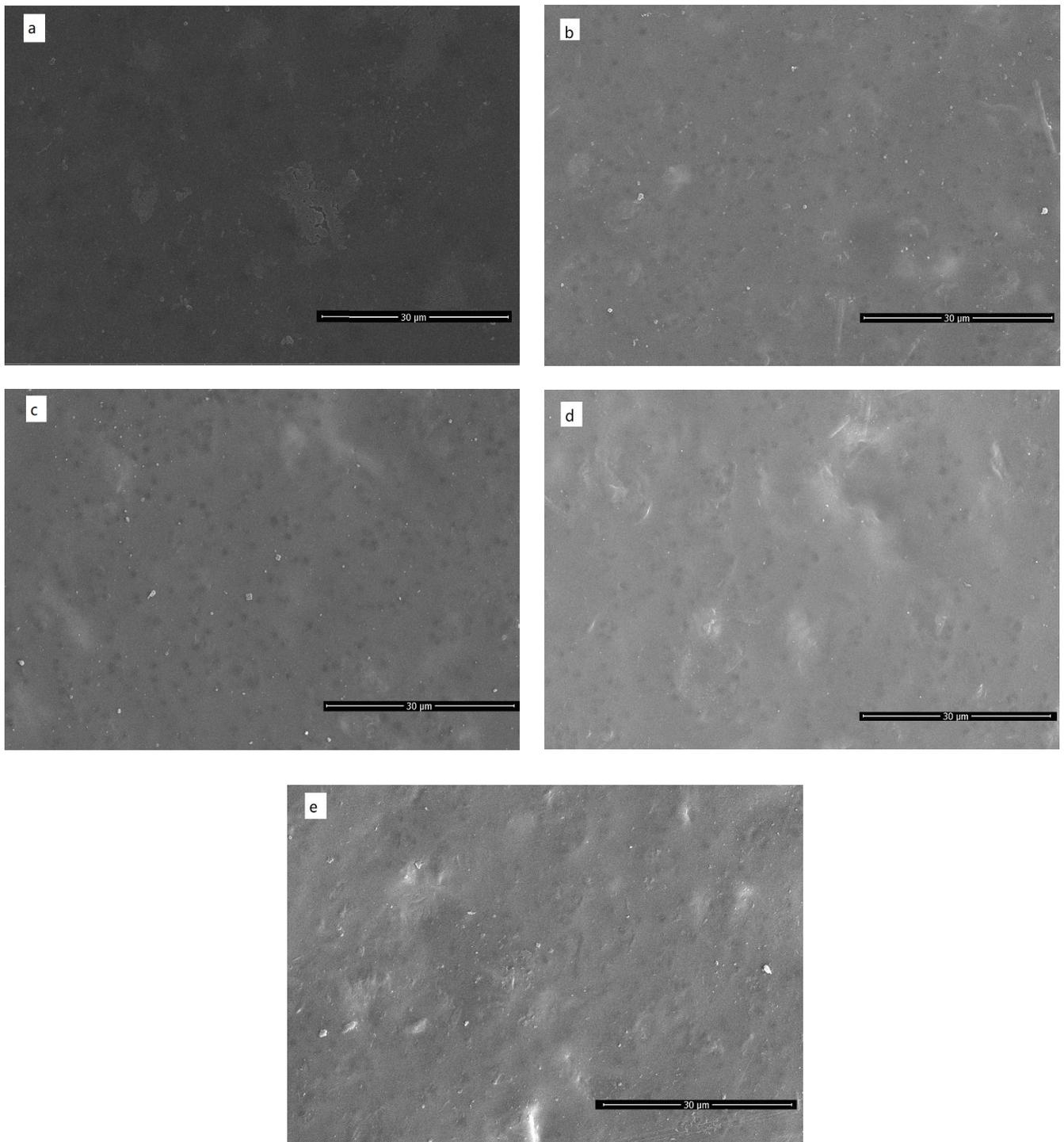
Fig. 1. Top surface morphology of polyimide membranes with different polymer content (a) 12%, (b) 13%, (c) 14%, (d) 15%, and (e) 16%.
