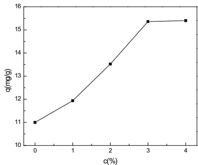
Fig. 10. Effect of LSCF content on the adsorption capacity of the affinity membrane.
