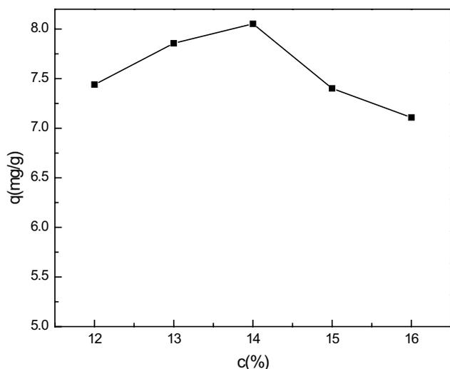
Fig. 3. Effect of polyimide concentration on the bilirubin adsorption.
