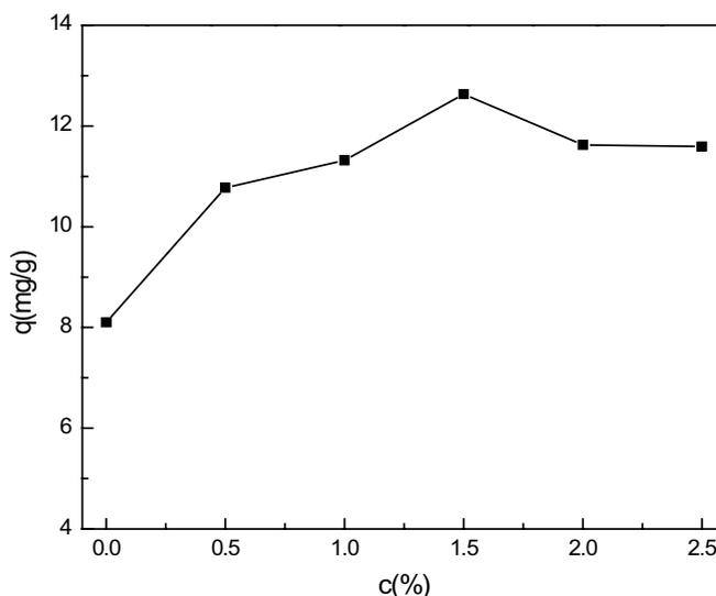
Fig. 4. Effect of PEI concentration on the adsorption capacity of affinity membrane.
