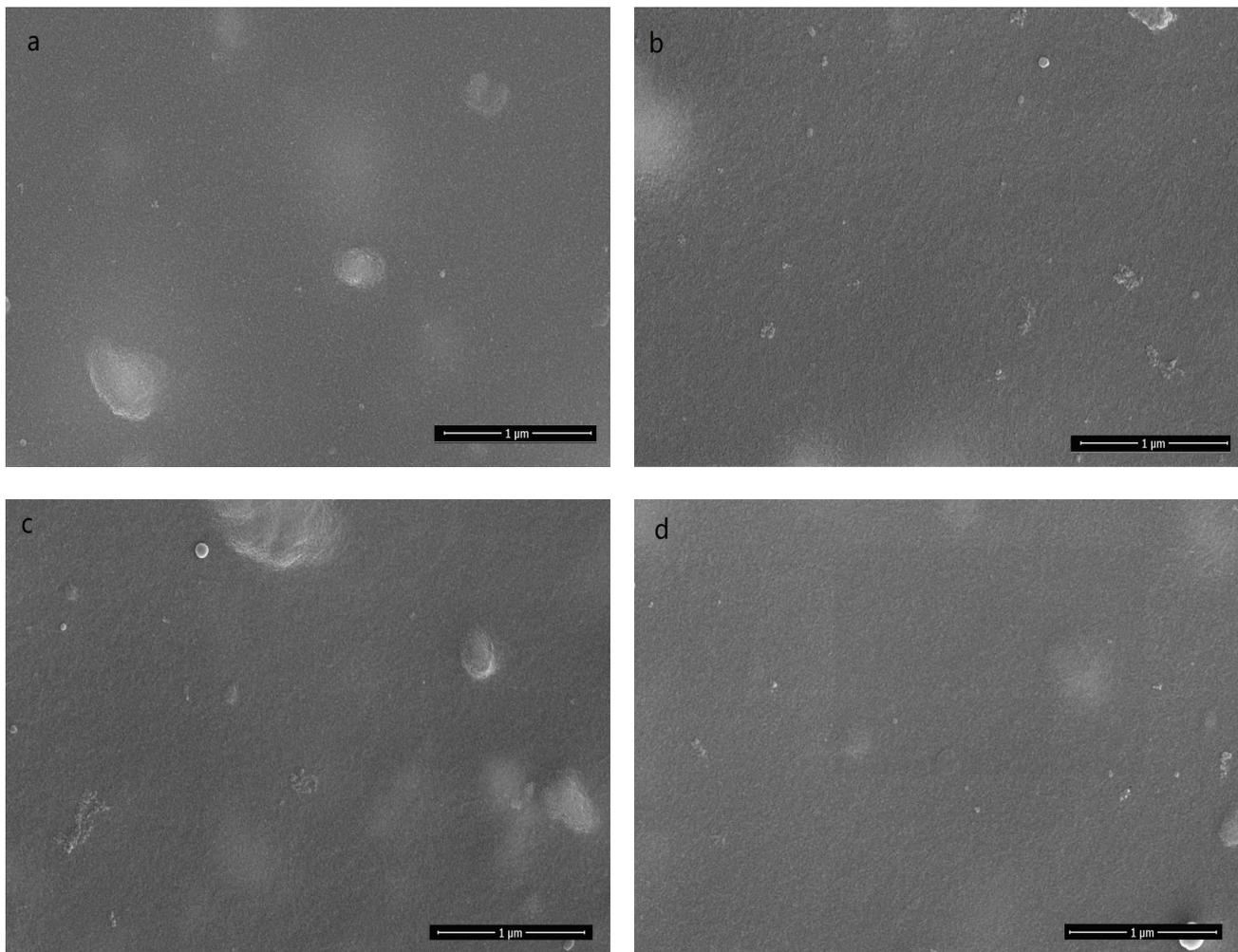
Fig. 8. Top surface morphology of polyimide membranes with different LSCF contents (a) 1 wt.%, (b) 2 wt.%, (c) 3 wt.%, and (d) 4 wt.%.
