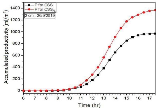
Fig. 6. Accumulative produced freshwater at 1 and 2 cm depths.
