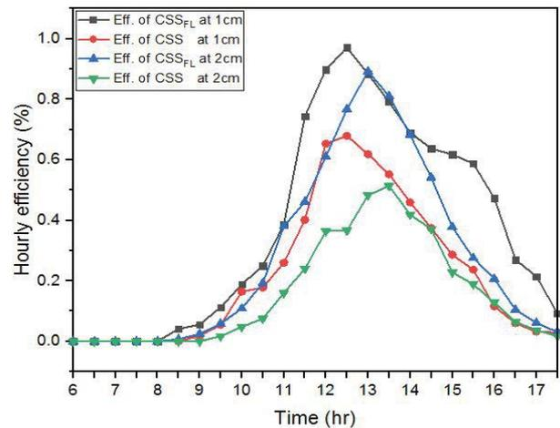
Fig. 7. Variation of hourly thermal efficiency of CSS and CSS<sub>FL</sub> at different depths (July experiments).
