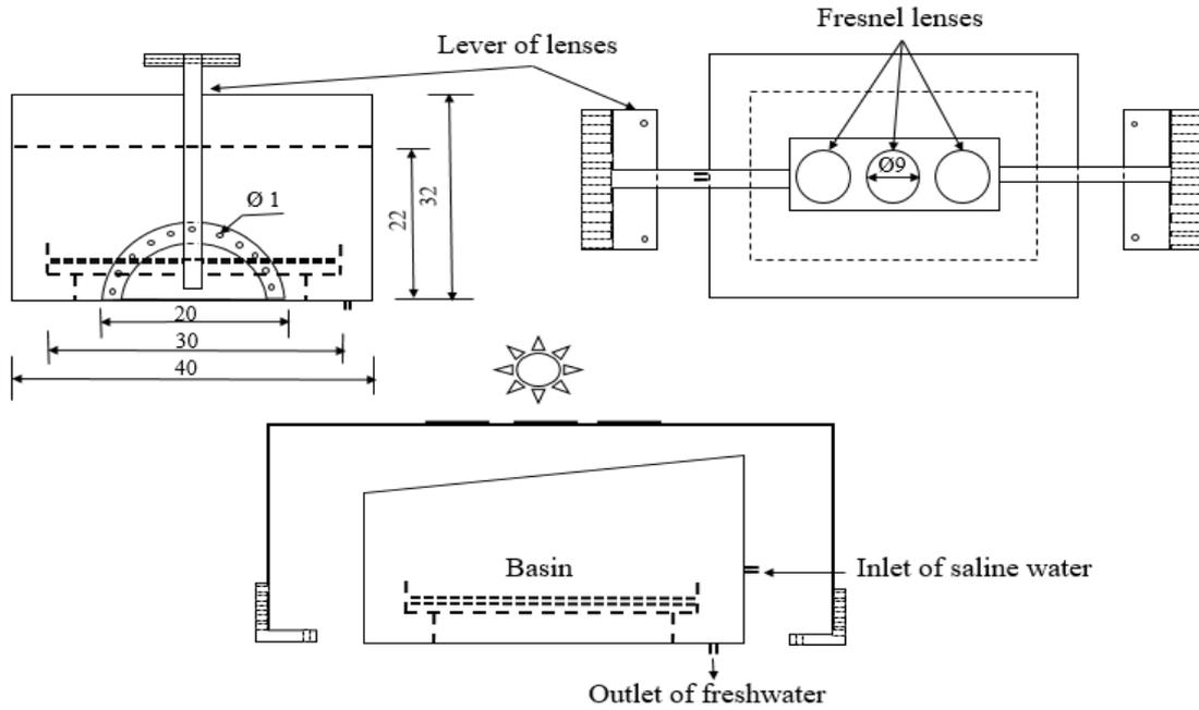
Fig. 2. 2D schematic view of the modified solar still.
