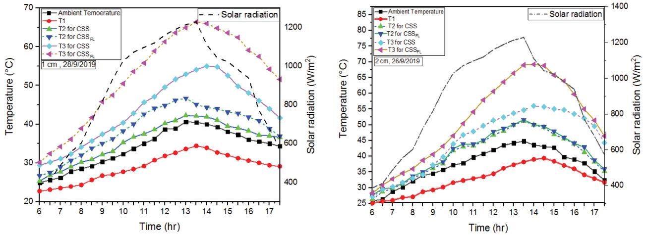
Fig. 4. Temperature variation for CSS and CSS<sub>FL</sub> at 1 and 2 cm depth in September 2019.
