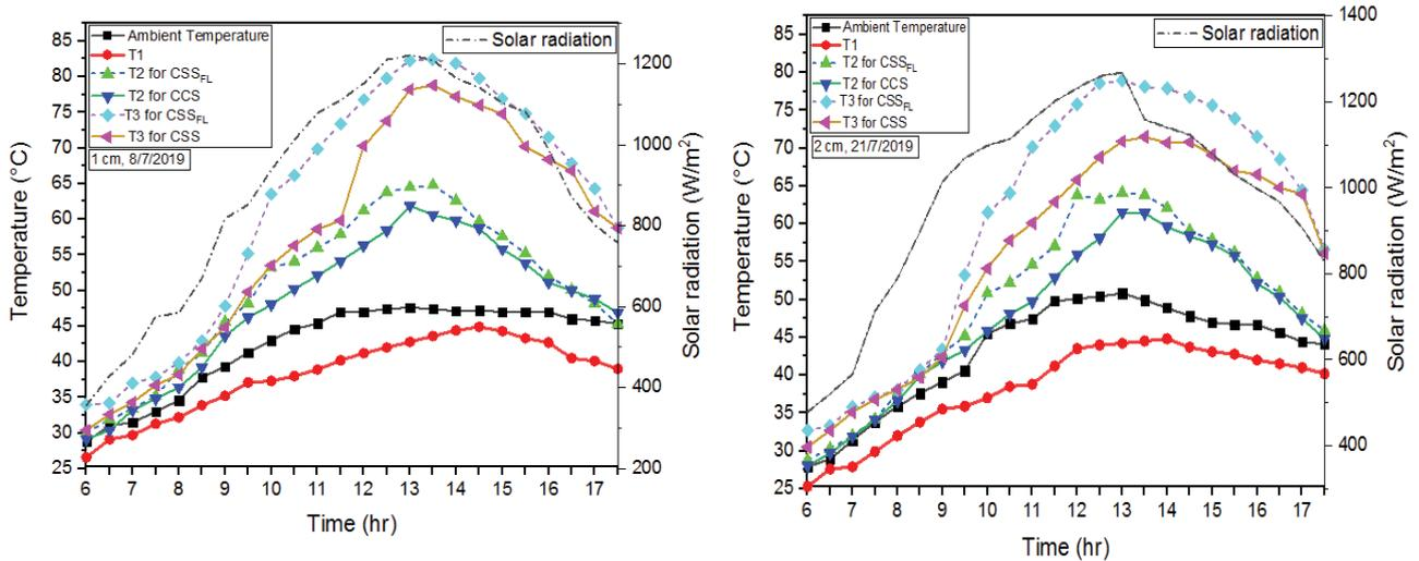
Fig. 3. Temperature variation for CSS and CSS<sub>FL</sub> at 1 and 2 cm depth in July 2019.
