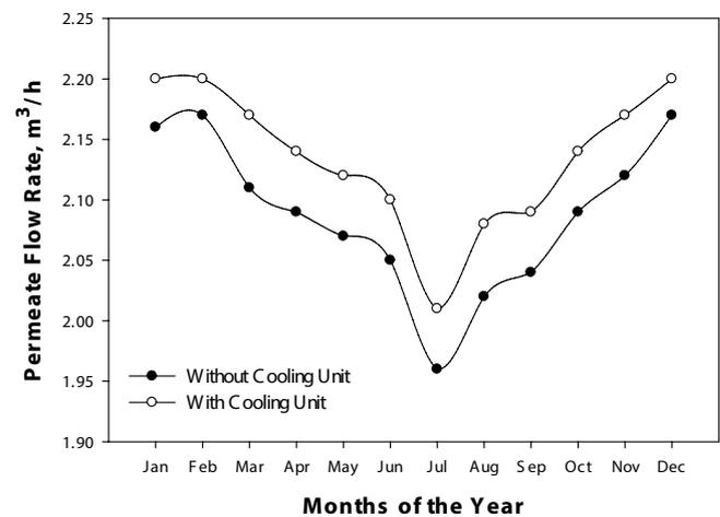
Fig. 9. Variation in monthly permeate flow rate (m<sup>3</sup>/h) of the first desalination line (without cooling unit) and the second desalination line (with cooling unit) for each month of the year.
