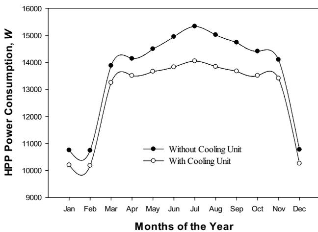
Fig. 8. Variation in monthly HPP power consumption of the first desalination line (without cooling unit) and the second desalination line (with cooling unit) for each month of the year.
