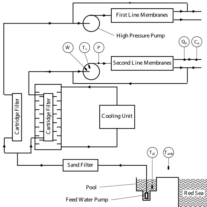
Fig. 1. Schematic of the RO plant coupled first line membranes (without cooling unit) and second-line membranes (with cooling unit) with a cooling unit and instruments.
