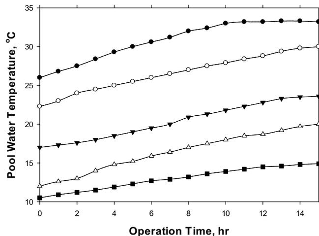
Fig. 5. Variation in pool water temperature vs. operational time of the RO plant for 5 sampling days.
