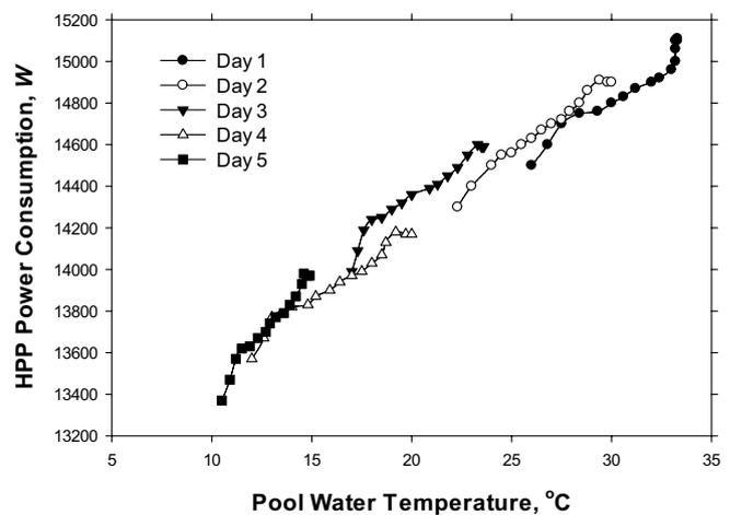
Fig. 3. Variation in power consumption of the HPP vs. brine temperature for the 5 sampling days.
