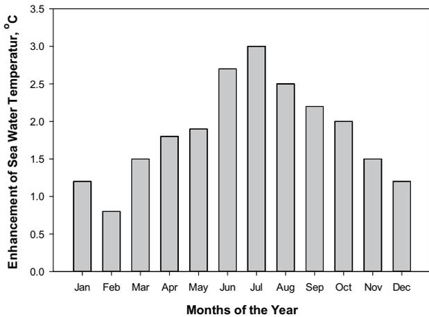
Fig. 6. Average reduction in seawater temperature achieved by using the cooling unit for each month of the year.
