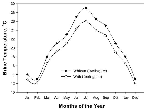
Fig. 7. Variation in monthly brine temperature of first desalination line (without cooling unit) and second desalination line (with cooling unit) for each month of the year.
