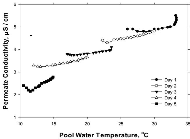
Fig. 4. Variation in permeate conductivity vs. pool water temperature.
