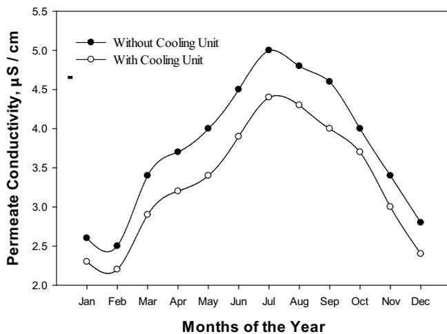
Fig. 10. Variation in monthly permeate conductivity of the first desalination line (without cooling unit) and the second desalination line (with cooling unit) for each months of the year.
