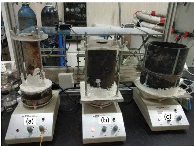
Fig. 2. Simulated pipeline reactor ((a) plastic steel, (b) ductile iron, and (c) PE).
