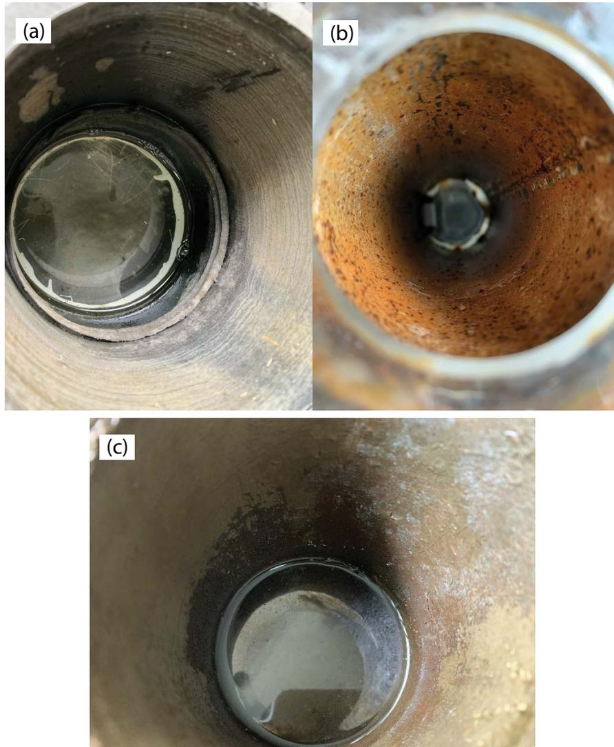
Fig. 1. Pipe wall images (a) PE pipe, (b) plastic steel pipe, and (c) ductile cast iron.
