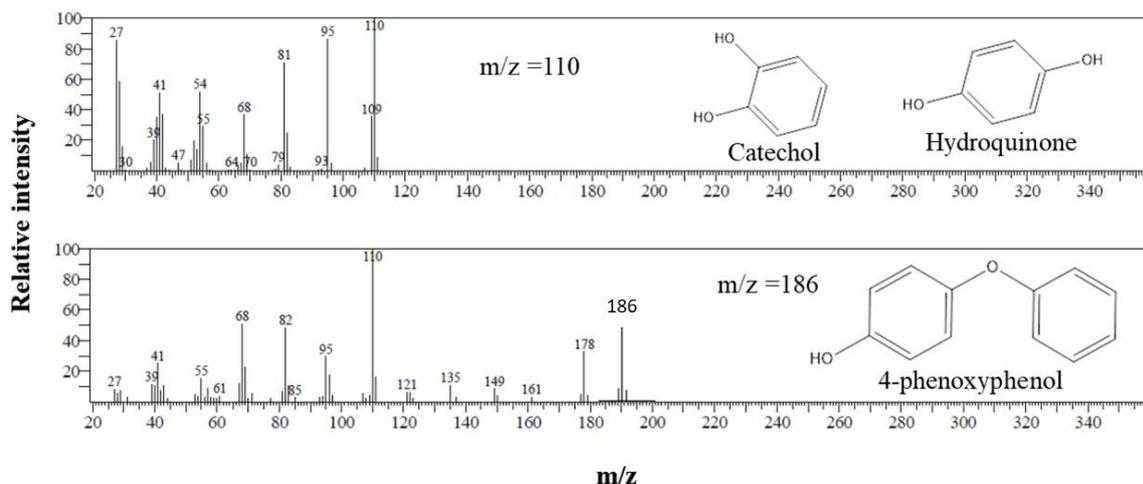
Fig. 3. Possible intermediate compounds of 10 mg L<sup>-1</sup> phenol treated by 500 mg L<sup>-1</sup> PS and 5 mg L<sup>-1</sup> Fe<sup>2+</sup> at 30 min treatment.
