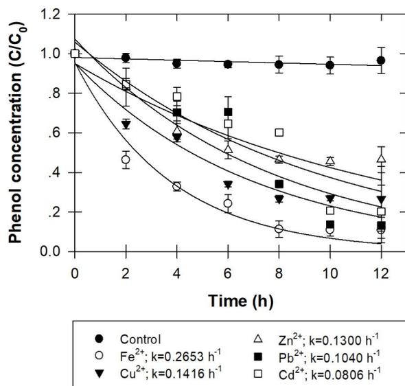
Fig. 1. Phenol ( $10 \text{ mg L}^{-1}$ ) degradation by  $500 \text{ mg L}^{-1}$  persulfate activated by  $5 \text{ mg L}^{-1}$  of various metal ions. The optimal activator was  $\text{Fe}^{2+}$ .
