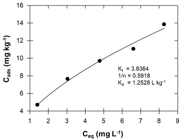
Fig. 6. Adsorption isotherm of phenol at pH 7 on aquifer at equilibrium time (24 h).
