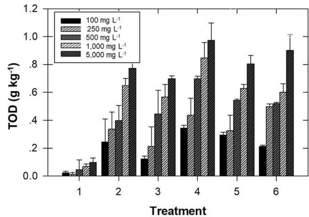
Fig. 5. Total oxygen demand (TOD) of aquifer material applying different PS concentration (100–5,000 mg L<sup>-1</sup>) and treatment conditions (treatment 1: sand + DI, treatment 2: aquifer + DI, treatment 3: sand + groundwater, treatment 4: aquifer + groundwater, treatment 5: aquifer mixed with: sand (50:50) + groundwater, and treatment 6). Aquifer mixed with sand (30:70) + groundwater.
