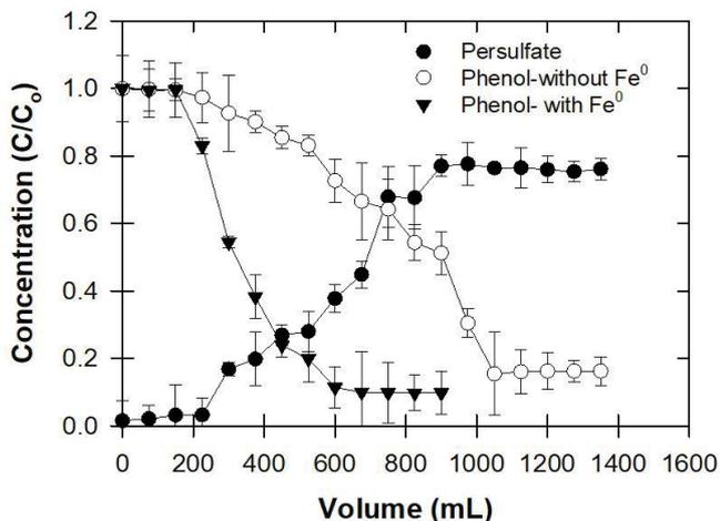
Fig. 7. Breakthrough curves of phenol ( $10 \text{ mg L}^{-1}$ ) at pH 7 and persulfate ( $500 \text{ mg L}^{-1}$ ) through the aquifer column with  $\text{Fe}^0$  (1%, w/w) and without  $\text{Fe}^0$  added. Bars on symbols represent standard deviations; where absent, bars fall within symbols.
