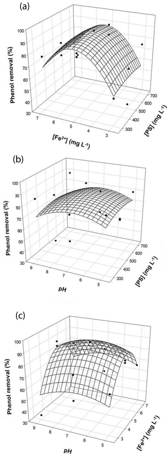
Fig. 4. Response surface plots of treating 10 mg L<sup>-1</sup> phenol in groundwater: (a) PS and Fe<sup>2+</sup>, the optimal condition was 525 mg L<sup>-1</sup> PS and 4.97 mg L<sup>-1</sup> Fe<sup>2+</sup>, (b) PS and pH, the optimal condition was 518 mg L<sup>-1</sup> PS at pH 6.7, and (c) Fe<sup>2+</sup> and pH, the optimal condition was 4.97 mg L<sup>-1</sup> Fe<sup>2+</sup> at pH 6.5.
