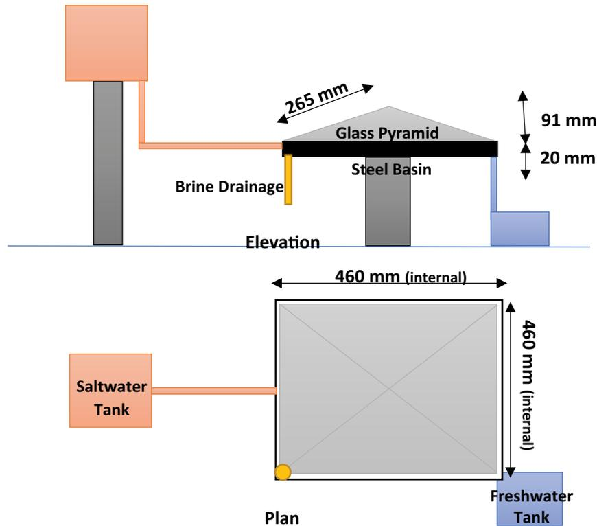
Fig. 1. Schematic for a desalination unit working by direct solar energy.
