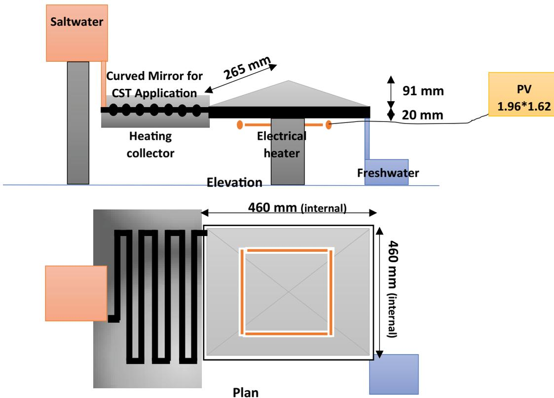
Fig. 8. Final design of the desalination unit with a hybrid system with both direct and indirect solar energy applications.
