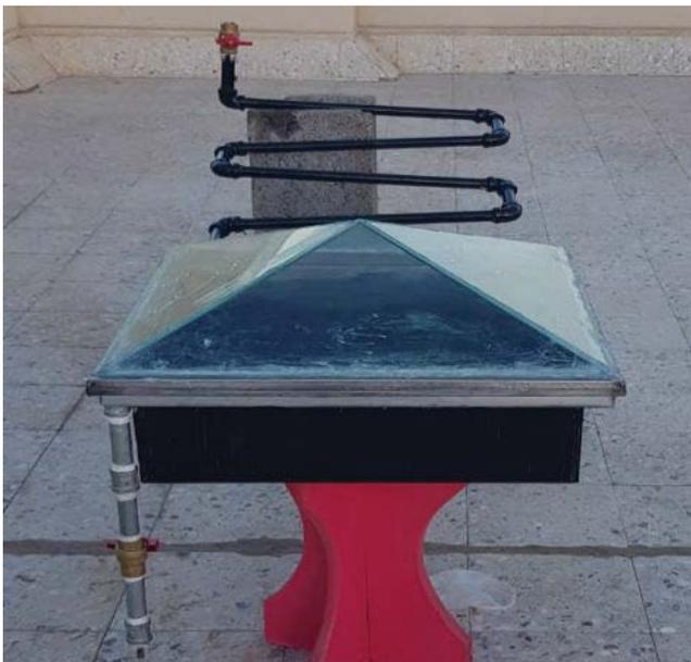
Fig. 5. A picture for setting heating collector in the prototype.
