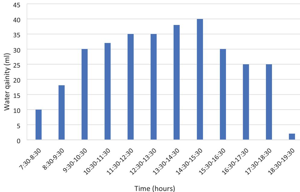
Fig. 4. Fresh water quantity generated by the control experiment (only the impact of direct solar heating).
