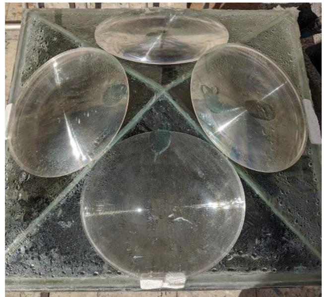
Fig. 6. A picture for setting four lenses above the pyramid glass of the prototype.
