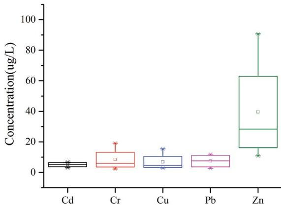
Fig. 6. Concentration of heavy metals in influent of sewage treatment plants.
