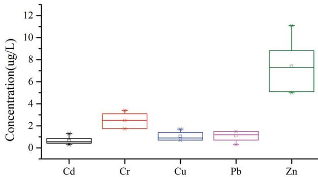
Fig. 2. Average concentration of heavy metals in surface water of Wenyu River.
