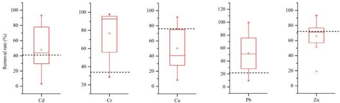
Fig. 8. Removal rate of heavy metals in Beijing and the reviewed Sewage Treatment Plants. The box plots indicated the removal rate of heavy metals in the reviewed Sewage Treatment Plants; the dash lines indicated average values of Sewage Treatment Plants in this study.
