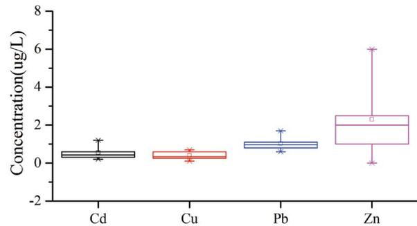
Fig. 4. Average concentration of heavy metals in groundwater of Beijing.
