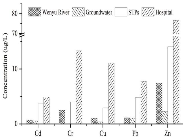
Fig. 9. Concentration of heavy metals in multiple water bodies of Beijing.
