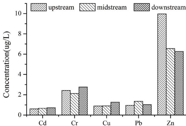
Fig. 3. Spatial distribution of heavy metals in surface water of Wenyu River.
