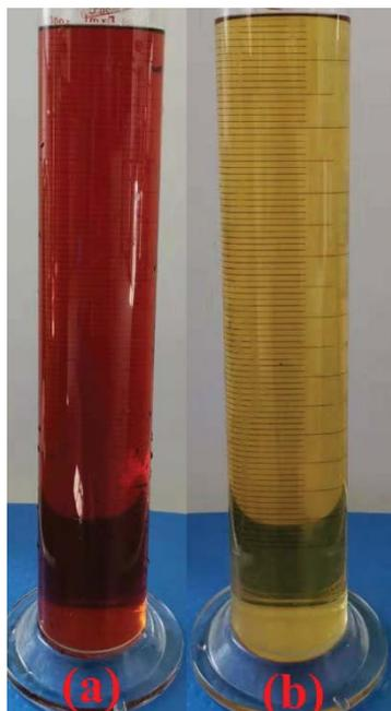
Fig. 7. Color change of wastewater (a) before and (b) after catalytic ozone oxidation treatment.
