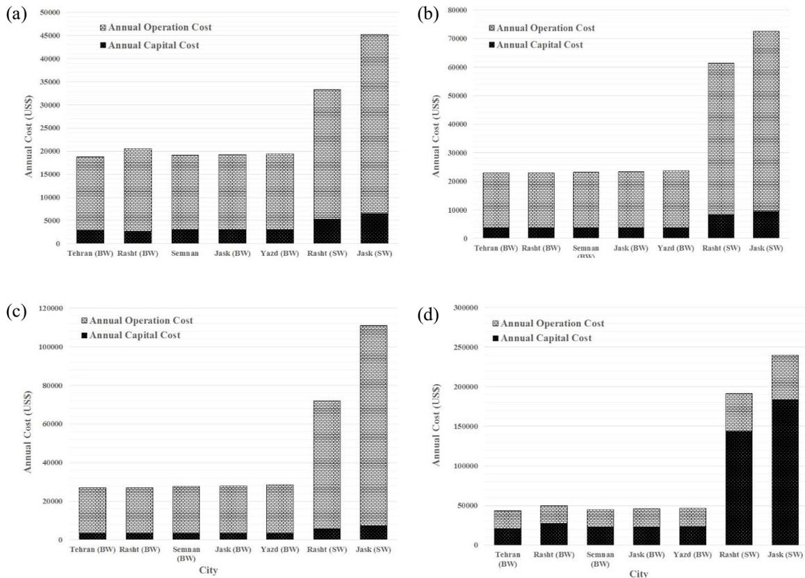
Fig. 8. Ratio of the annualized capital cost of system vs. its annualized operating and flow costs in different scenarios. Input energy from (a) grid power, (b) gas engine, (c) diesel engine, and (d) solar PV.
