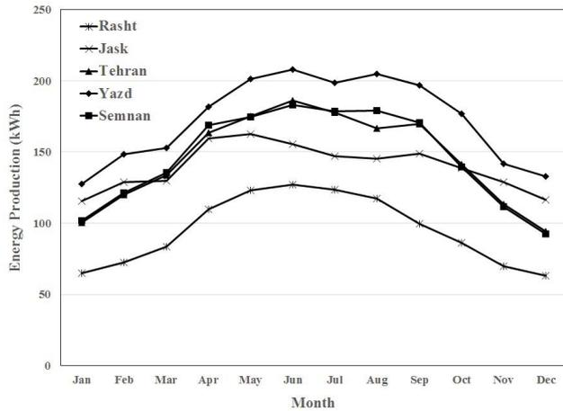
Fig. 5. Monthly energy production from 1 kW solar PV panels and in selected cities.
