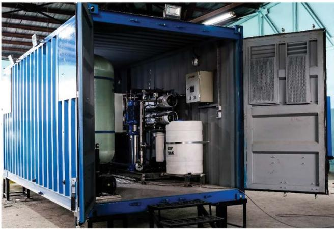
Fig. 1. Constructed brackish water RO unit which is developed as a pilot for this study.
