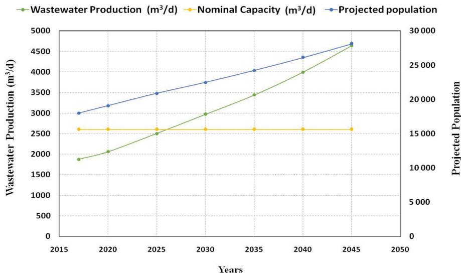
Fig. 14. Wastewater production according to population growth in different horizons (with the discharge of AbdAlmalek Locality).
