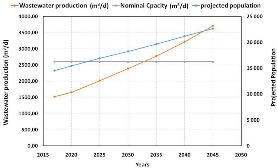
Fig. 12. Wastewater production evolution according to the population growth (taking into account the connection of Safsaf Locality).
