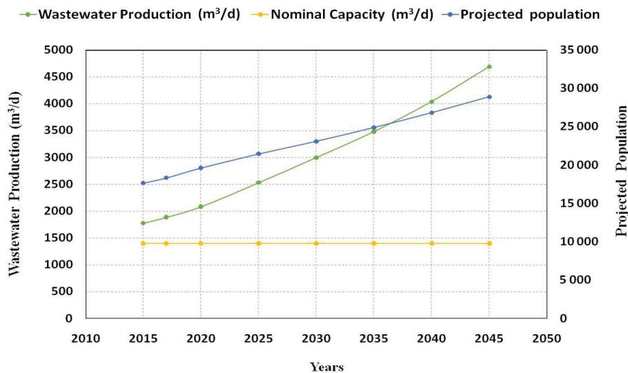
Fig. 15. Wastewater production according to population growth in the different horizons.
