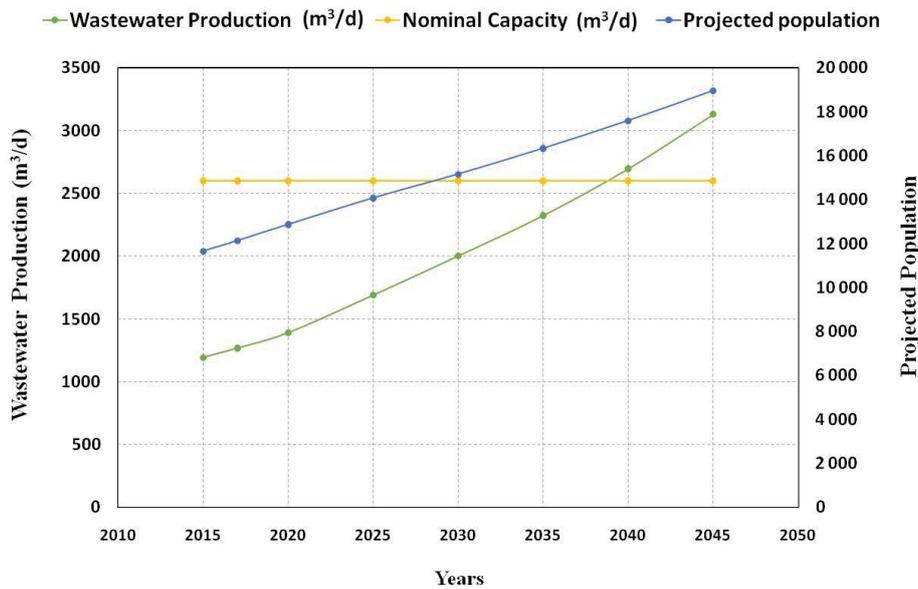
Fig. 13. Wastewater production as a function of population growth in different horizons.
