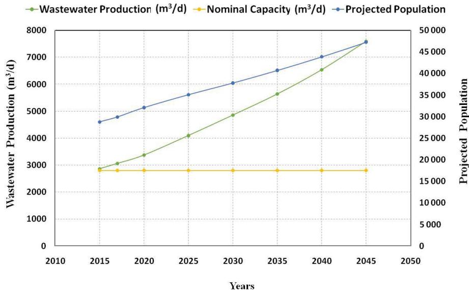
Fig. 7. Production of wastewater according to the projection of the population in the different horizons (with the rejection of Mansourah-Bled Touahriya-Sirat).
