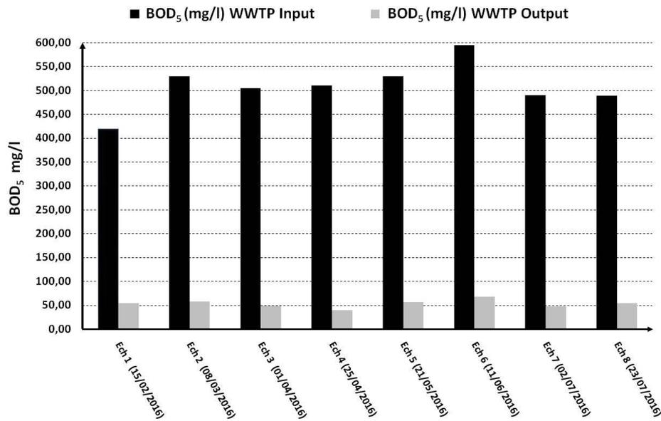
Fig. 8. Characteristics of wastewater samples in terms of BOD<sub>5</sub>.
