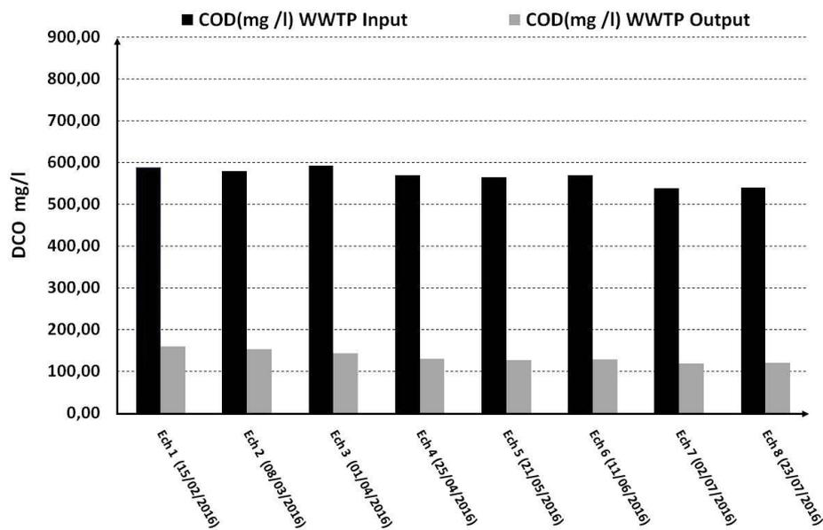
Fig. 9. Characteristics of wastewater samples in terms of COD.
