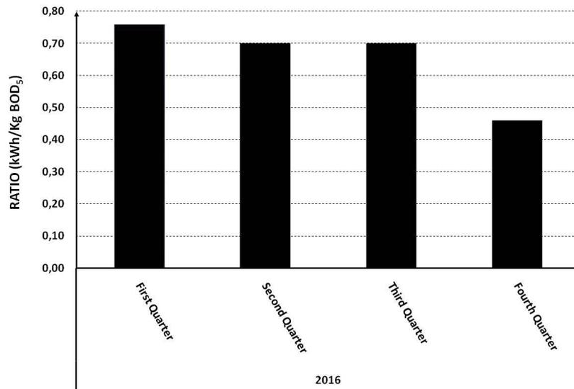
Fig. 5. Estimated KWh/ratio (Kg BOD<sub>5</sub> eliminated).
