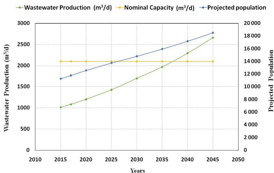
Fig. 10. Wastewater production as a function of population projection in different horizons.
