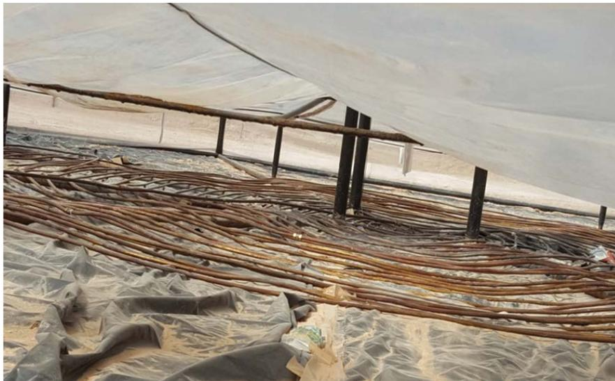
Fig. 8. Copper coil installed inside the solar chimney collector.
