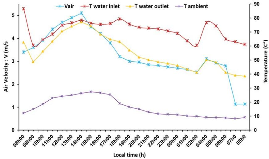
Fig. 12. Variation of air velocity, water temperature inlet and outlet in the solar chimney at night vs. local time 27th and 28th of February 2017, with water heater integration.
