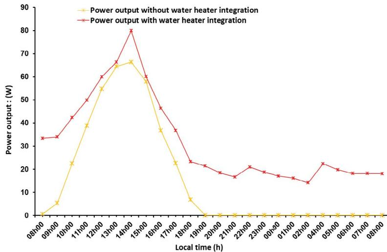
Fig. 14. Variation of power output of the solar chimney power plant with and without water heater integration.
