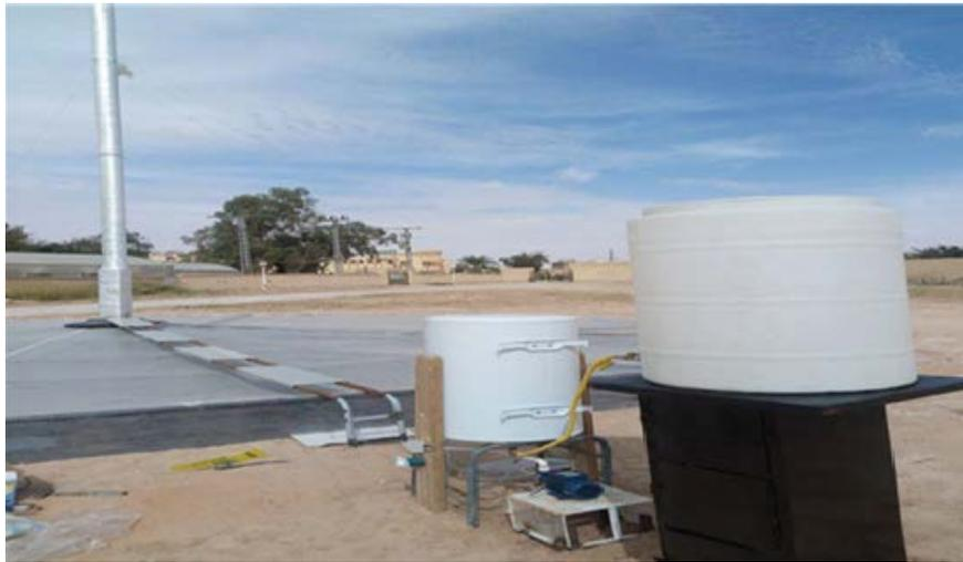
Fig. 7. Electrical water heater integrated with solar chimney power plant.
