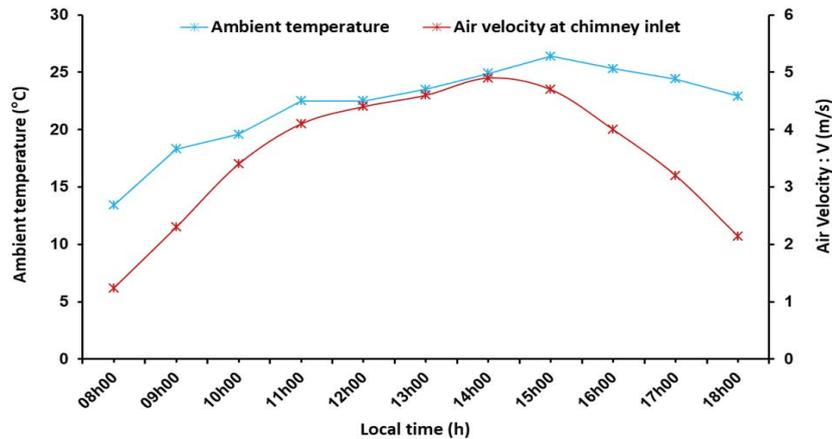
Fig. 10. Measured ambient temperature and air velocity vs. local time on 8th of February 2017, without water heater integration.
