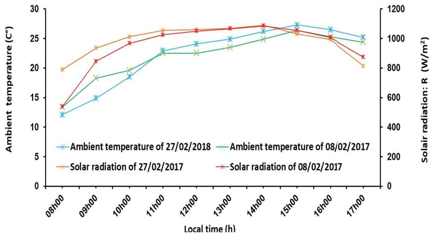
Fig. 13. Meteorological parameters of the days of 8th and 27th February 2017.
