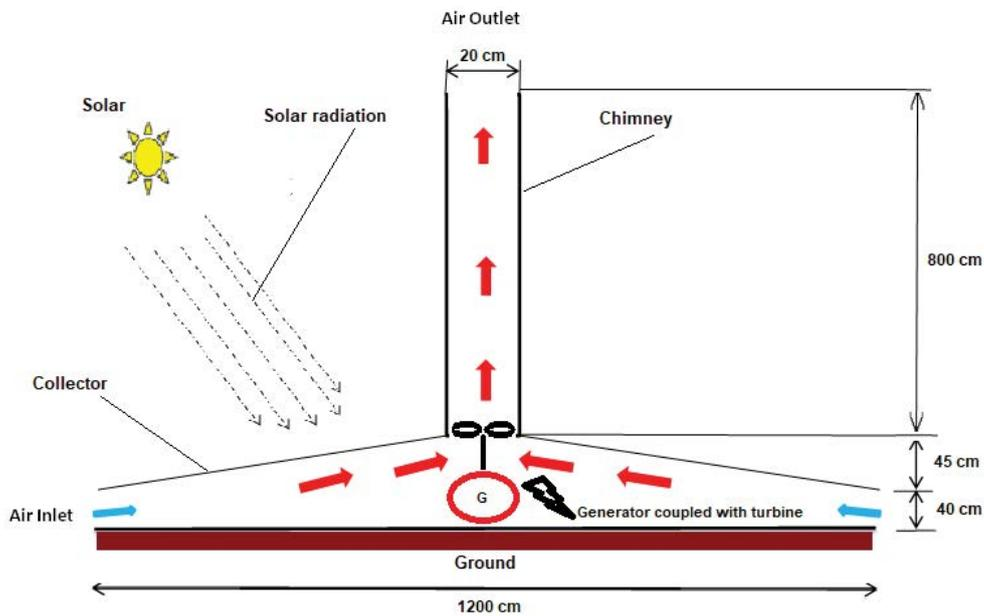
Fig. 3. Prototype solar chimney power plant schematic layout.
