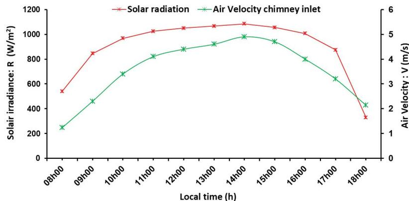
Fig. 9. Measured solar irradiance and air velocity vs. local time on 8th of February 2017, without water heater integration.
