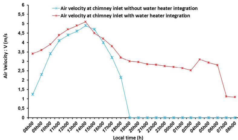
Fig. 11. Temporal variation of air velocity at the chimney inlet with and without water heater integration.
