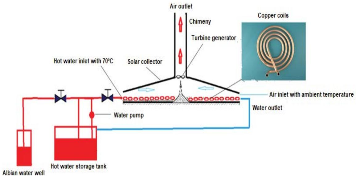
Fig. 2. Schematic layout of the proposed solar chimney power plant integrated with geothermal source (Albian water).
