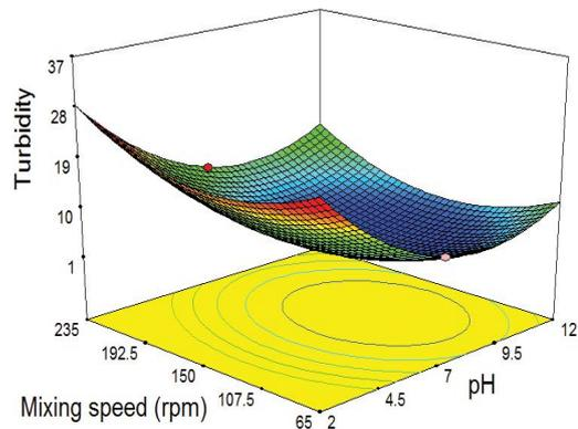
Fig. 9. Effect of mixing speed and pH on turbidity removal.
