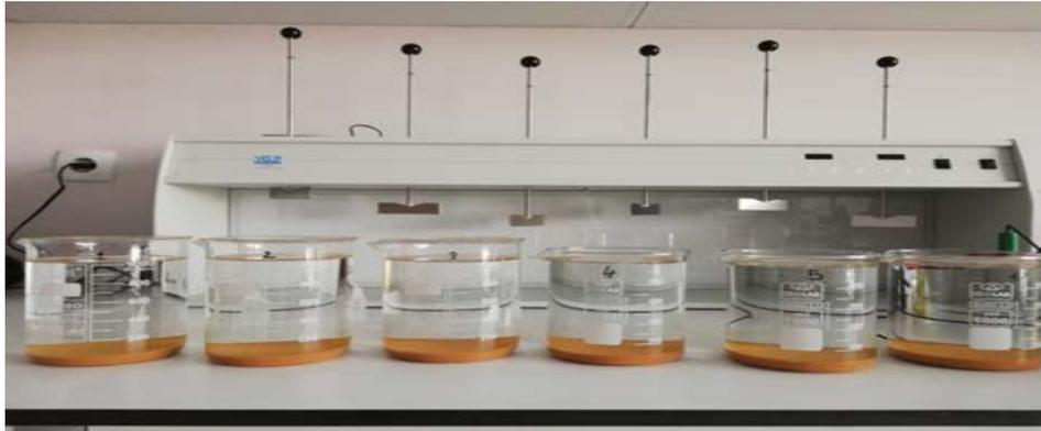
Fig. 1. Jar test set-up used in wastewater treatment.
