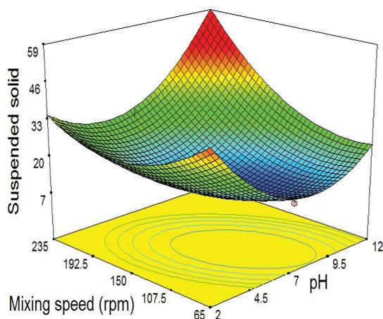
Fig. 12. Effect of mixing speed and pH on TSS removal.
