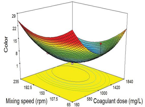
Fig. 7. Effect of mixing speed and coagulant dose on color removal.
