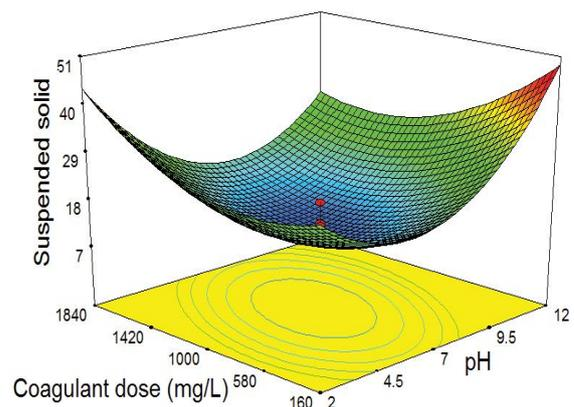
Fig. 11. Effect of coagulant dose and pH on TSS removal.
