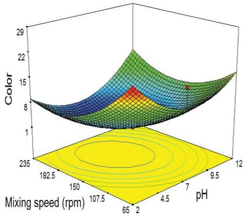
Fig. 6. Effect of mixing speed and pH on color removal.
