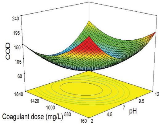
Fig. 2. Effect of coagulant dose and pH on COD removal.
