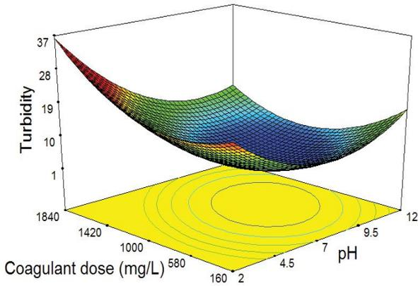
Fig. 8. Effect of coagulant dose and pH on turbidity removal.
