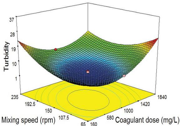
Fig. 10. Effect of coagulant dose and mixing speed on turbidity removal.
