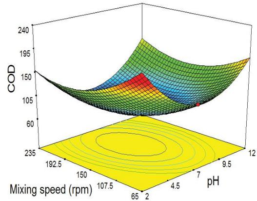
Fig. 3. Effect of mixing speed and pH on COD removal.
