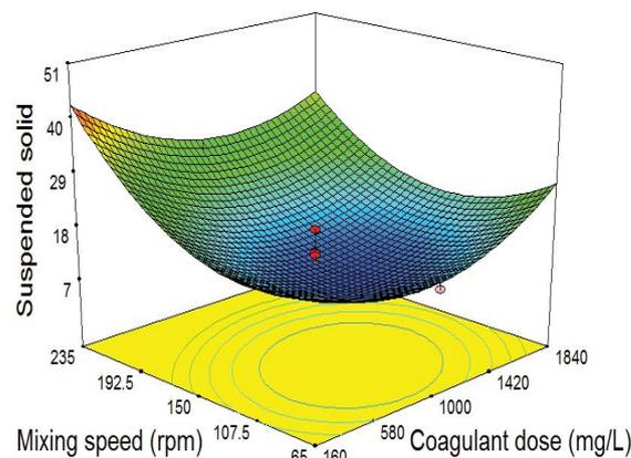
Fig. 13. Effect of coagulant dose and mixing speed on TSS removal.
