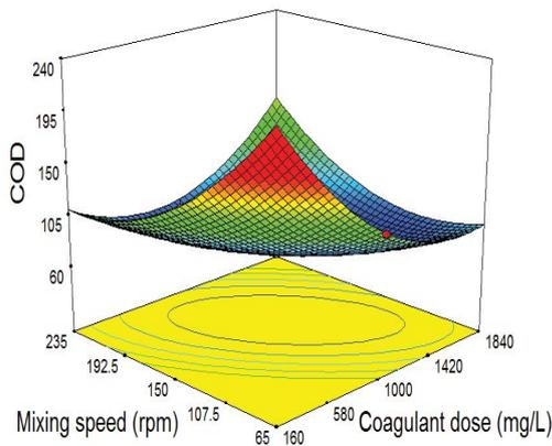
Fig. 4. Effect of mixing speed and coagulant dose on COD removal.
