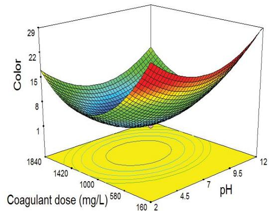
Fig. 5. Effect of coagulant dose and pH on color removal.
