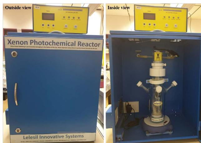
Fig. 2. Setup of photo-reactor for dye degradation.
