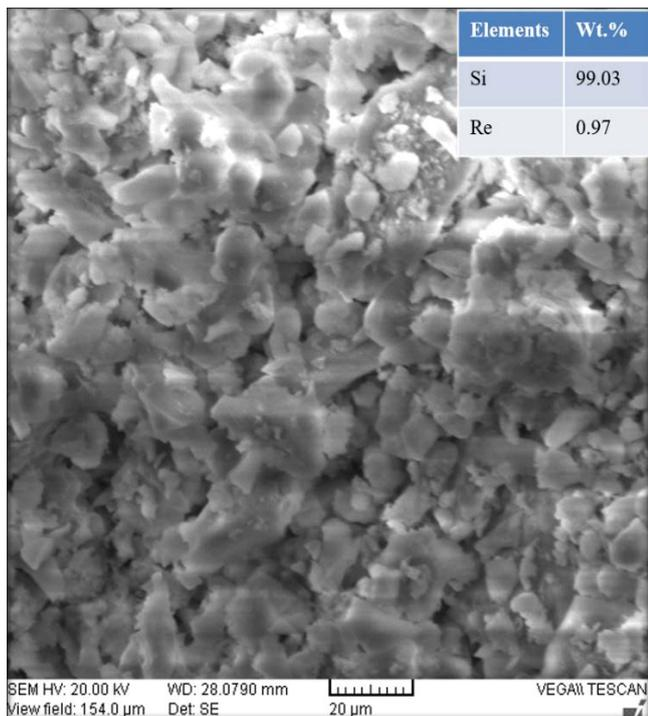
Fig. 5. SEM micrographs of Si<sub>0.9</sub>Re<sub>0.1</sub>O<sub>2</sub> photo-catalyst.
