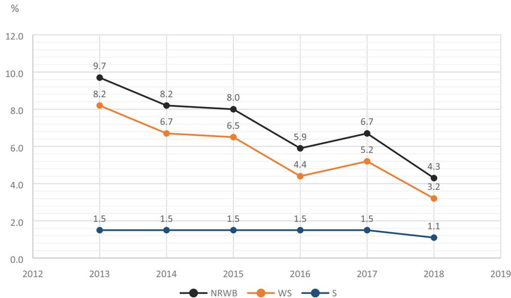
Fig. 2. Percentage water loss index (WS), non-revenue water basic index (NRWB), and percentage water used for own needs of the company (S) – company B.
