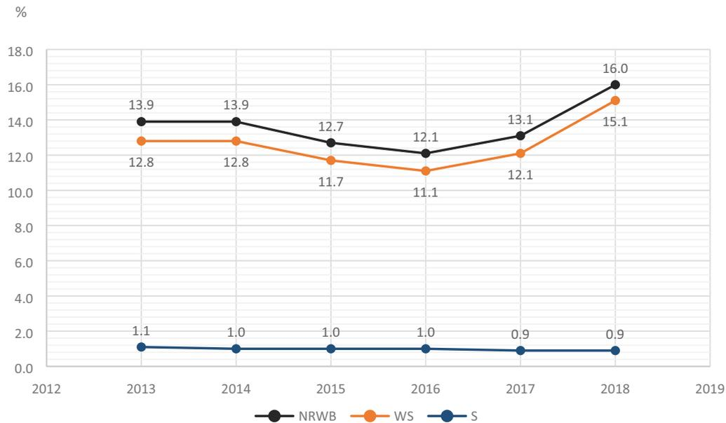
Fig. 1. Percentage water loss index (WS), non-revenue water basic index (NRWB), and percentage water used for own needs of the company (S) – company A.
