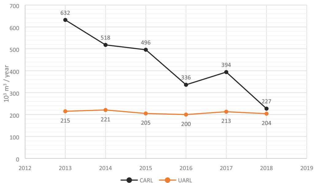
Fig. 4. Unavoidable losses in relation to total losses in the years 2013–2018 (system B).
