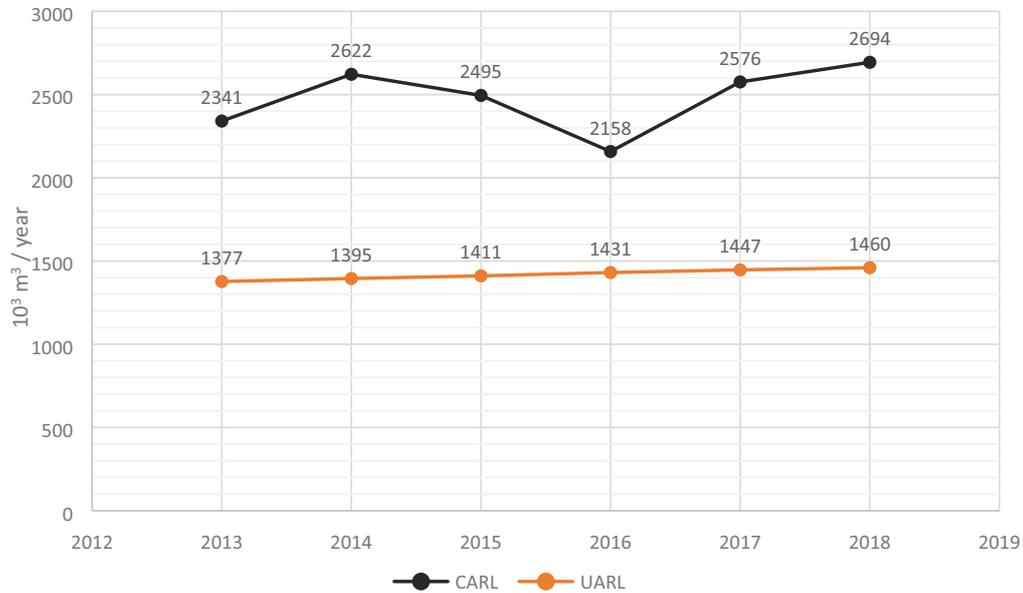
Fig. 3. Unavoidable losses in relation to total losses in the years 2013–2018 (company A).
