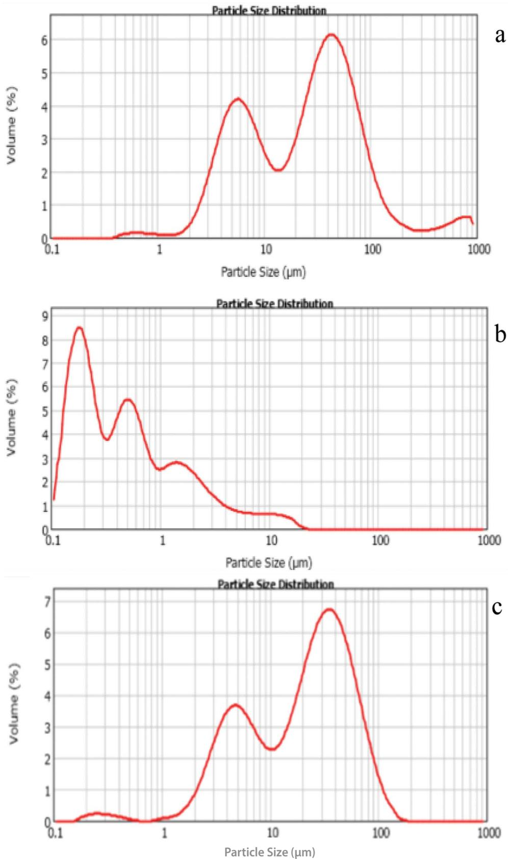
Fig. 2. Particle size distribution of microalgae inoculum (a), anaerobic digestate (b), and mixed microalgae (c) grown in 10% anaerobic digestate (last day of cultivation).
