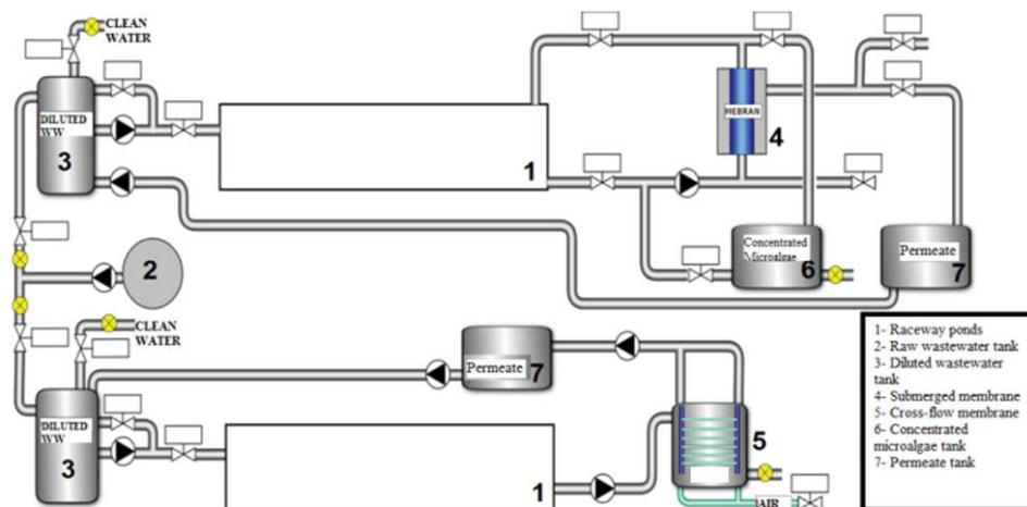
Fig. 1. Automation system of membrane systems (1) raceway pond, (2) raw wastewater tank, (3) diluted wastewater tank, (4) submerged membrane, (5) cross-flow membrane, (6) concentrated microalgae tank, and (7) permeate tank.
