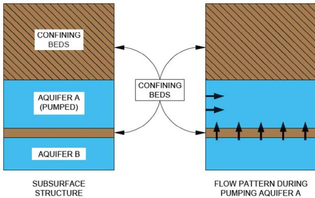
Fig. 11. Diagram of the upward recharge flow pattern of a brackish-water aquifer during pumping [3].
