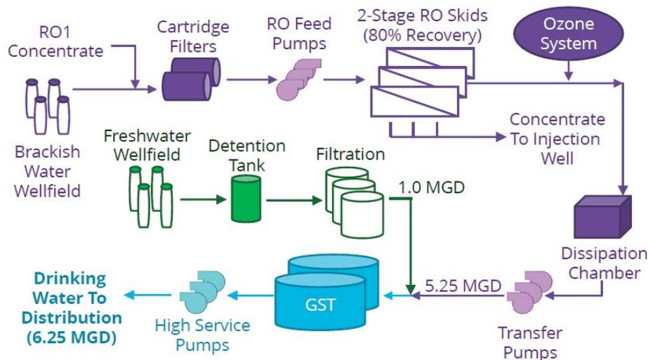
Fig. 2. Process flow diagram for the City of Clearwater BWRO water treatment facility [10].
