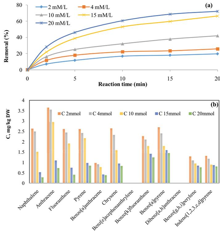
Fig. 2. (a) Effect of concentration of sodium persulfate on degradation efficiency of PAH compounds and (b) residuals of PAH compounds affected by primary concentration of persulfate in AOPs process ( $C_{\text{PAHs}} = 28.3 \text{ mg/kg dw}$ ,  $T = 25^\circ\text{C}$ , and  $\text{pH} = 11$ ).
