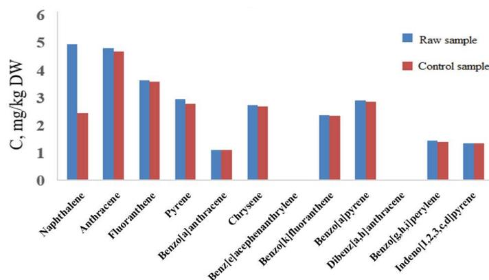
Fig. 5. PAHs changes in the control sludge after 20 d in comparison to raw sludge.
