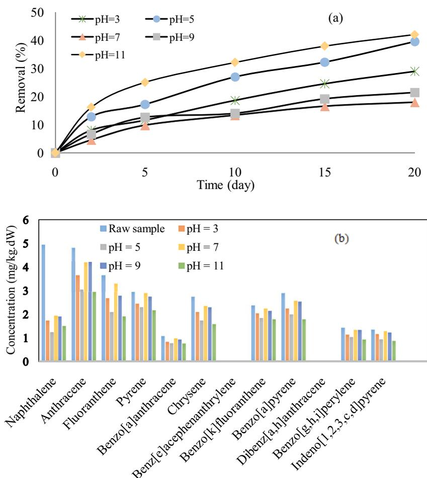
Fig. 1. (a) Effect of pH on the efficiency of PAH compounds degradation and (b) residuals of PAH compounds affected by different pH in AOPs process ( $C_{\text{persulfate}} = 10 \text{ mM/L}$ ,  $C_{\text{PAHs}} = 28.3 \text{ mg/kg dw}$ , and  $T = 25^\circ\text{C}$ ).
