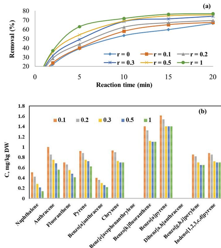
Fig. 3. (a) Effect of the ratio of peroxide to persulfate on PAH compounds degradation efficiency and (b) residuals of PAH compounds affected by various ratios of peroxide to persulfate in AOPs process ( $C_{\text{persulfate}} = 15 \text{ mmol/L}$ ,  $C_{\text{PAHs}} = 28.3 \text{ mg/kg dw}$ ,  $T = 25^\circ\text{C}$ , and  $\text{pH} = 11$ ).
