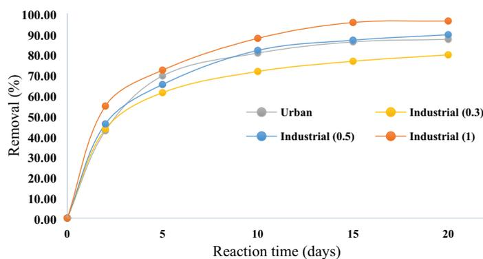
Fig. 6. Effect of PAH compounds concentration on AOPs process efficiency ( $C_{\text{persulfate}} = 15 \text{ mmol/L}$ ,  $C_{\text{PAHs}} = 143.45 \text{ mg/kg dw}$ ,  $T = 45^\circ\text{C}$ , and  $\text{pH} = 11$ ).
