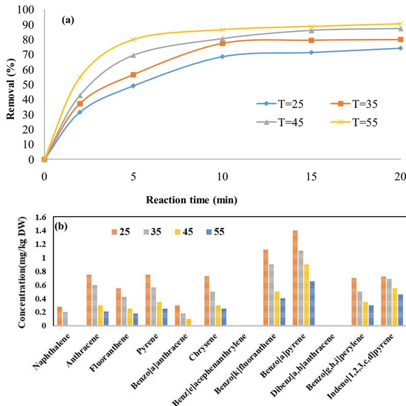
Fig. 4. (a) Effect of reaction temperature on efficiency of AOPs process in PAH compounds degradation efficiency and (b) residuals of PAH compounds affected by various temperatures in AOPs process ( $C_{\text{persulfate}} = 15$  mmol/L,  $C_{\text{PAHs}} = 28.3$  mg/kg dw, ratio<sub>peroxide/persulfate</sub> = 0.3, pH = 11, and time = 20 d).
