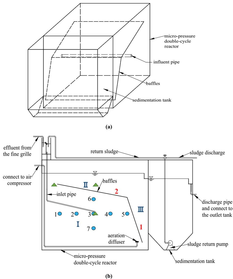
Fig. 3. (a) Three-dimensional schematic diagram of pilot test device and (b) schematic diagram of technological process and distribution of test points of pilot test device.
