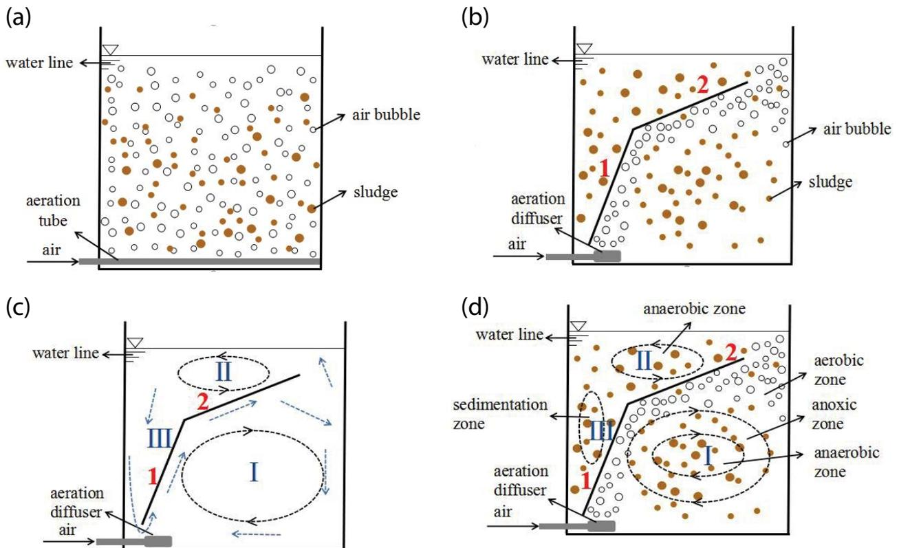
Fig. 1. (a) Schematic diagram of traditional biological aeration tank, (b) schematic diagram of MPDR biological aeration tank, (c) schematic diagram of MPDR mixed liquid flow distribution in ideal state, and (d) schematic diagram of MPDR different dissolved oxygen zones in ideal state.
