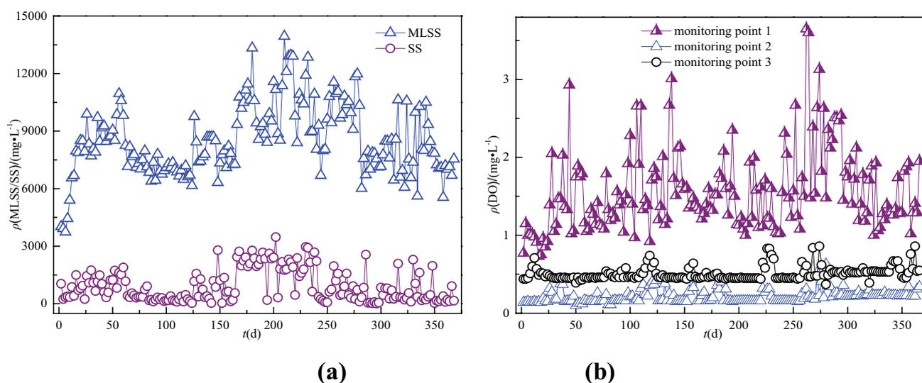
Fig. 6. (a) Changes in average MLSS concentration in the reactor and changes in SS concentration in the influent during the test and (b) changes in DO during the test period at three DO monitoring points.
