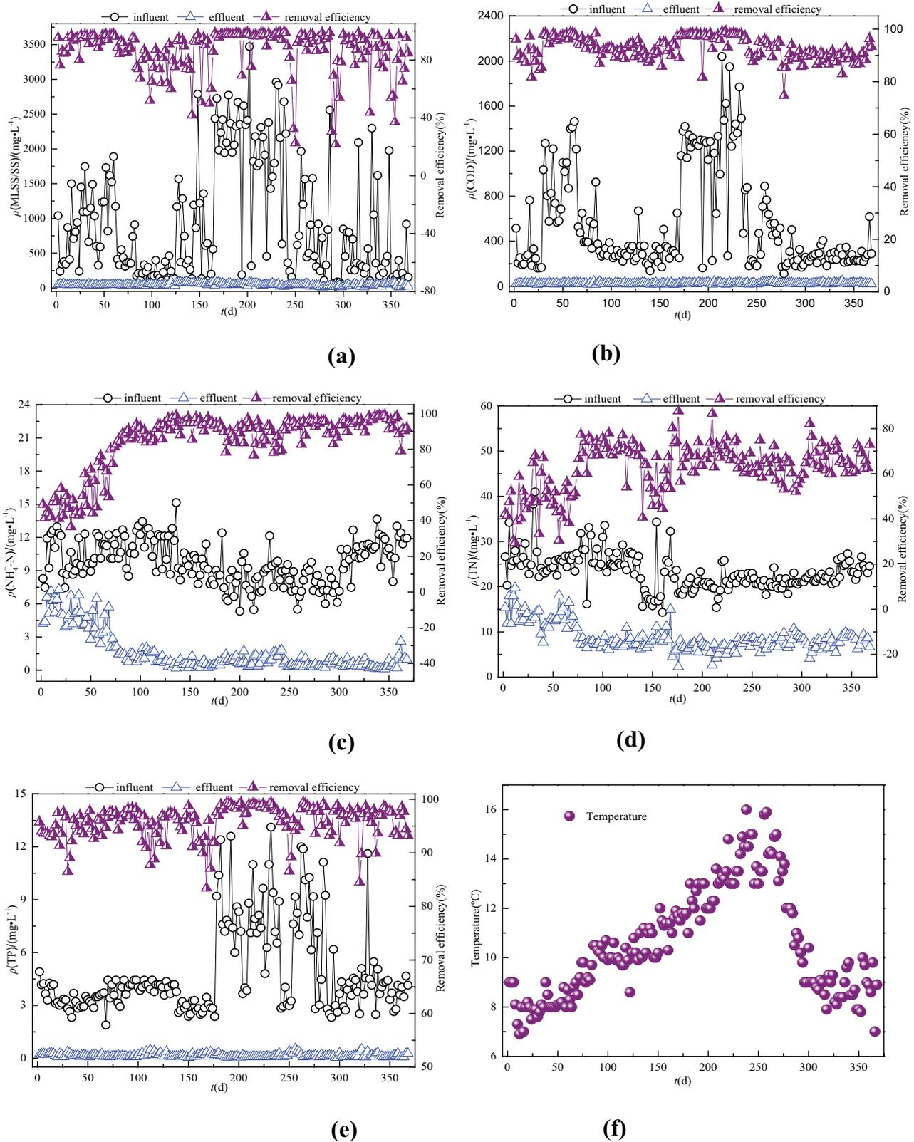
Fig. 5. (a) SS removal effect of pilot test device, (b) COD removal effect of pilot test device, (c)  $\text{NH}_4^+\text{-N}$  removal effect of pilot test device, (d) TN removal effect of the pilot test device, (e) TP removal effect of the pilot test device, and (f) influent temperature change during the test.
