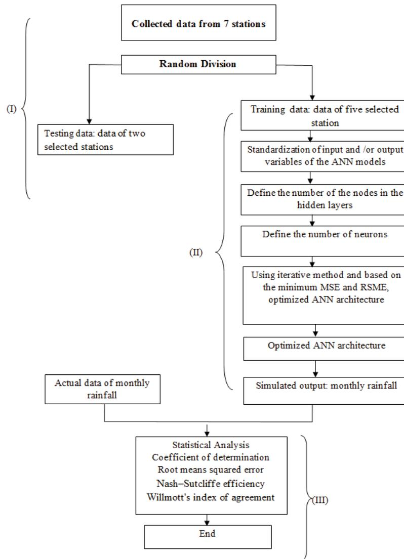
Fig. 3. Flowchart of the ANN-based method prediction procedure.
