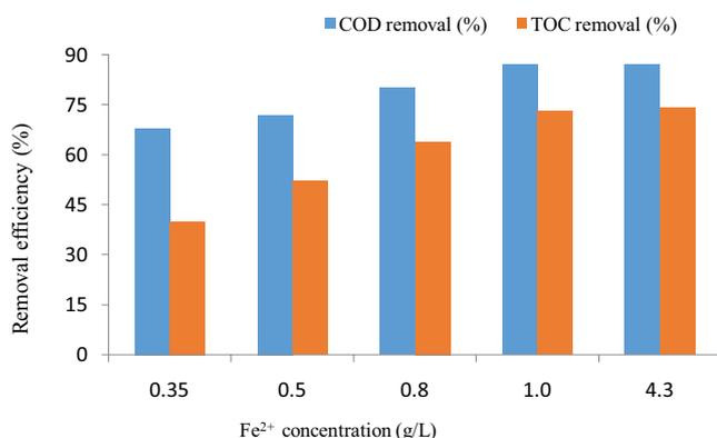
Fig. 2. Effects of different  $\text{Fe}^{2+}$  doses on COD and TOC removal efficiencies ( $\text{pH} = 3$ ;  $\text{H}_2\text{O}_2 = 3.5$  g/L;  $T = 25^\circ\text{C}$ ).
