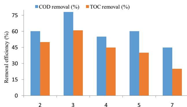
Fig. 3. Effects of different pH values on COD and TOC removal efficiencies ( $\text{H}_2\text{O}_2 = 1.5$  g/L;  $\text{Fe}^{2+} = 1.5$  g/L;  $T = 25^\circ\text{C}$ ).
