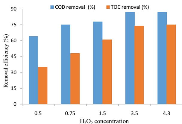
Fig. 1. Effects of different  $\text{H}_2\text{O}_2$  doses on COD and TOC removal efficiencies ( $\text{pH} = 3$ ;  $\text{Fe}^{2+} = 1$  g/L;  $T = 25^\circ\text{C}$ ).
