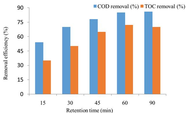
Fig. 4. Effects of reaction time on COD and TOC removal efficiencies ( $H_2O_2 = 1.5 \text{ g/L}$ ;  $Fe^{2+} = 1.5 \text{ g/L}$ ;  $T = 25^\circ\text{C}$ ).
