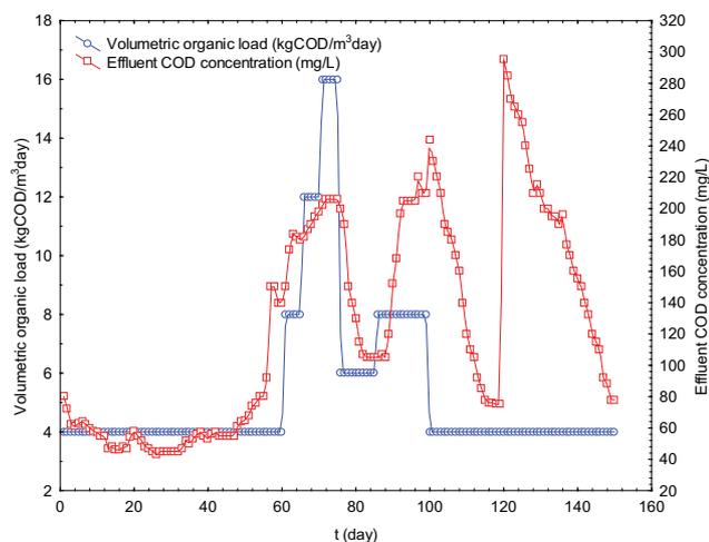
Fig. 8. Change in different volumetric organic loadings over time.
