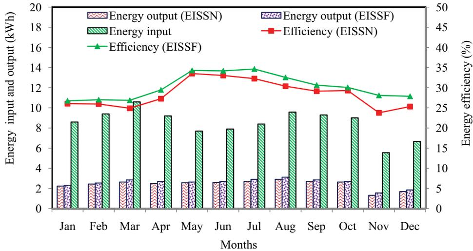
Fig. 6. Comparative daily energy input/output and energy efficiencies of ESSN and EISSF.
