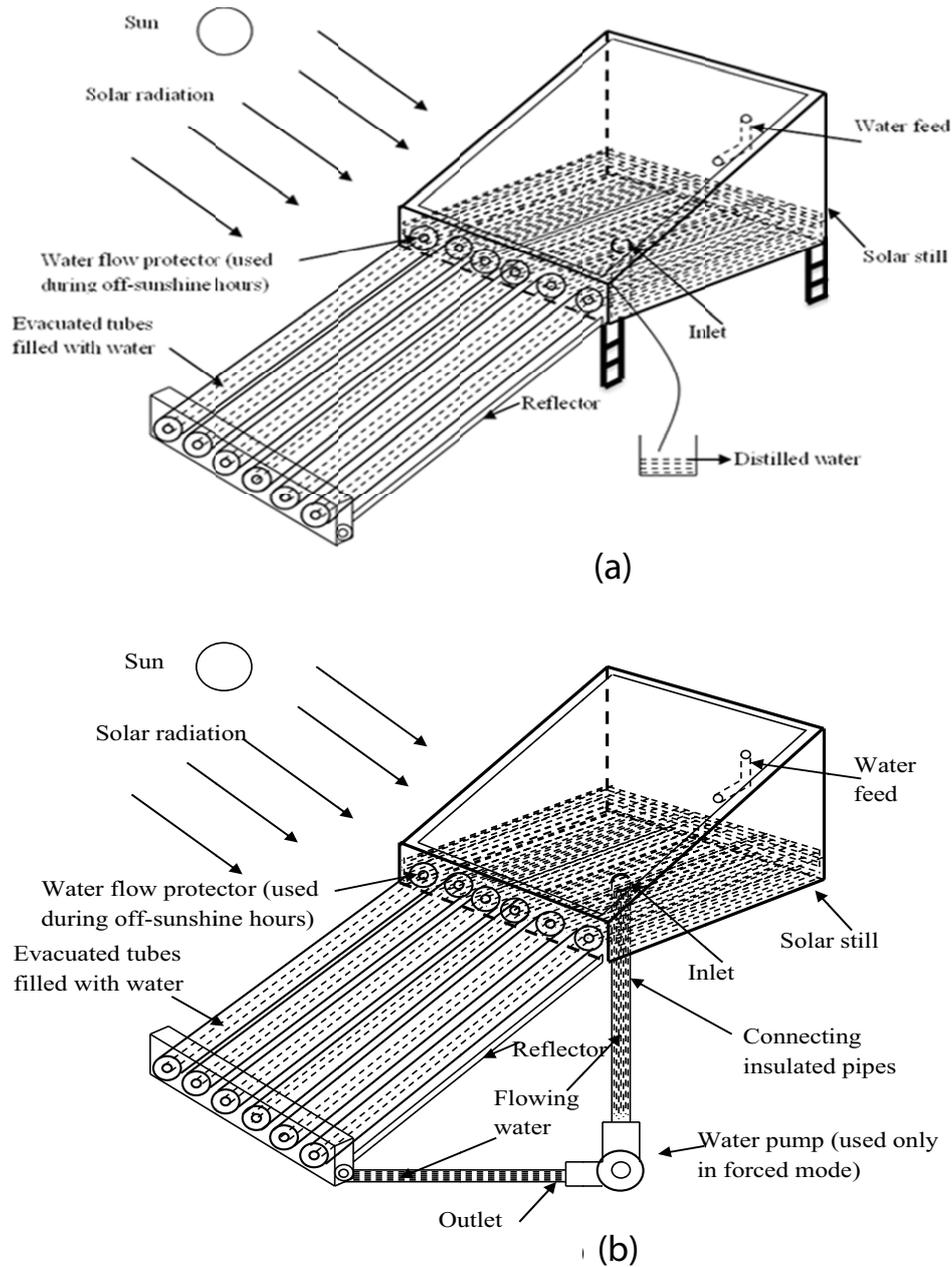
Fig. 1. Schematic of (a) EISSN and (b) EISSF solar still.
