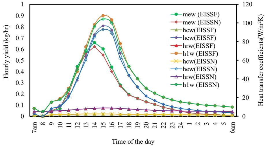
Fig. 3. Variation of yield and heat transfer coefficients from EISSN and EISSF.
