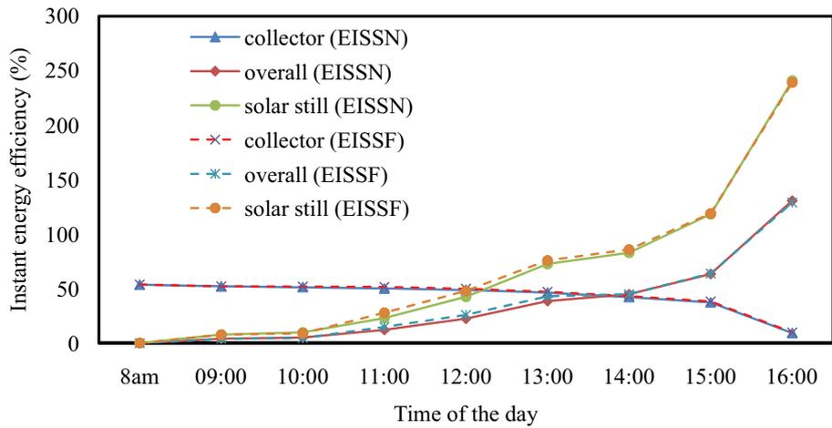
Fig. 4. Variation of instant energy efficiency of EISSN and EISSF.
