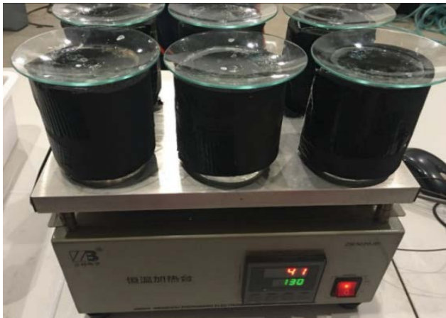
Fig. 2. Brine scaling test bench picture.
