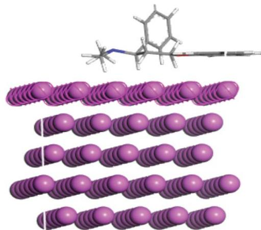
Fig. 11. Adsorption configuration at equilibrium of dapoxetine on Al(111) obtained by molecular dynamic simulation.
