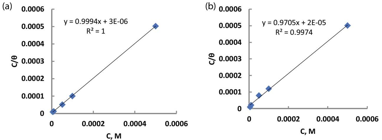
Fig. 7. Langmuir adsorption isotherm for AA6063 in (a) 1.0 M HCl and (b) 1.0 M NaOH solutions containing different concentrations of dapoxetine.
