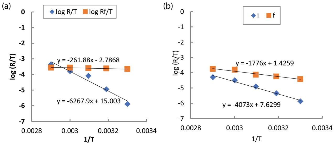
Fig. 5. Transition state plot for the corrosion of AA6063 in the free (a) 1.0 M HCl and (b) 1.0 M NaOH solutions and in the presence of 0.0005 M of dapoxetine.
