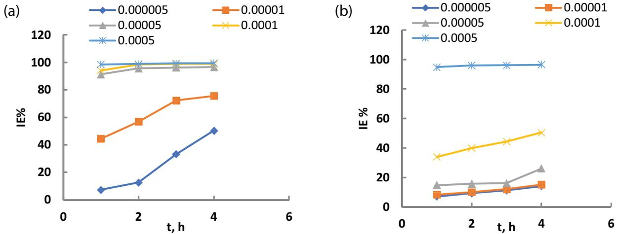
Fig. 3. Impact of immersion time on the IE% of dapoxetine for corrosion of AA6063 in (a) 1.0 M HCl and (b) 1.0 M NaOH solutions.
