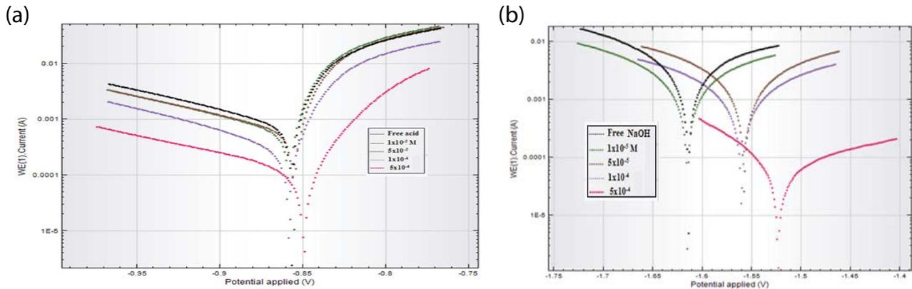
Fig. 6. PDP curves of AA6063 in free (a) 1.0 M HCl solution and (b) 1.0 M NaOH solution and containing different concentrations of dapoxetine.
