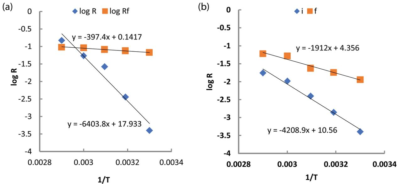
Fig. 4. Arrhenius plot for the corrosion of AA6063 in the free (a) 1.0 M HCl and (b) 1.0 M NaOH solutions and in the presence of 0.0005 M of dapoxetine.
