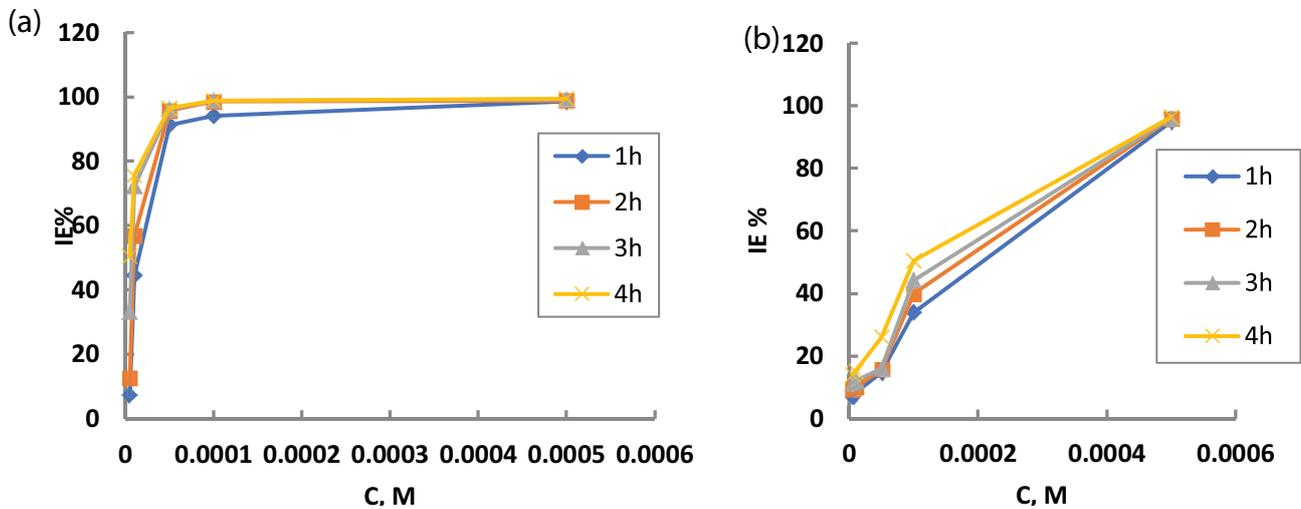
Fig. 2. Effect of various concentrations of dapoxetine on the IE% for AA6063 corrosion in (a) 1.0 M HCl and (b) 1.0 M NaOH solutions.
