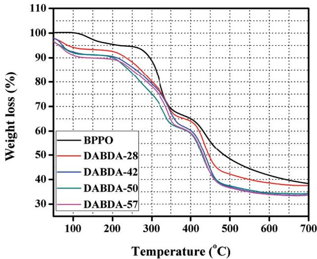
Fig. 4. TGA curves of pristine BPPO and prepared membranes.
