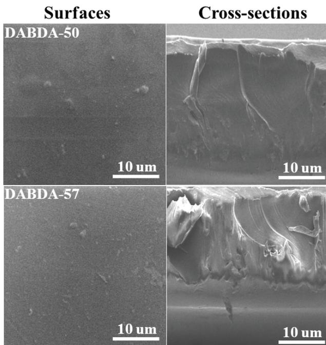
Fig. 5. SEM micrographs of surfaces and cross-sections of the prepared membranes DABDA-50 and DABDA-57 representing the homogeneous morphology.
