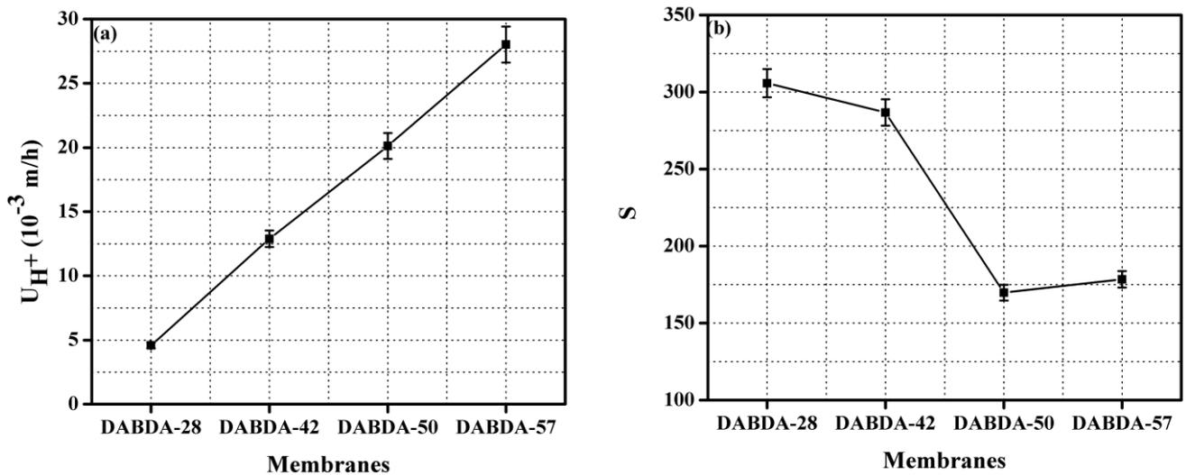
Fig. 7. (a) Diffusion dialysis coefficient of acid ( $U_{H^+}$ ) and (b) separation factor (S) of the prepared anion exchange membranes at 25°C.
