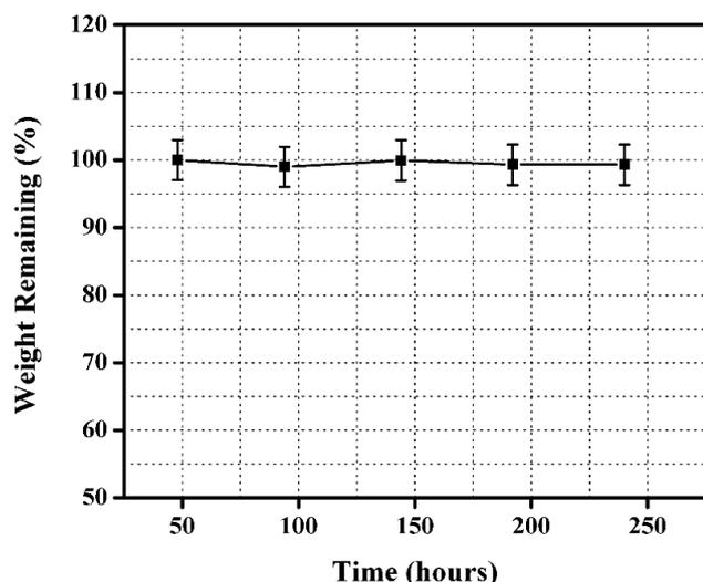
Fig. 6. Weight remaining of the prepared membrane DABDA-57 after immersion in HCl/FeCl<sub>2</sub> feed solution for 240 h at 60°C.
