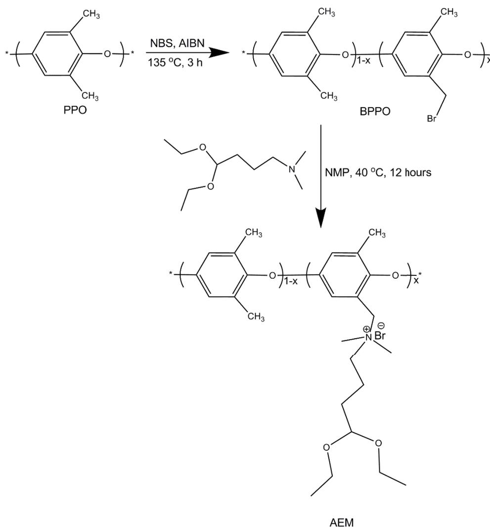
Fig. 1. Preparation of BPPO-based anion exchanged membranes.
