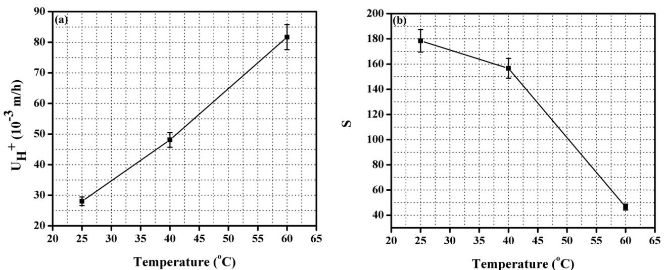
Fig. 8. (a) Diffusion dialysis coefficient of acid ( $U_{H^+}$ ), (b) separation factor (S) of the prepared anion exchange membranes at different temperature.
