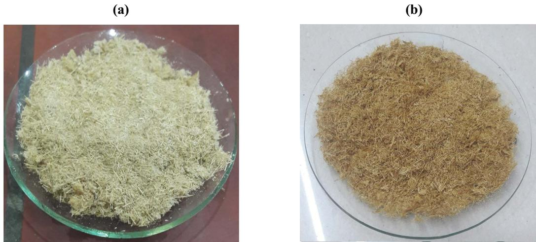
Fig. 1. Images of sugarcane bagasse (a) before and (b) after modification.
