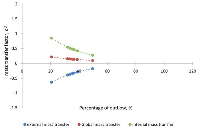
Fig. 7. Global, internal, and external mass transfer factor vs. percentage of outflow for the adsorption of OM (COD) onto BCF.
