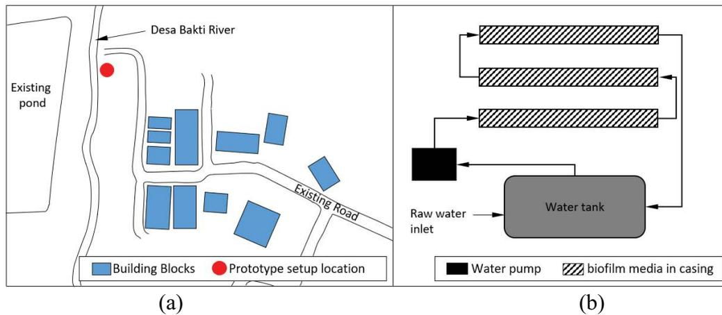
Fig. 1. Illustration showing (a) the location of the prototype setup and (b) the details of the fabricated column model.
