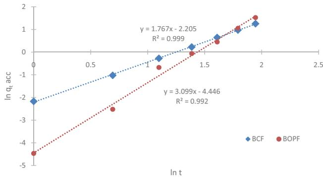
Fig. 6. Plot of  $\ln q_t, \text{acc}$  vs.  $\ln t$  for the mass accumulation of OM onto BCF and BOPF.
