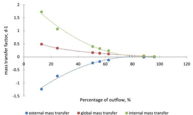
Fig. 8. Global, internal, and external mass transfer factor vs. percentage of outflow for the adsorption of OM (COD) onto BOPF.
