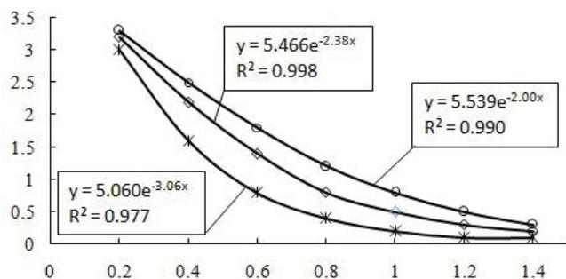
Fig. 3. Removal efficiencies of TP by different phosphorus removal agents.
