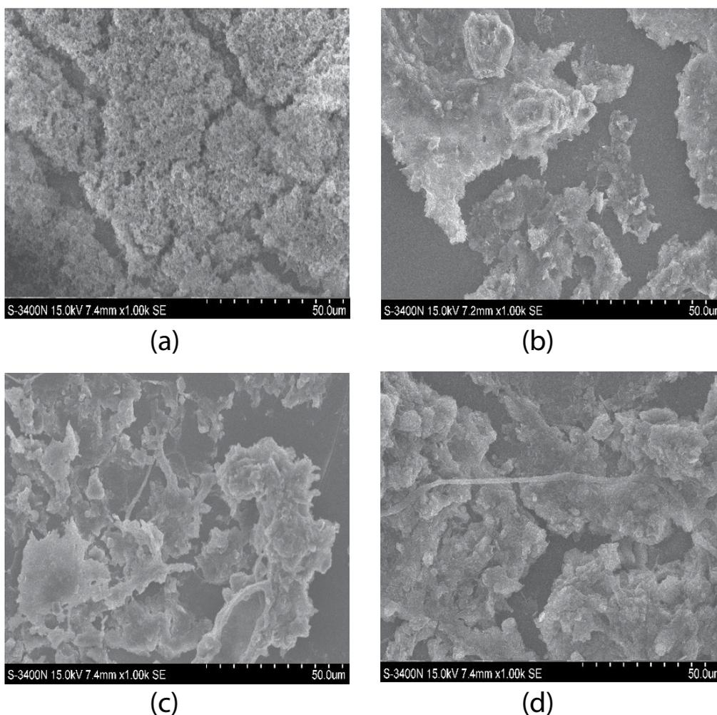
Fig. 2. Scanning electron microscope photos of sludge floc ( $\times 1,000$ ). (a) Control, (b) added polysilicate ferric, (c) added aluminum sulfate and (d) added ferric chloride.
