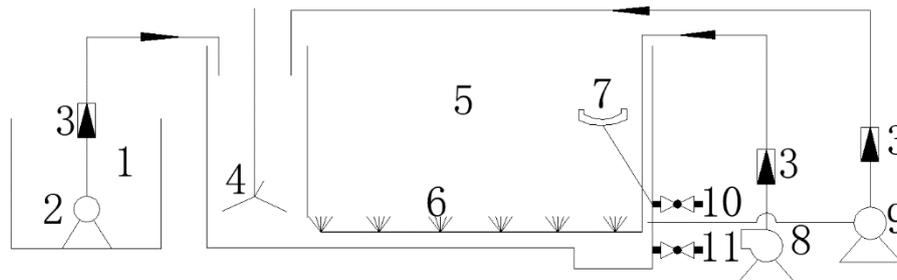
Fig. 1. Flowchart of CASS process. 1, Regulation pool; 2, inlet pump; 3, flow meter; 4, blender; 5, CASS reactor; 6, aeration head; 7, decanter; 8, aeration pump; 9, return pump; 10, drain pipe; 11, mud tubes.
