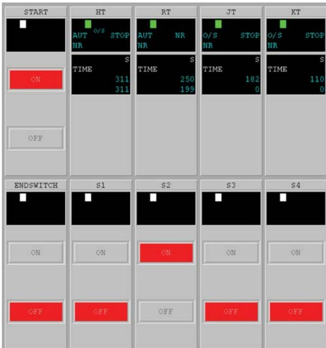
Fig. 9. Faceplate showing timers and internal switches activation.
