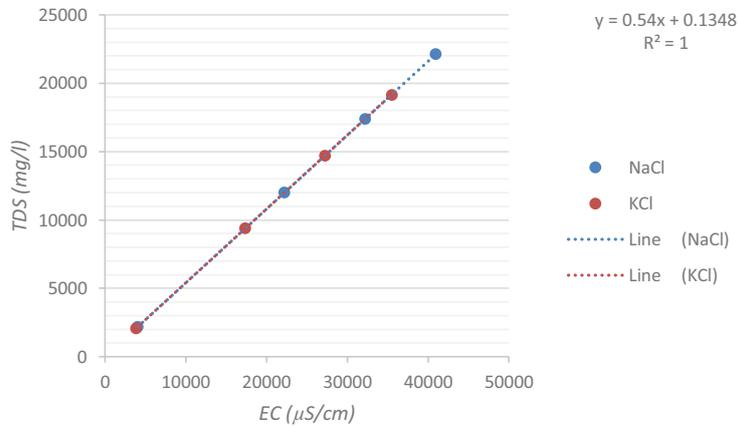
Fig. 9. Total dissolved salts (TDS) content vs. electrical conductivity.
