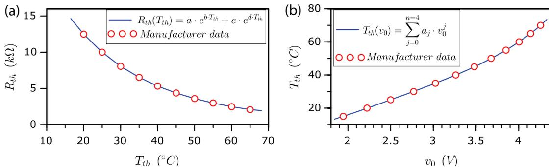
Fig. 10. Relationship between resistance and temperature (a) and between temperature and voltage (b) and resistance, compared with the data provided by the manufacturer.
