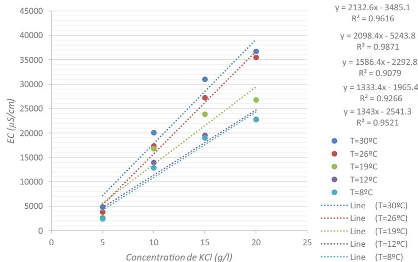
Fig. 7. Electrical conductivity vs. different salinity concentrations of KCl at different temperatures.
