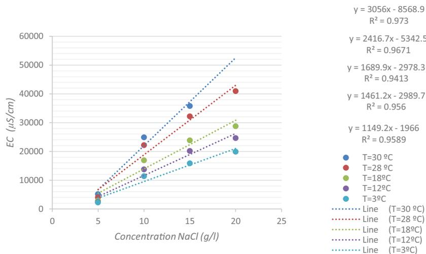
Fig. 6. Electrical conductivity vs. different salinity concentrations of NaCl at different temperatures.
