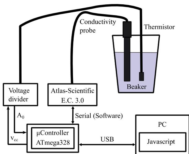
Fig. 1. Low-cost system to measure electrical conductivity (EC) and temperature (T).
