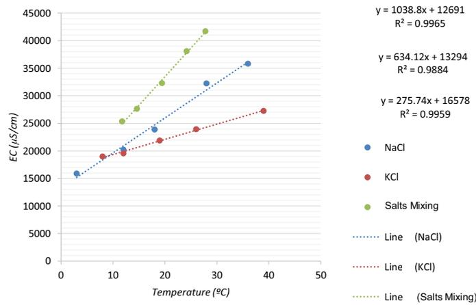
Fig. 8. Effect of temperature on conductivity [NaCl] = 15 g/L; [KCl] = 15 g/L.
