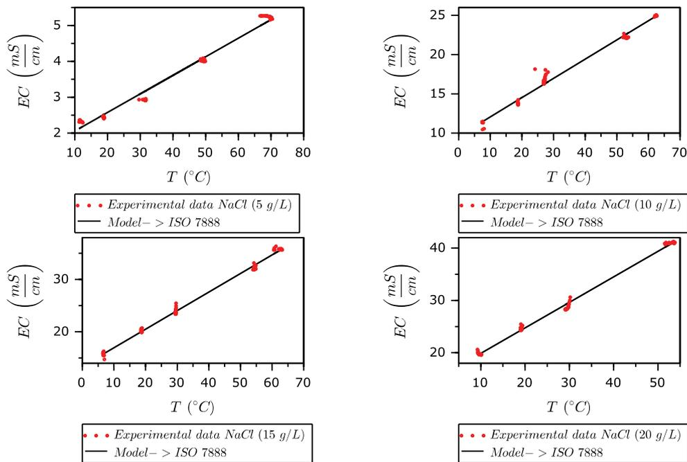
Fig. 12. Experimental results of EC vs. T at different NaCl solution concentrations and theoretical values calculated based on the ISO 7888-1985 model.
