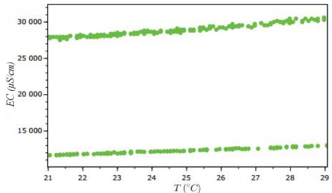
Fig. 5. Electrical conductivity vs. temperature comparing two solutions of KCl.
