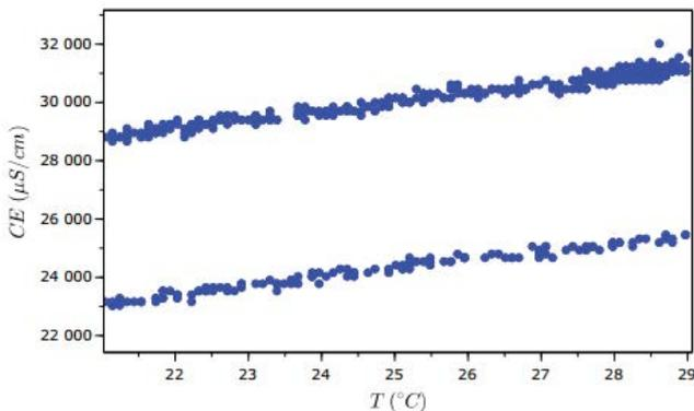
Fig. 4. Electrical conductivity vs. temperature comparing two solutions of NaCl.
