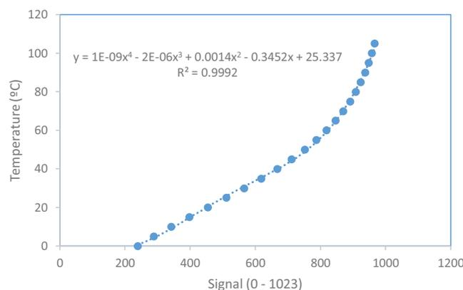
Fig. 2. Temperature curve for the thermistor used.
