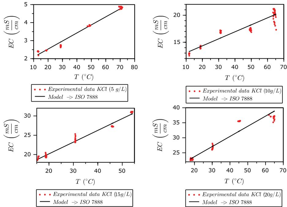
Fig. 11. Experimental results of EC vs. T at different KCl solution concentrations and theoretical values calculated based on the ISO 7888-1985 model.
