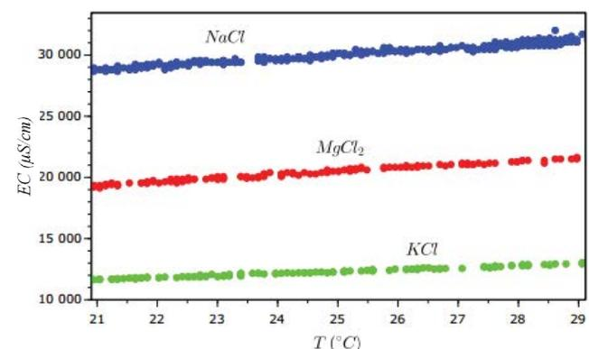
Fig. 3. Electrical conductivity vs. temperature comparing three different salts.
