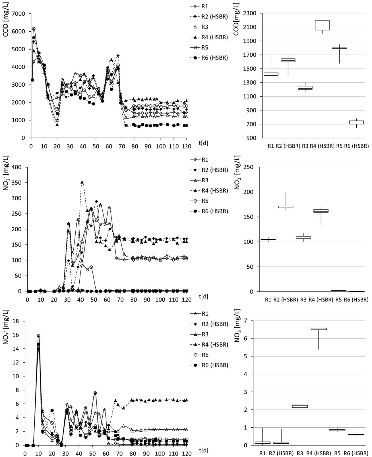
Fig. 3. The dynamics of organic substances expressed as COD, nitrite and nitrate concentration in the outflows from reactors, in subsequent days (d) of the experiment. Box-plot graphs show quartiles (box) and range (whiskers).
