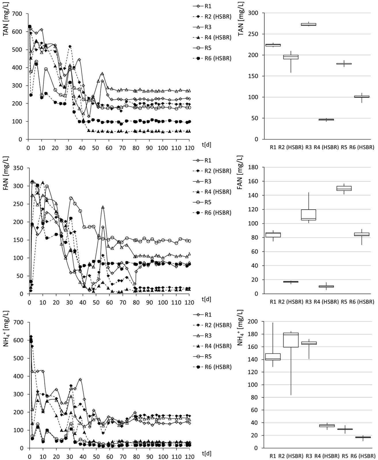
Fig. 4. The dynamics of total ammonia nitrogen (TAN), free ammonium nitrogen (FAN) and ammonia nitrogen concentration in the outflows from reactors, in subsequent days (d) of the experiment. Box-plot graphs show quartiles (box) and range (whiskers).
