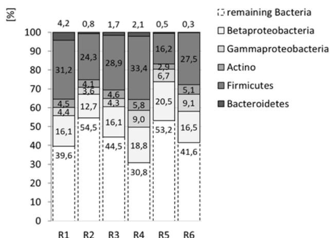
Fig. 9. Proportions of selected phyla in subsequent reactors on the basis of quantitative measurement of total bacteria count.
