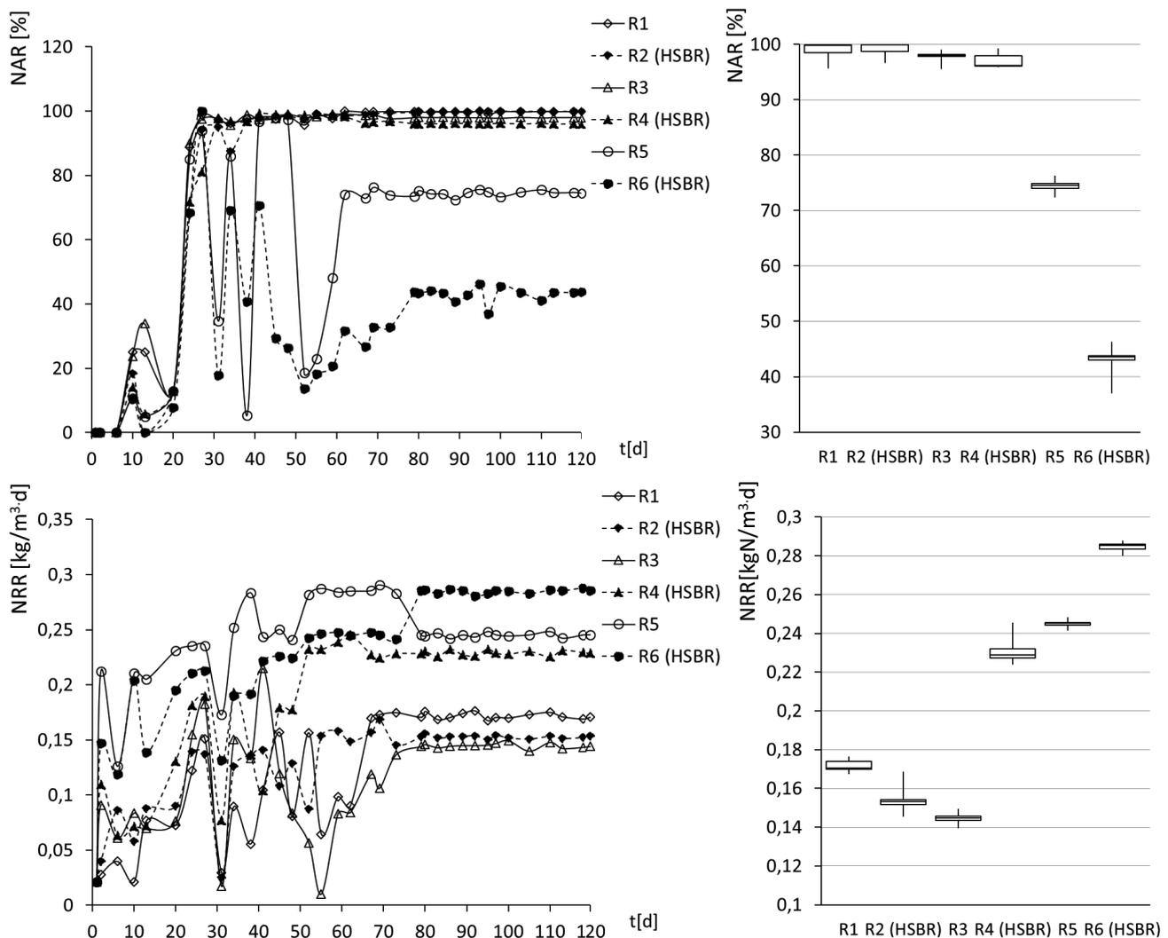
Fig. 5. The dynamics of nitrite accumulation ratio (NAR) and nitrogen removal rate (NRR) in reactors, in subsequent days (d) of the experiment. Box-plot graphs show quartiles (box) and range (whiskers).
