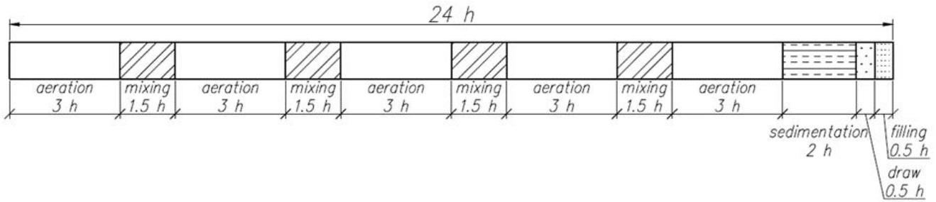
Fig. 2. The operational cycle of hybrid and conventional SBRs.
