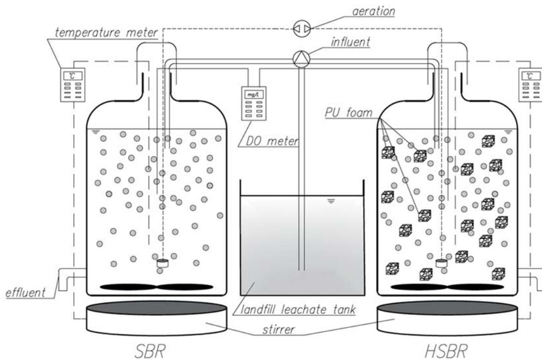
Fig. 1. Schematic diagram of the experimental layout used in this study to compare the efficiency of landfill leachate treatment in different temperatures.
