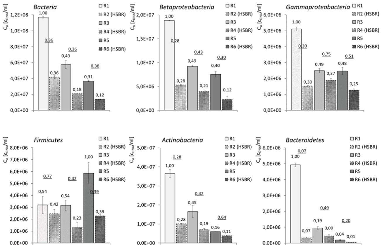
Fig. 8. A number of 16S rRNA copies specific to the chosen phyla. Whiskers indicate the measurement error, numbers above the bars relative proportion of the number of genomes to the highest recorded value, and the numbers underlined proportion between SBR and HSBR operating at the same temperature.
