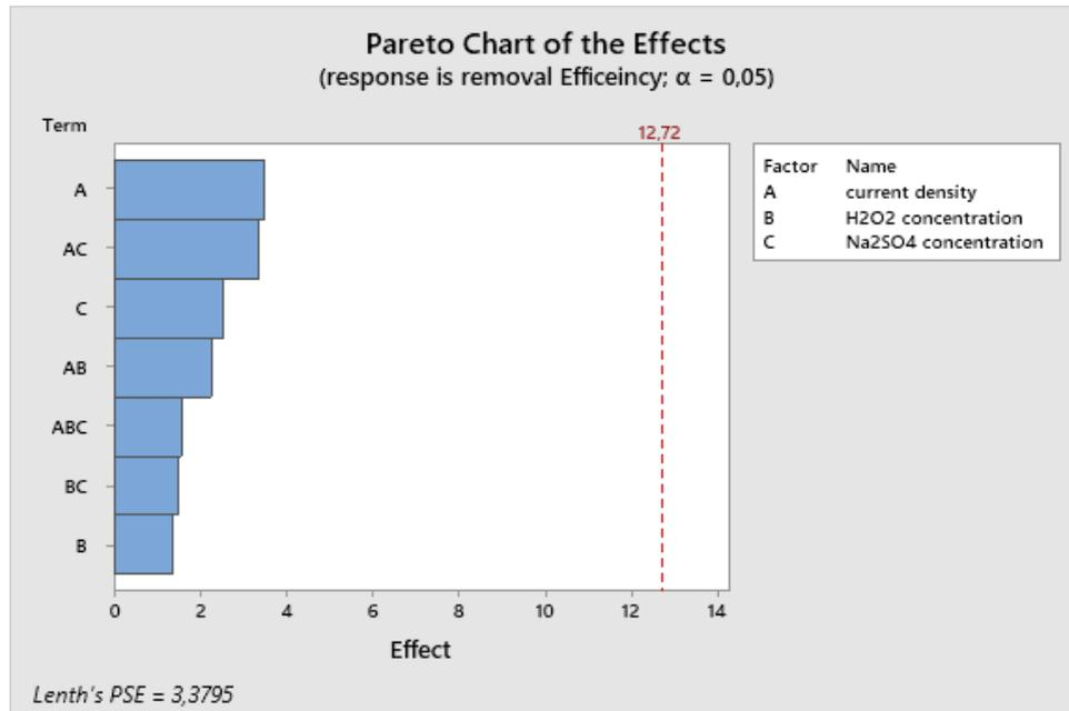
Fig. 3. Pareto chart of EF process parameter on COD removal efficiency.
