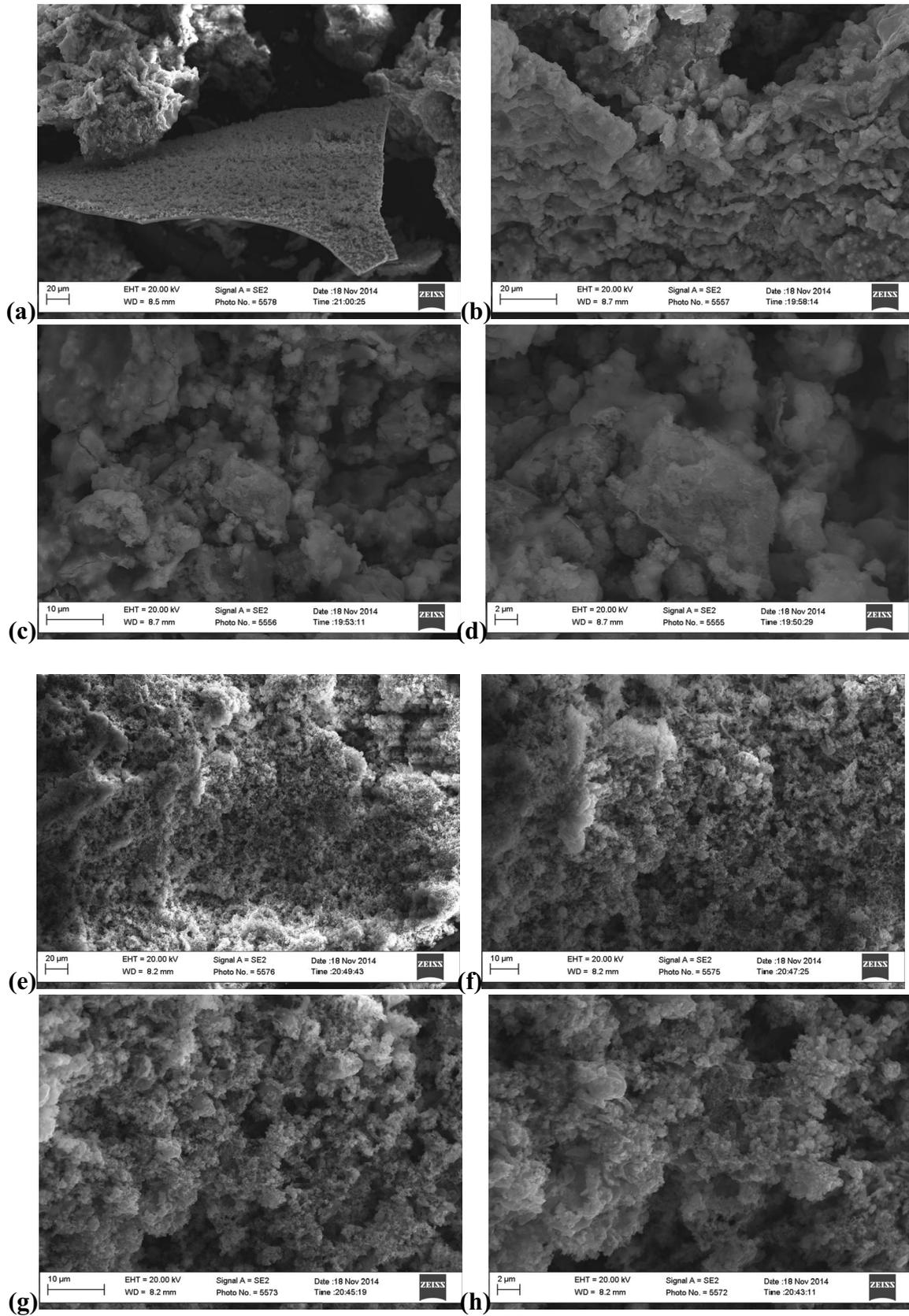
Fig. 7. SEM images of sludge samples (a) 1,000x; (b) 2,500x; (c) 5,000x; (d) 10,000x magnification of untreated wastewater sludge, (e) 1,000x; (f) 2,500x; (g) 5,000x; (h) 10,000x magnification of  $\bullet\text{OH}$ -based EF treated wastewater sludge.
