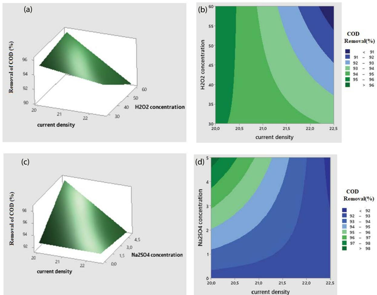
Fig. 4. The surface plot (a) and the contour plot (b) of the COD removal response as a function of the current density vs. H<sub>2</sub>O<sub>2</sub> concentration, and the surface plot (c) and the contour plot (d) of the COD removal response as a function of and current density vs. Na<sub>2</sub>SO<sub>4</sub> concentration.
