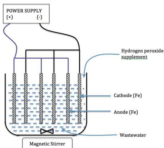
Fig. 1. Experimental setup used in the electrochemical-Fenton (EF) treatment.
