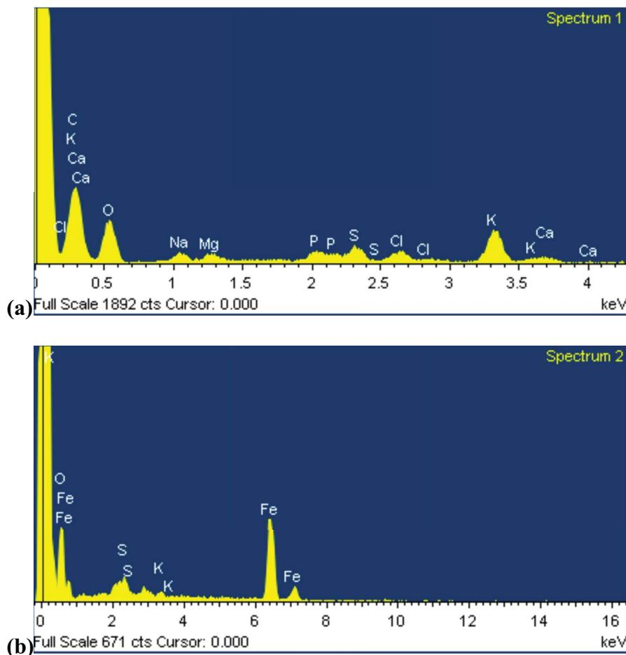
Fig. 6. EDX spectrum for untreated wastewater sludge (a) and  $\cdot\text{OH}$ -based EF treated wastewater sludge (b).
