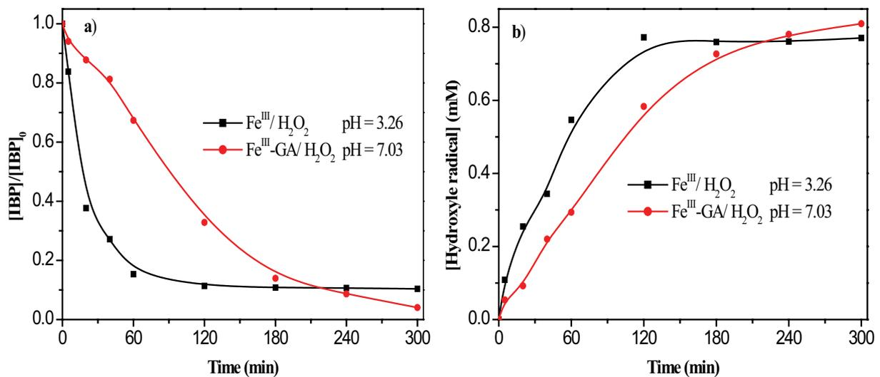
Fig. 6. (a) Comparative study between classical Fenton-like and modified Fenton-like for the degradation of IBP (0.05 mM), H<sub>2</sub>O<sub>2</sub> (5 mM), T = 25°C and (b) hydroxyl radicals formation.
