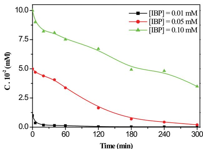
Fig. 10. Effect of the initial concentration of the IBP on its degradation by the  $\text{Fe}^{\text{III}}$ -GA/ $\text{H}_2\text{O}_2$  system (0.1 and 5 mM),  $\text{pH} = 7.0 \pm 0.1$ ,  $T = 25^\circ\text{C}$ .
