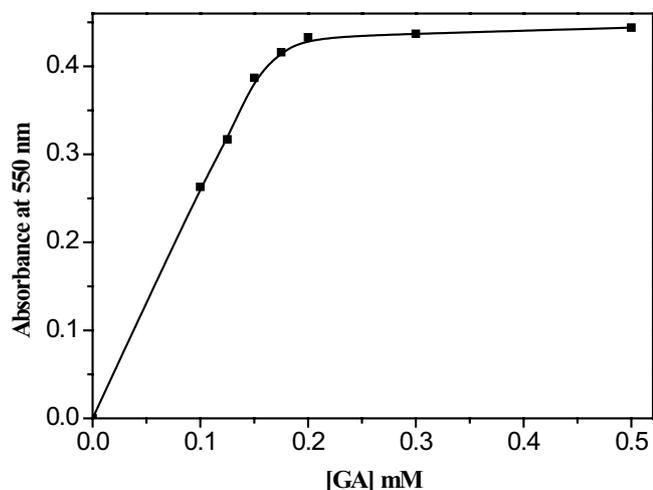
Fig. 3. Evolution of the absorbance at 550 nm as a function of the GA concentration.
