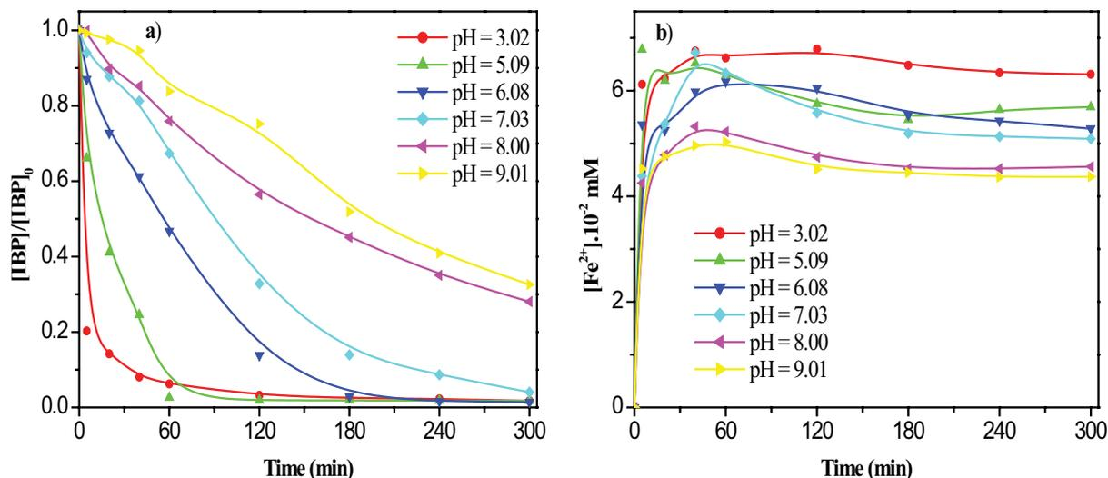
Fig. 11. (a) Effect of pH on the degradation of IBP (0.05 mM) by the  $\text{Fe}^{\text{III}}$ -GA/ $\text{H}_2\text{O}_2$  system (0.1 and 5 mM),  $\text{pH} = 7.0 \pm 0.1$ ,  $T = 25^\circ\text{C}$  and (b)  $\text{Fe}^{\text{II}}$  formation.
