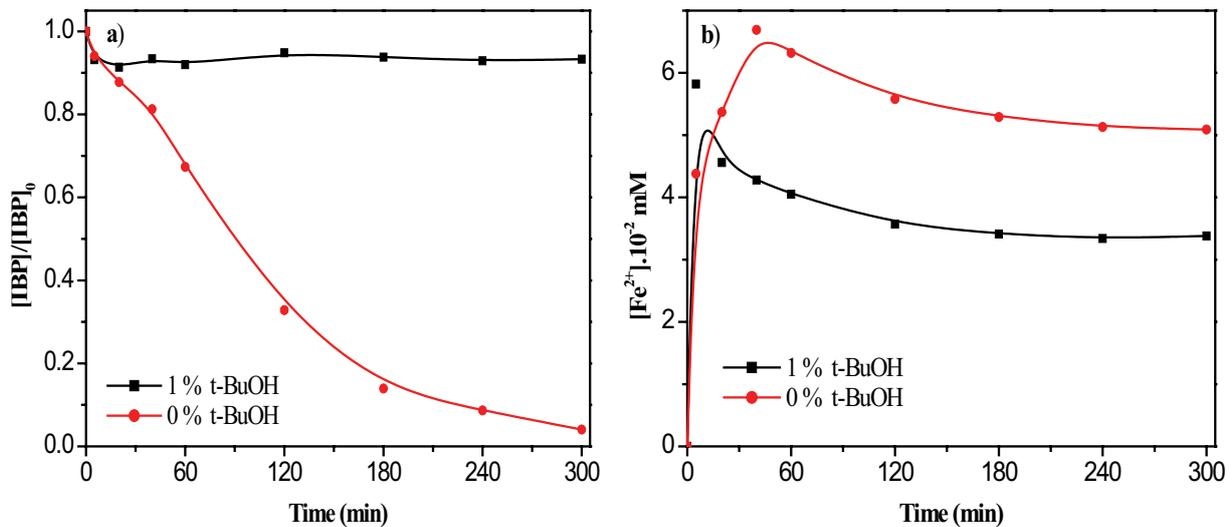
Fig. 13. (a) Effect of t-BuOH on the degradation of IBP (0.05 mM) by the  $\text{Fe}^{\text{III}}$ -GA/ $\text{H}_2\text{O}_2$  system (0.1 and 5 mM),  $\text{pH} = 7.0 \pm 0.1$ ,  $T = 25^\circ\text{C}$  and (b)  $\text{Fe}^{\text{II}}$  formation.
