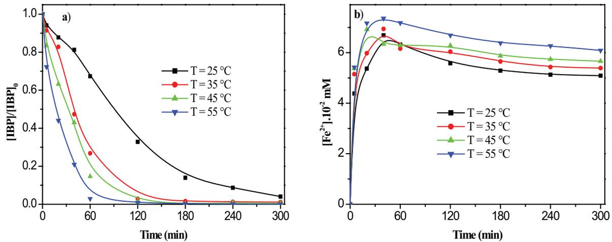
Fig. 12. (a) Effect of temperature on the degradation of IBP (0.05 mM) by the  $\text{Fe}^{\text{III}}$ -GA/ $\text{H}_2\text{O}_2$  system (0.1 and 5 mM),  $\text{pH} = 7.0 \pm 0.1$  and (b)  $\text{Fe}^{\text{II}}$  formation.
