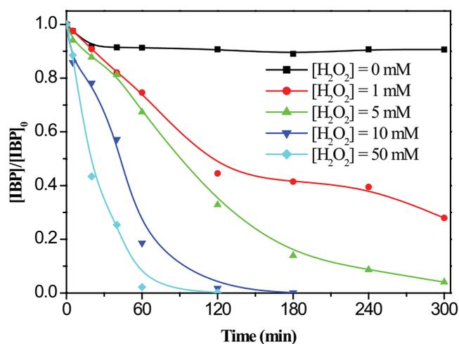
Fig. 7. Effect of  $H_2O_2$  concentrations on the degradation of IBP (0.05 mM) by the  $Fe^{III}$ -GA/ $H_2O_2$  system (0.1 mM), pH =  $7.0 \pm 0.1$ ,  $T = 25^\circ C$ .
