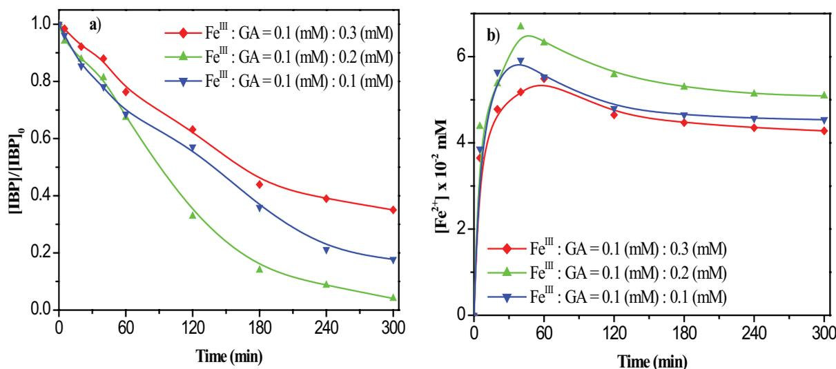
Fig. 9. (a) Effect of  $\text{Fe}^{\text{III}}$ :GA molar ratio on the degradation of IBP (0.05 mM) by the  $\text{Fe}^{\text{III}}$ -GA/ $\text{H}_2\text{O}_2$  system,  $[\text{H}_2\text{O}_2] = 5$  mM,  $\text{pH} = 7.0 \pm 0.1$ ,  $T = 25^\circ\text{C}$  and (b)  $\text{Fe}^{\text{II}}$  formation.
