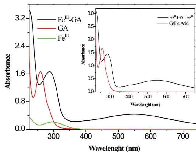
Fig. 1. UV-visible absorption spectrum: GA (0.2 mM),  $\text{Fe}^{\text{III}}$  (0.1 mM) and the  $\text{Fe}^{\text{III}}\text{-GA}$  complex (0.1 mM), pH = 7.0  $\pm$  0.1. Insertion: UV-visible absorption spectrum of the difference [ $\text{Fe}^{\text{III}}\text{-GA} - \text{Fe}^{\text{III}}$ ], pH = 7.0  $\pm$  0.1.
