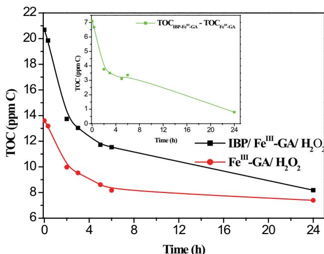
Fig. 14. Evolutions of TOC of IBP (0.05 mM) in Fe<sup>III</sup>-GA/H<sub>2</sub>O<sub>2</sub> system (0.1 mM, 5 mM), pH = 7.0 ± 0.1, T = 25°C.
