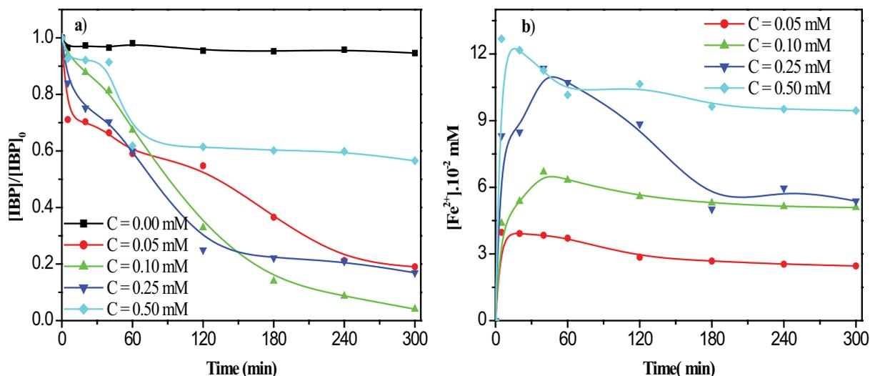
Fig. 8. (a) Effect of  $Fe^{III}$ -GA complex concentration on the degradation of IBP (0.05 mM) by the  $Fe^{III}$ -GA/ $H_2O_2$  system (0.1 and 5 mM), pH =  $7.0 \pm 0.1$ ,  $T = 25^\circ C$  and (b)  $Fe^{II}$  formation.
