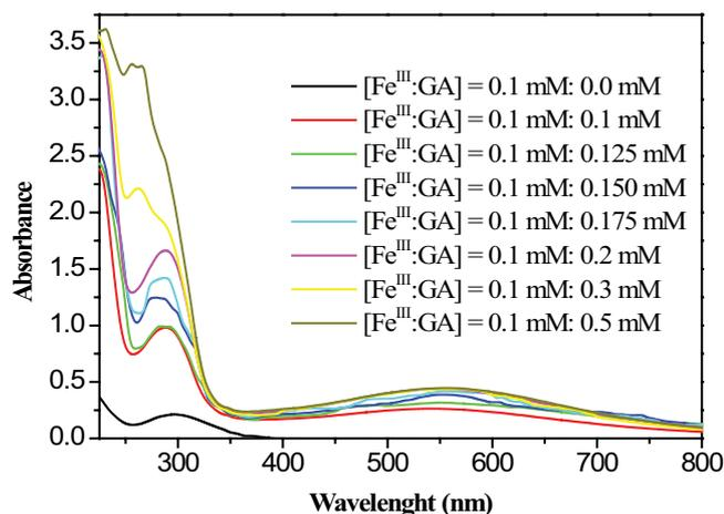
Fig. 2. UV-visible spectra of GA and Fe<sup>III</sup> mixtures in aqueous solution at pH = 7.0 ± 0.1.
