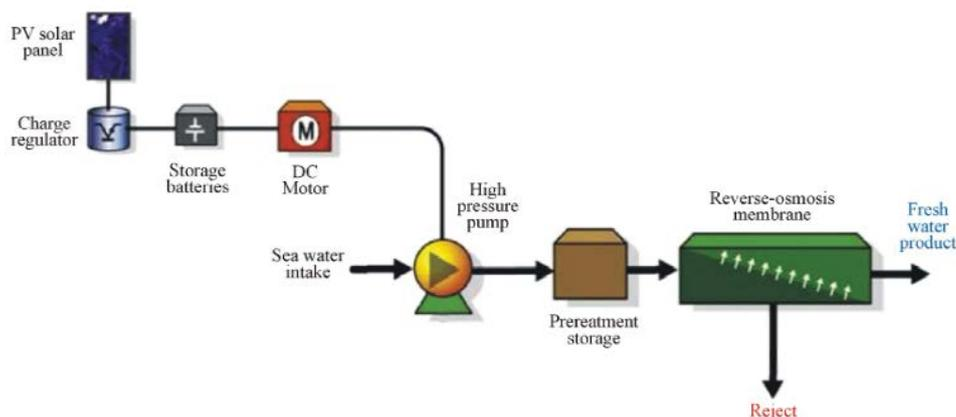
Fig. 3. Schematic diagram of PV-RO system [18].
