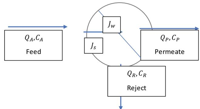
Fig. 1. Simplification of the desalination process.
