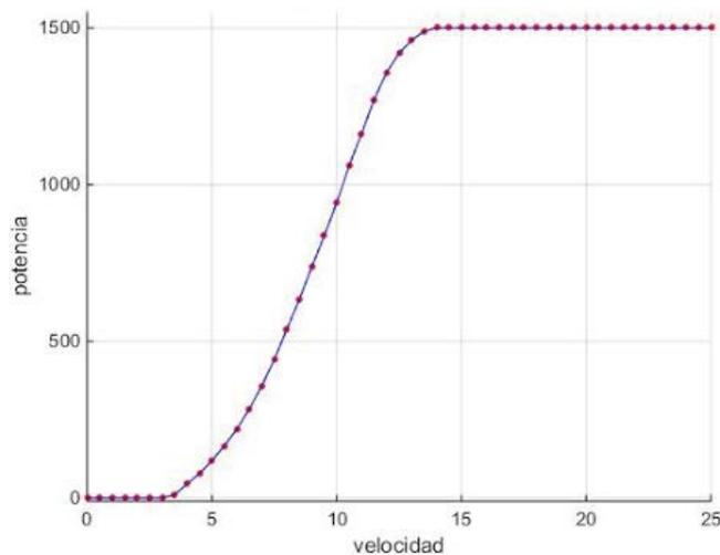
Fig. 2. Energy produced by a wind turbine.
